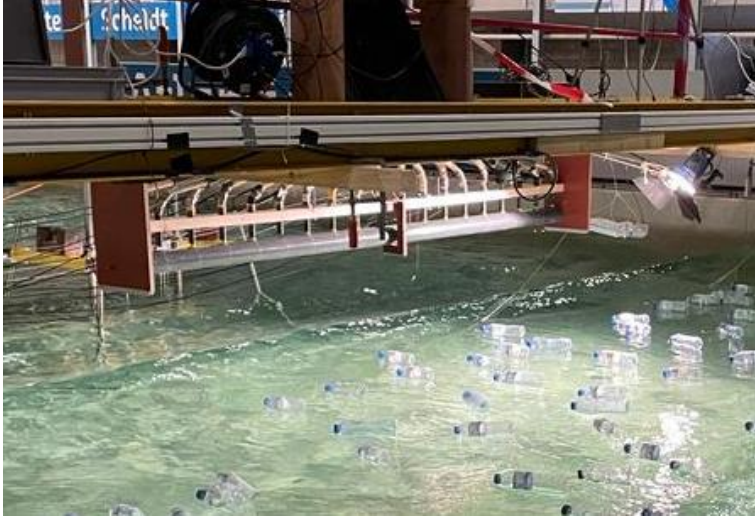
Figure 2.4 The particle dispenser mounted to the bridge at the center of the basin 16.7 m from the wavemaker.
