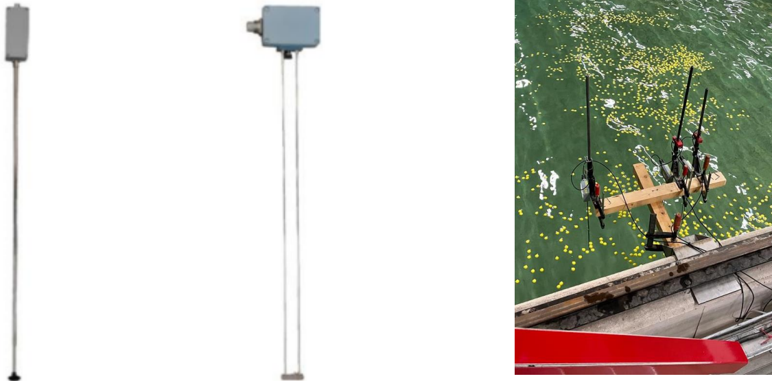
Figure 2.3 Measurement equipment used in the physical model (left) the electromagnetic velocity sensor, (center) the wave gauge, and (right) installed wave gauges at the side of the basin.
