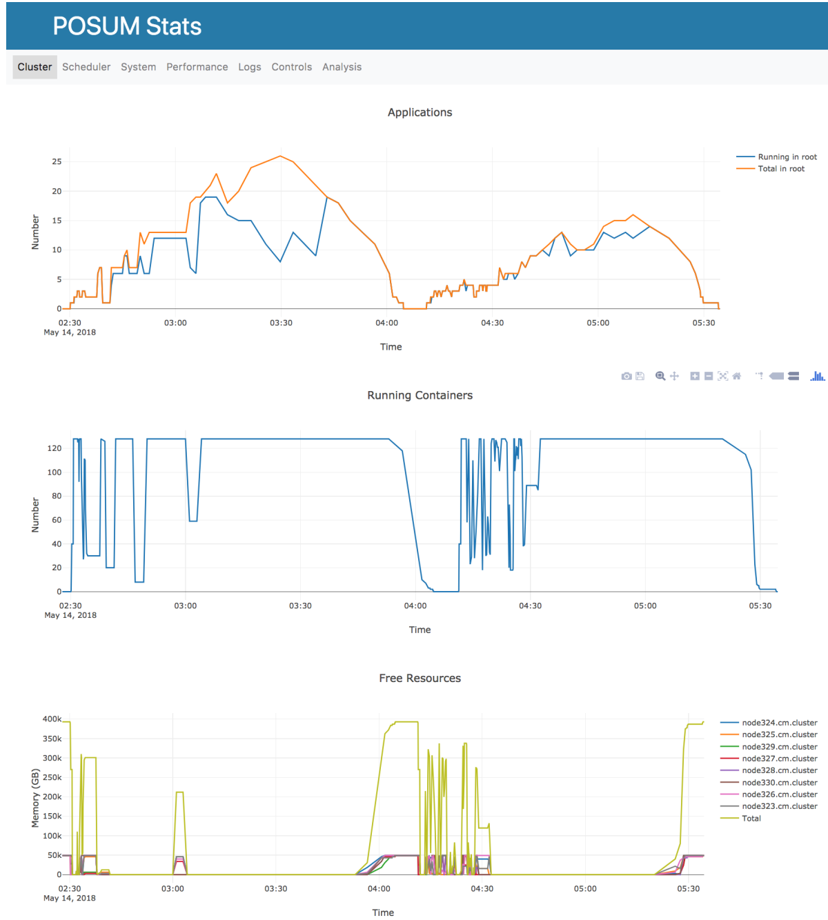
Figure B.1: The cluster tab displays the number of running applications and containers, and the available resources.
