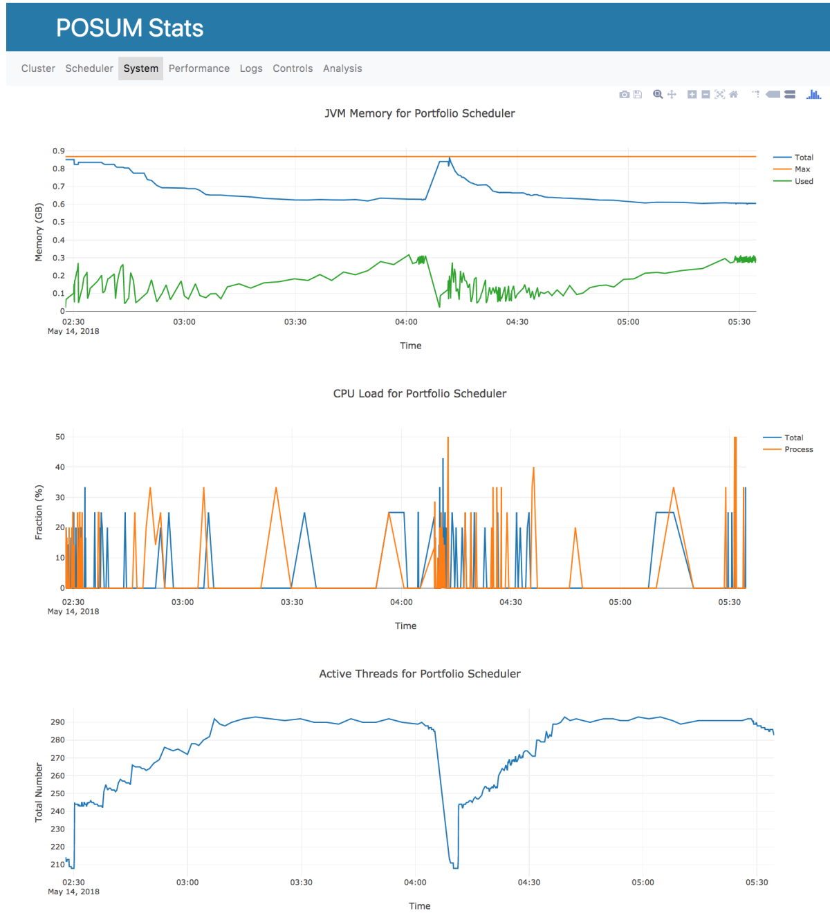
Figure B.3: The system tab displays the resource usage of each process in the environment.
