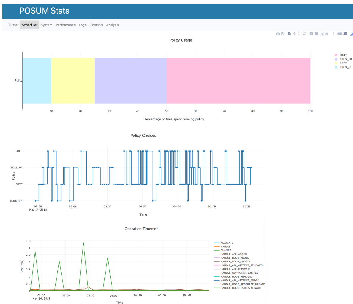
Figure B.2: The scheduler tab displays the information about policy usage and the time cost of scheduler operations.
