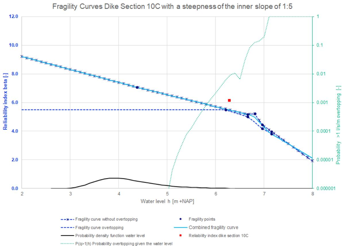
Figure 115: Fragility curves dike section 10C with a steepness of the inner slope of 1:5
