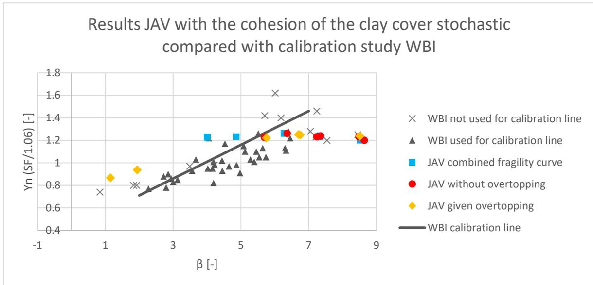
Figure 48: The results of the calculations of JAV with the cohesion of the clay cover stochastic compared with the calibration study of WBI. The vertical position of the results of JAV from the combined fragility curves (blue squares) are determined based on the semi-probabilistic results without overtopping
