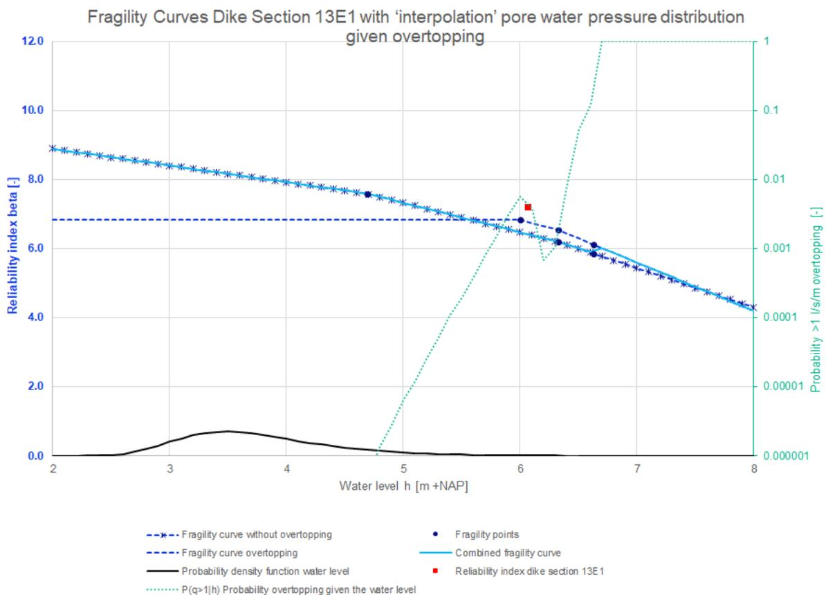
Figure 76: Fragility curves dike section 13E1 with 'interpolation' pore water pressure distribution given overtopping
