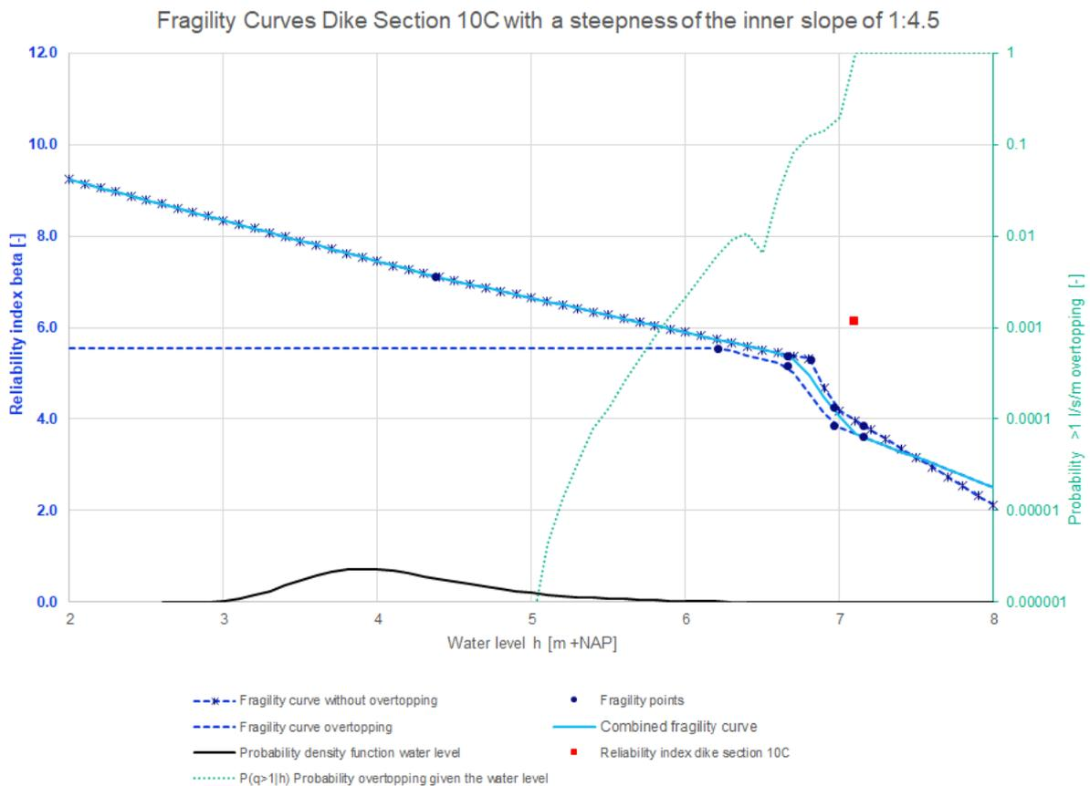
Figure 107: Fragility curves dike section 10C with a steepness of the inner slope of 1:4.5
