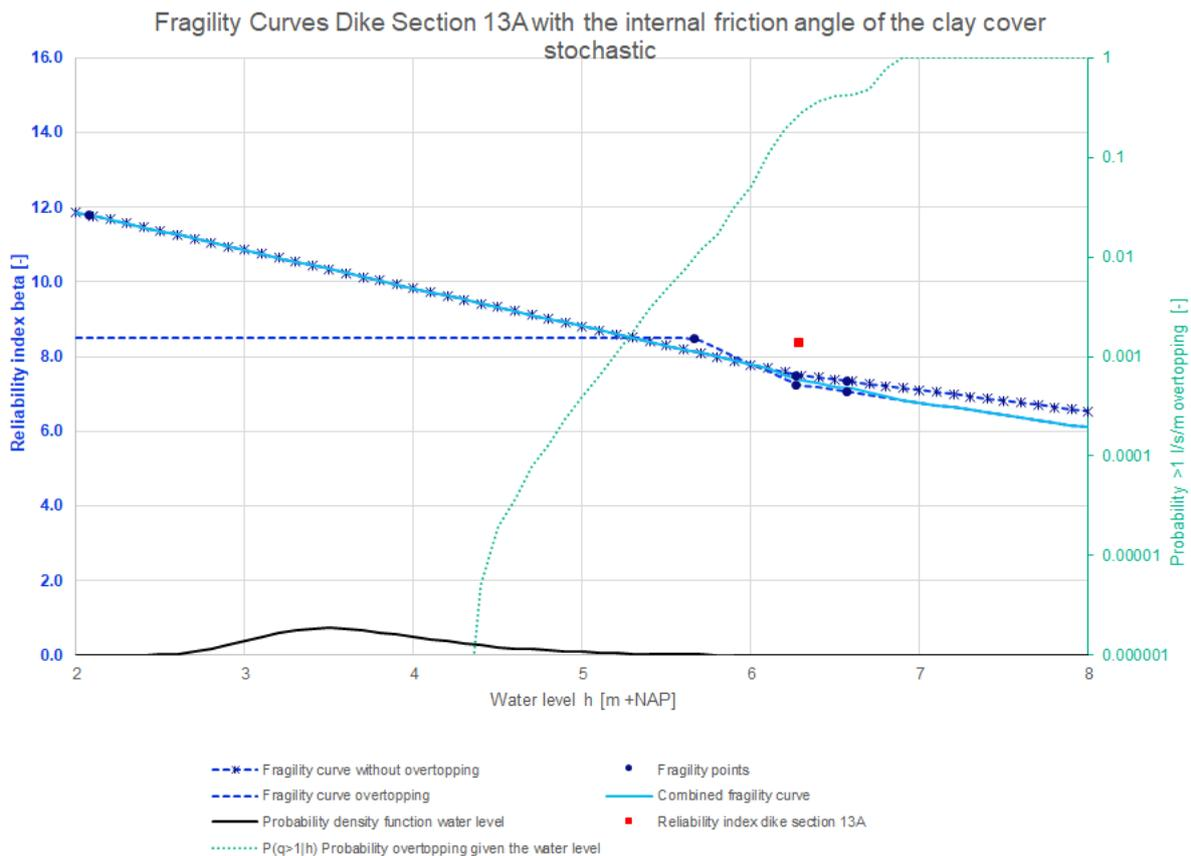
Figure 53: Fragility curves dike section 13A with the internal friction angle of the clay cover stochastic
