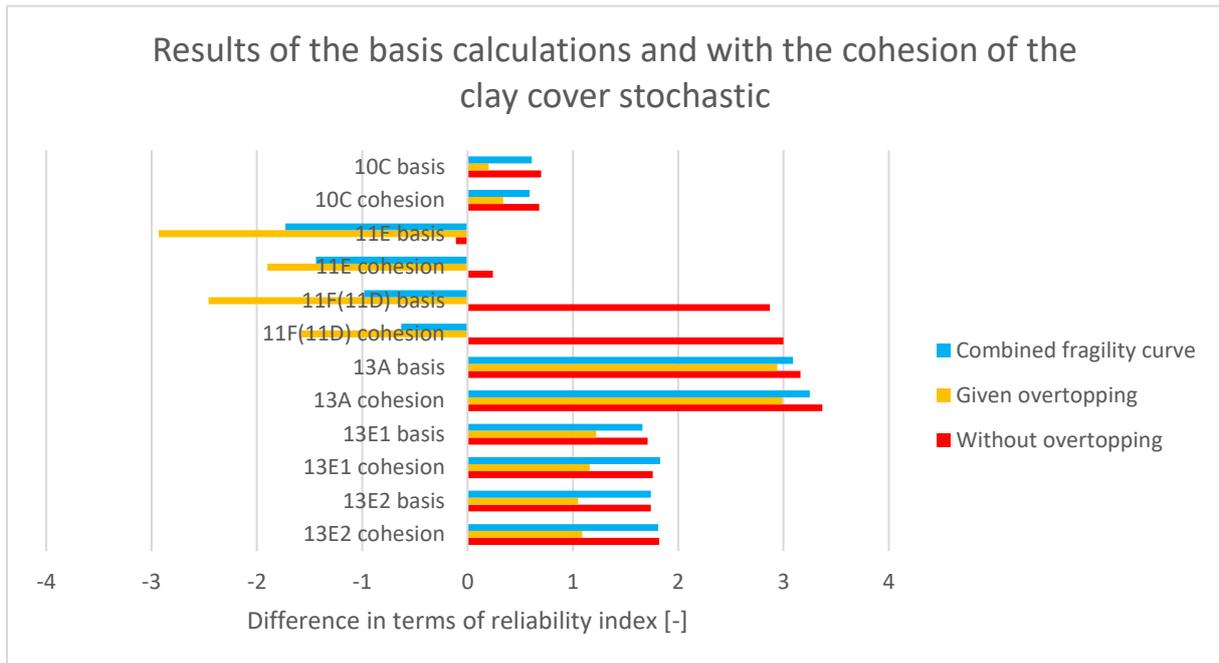
Figure 22: The results of the basis calculations of JAV and with the cohesion stochastic compared with the calibration study of WBI. The semi-probabilistic results without overtopping are used to determine the difference in terms of reliability index for the combined fragility curves
