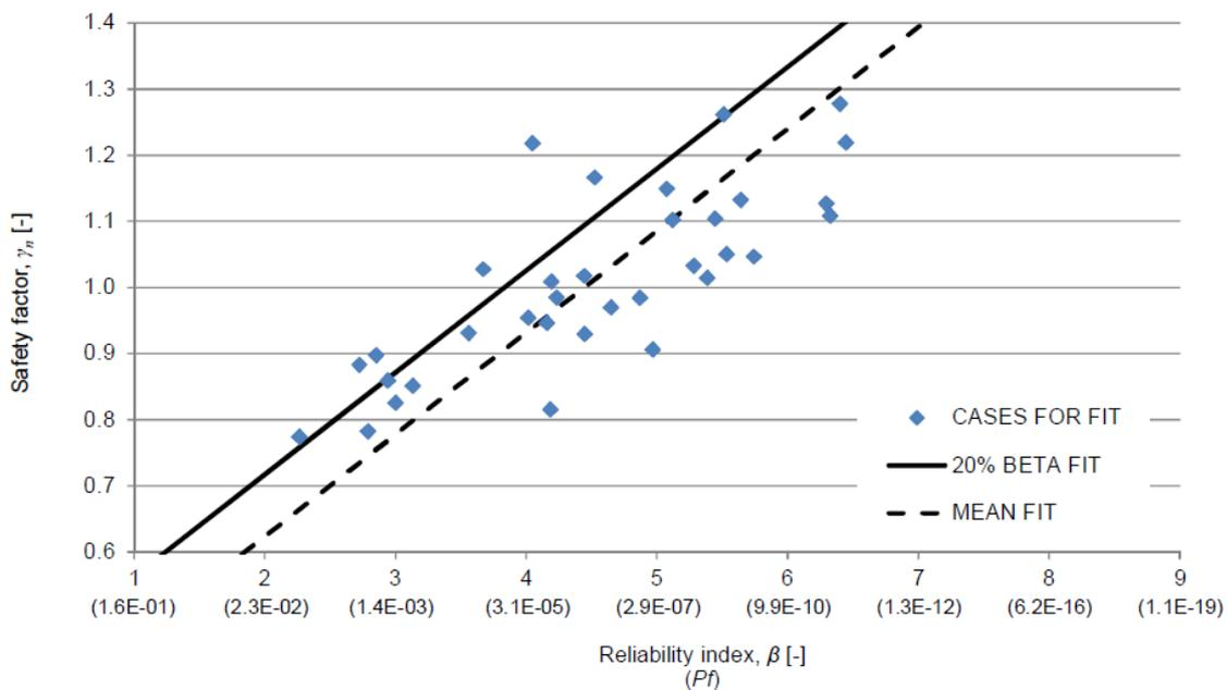
Figure 8: Calibration fit between the safety factor and the reliability index (Kanning, Teixeira, Van der Krogt, & Rippi, 2017)
