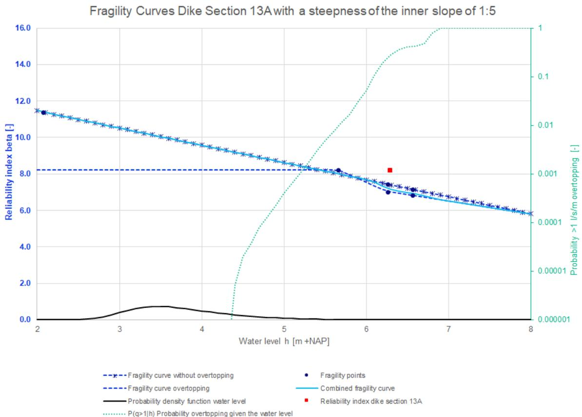
Figure 118: Fragility curves dike section 13A with a steepness of the inner slope of 1:5
