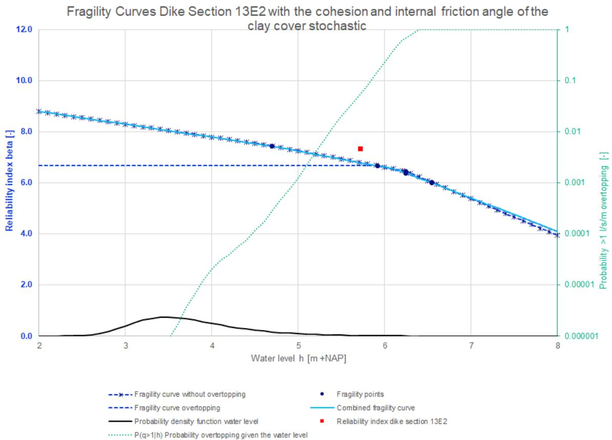
Figure 63: Fragility curves dike section 13E2 with the cohesion and internal friction angle of the clay cover stochastic
