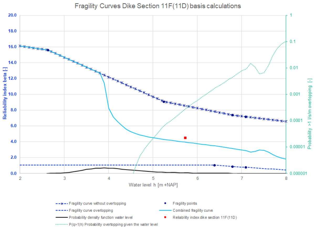
Figure 38: Fragility curves dike section 11F(11D) basis calculations
