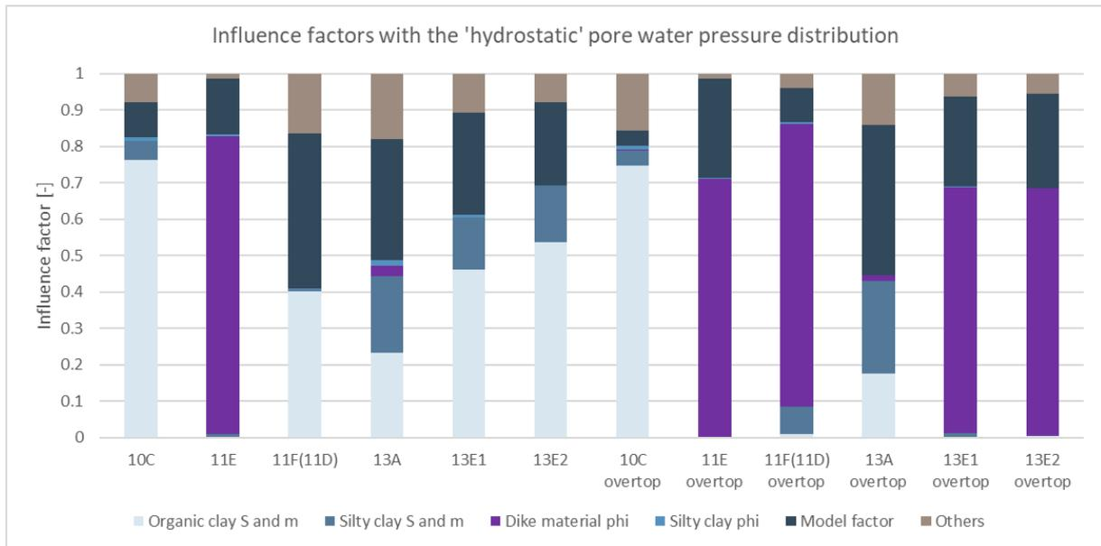
Figure 71: Influence factors with the 'hydrostatic' pore water pressure distribution at WBN without overtopping and at the 1 l/s/m overtopping water level with overtopping
