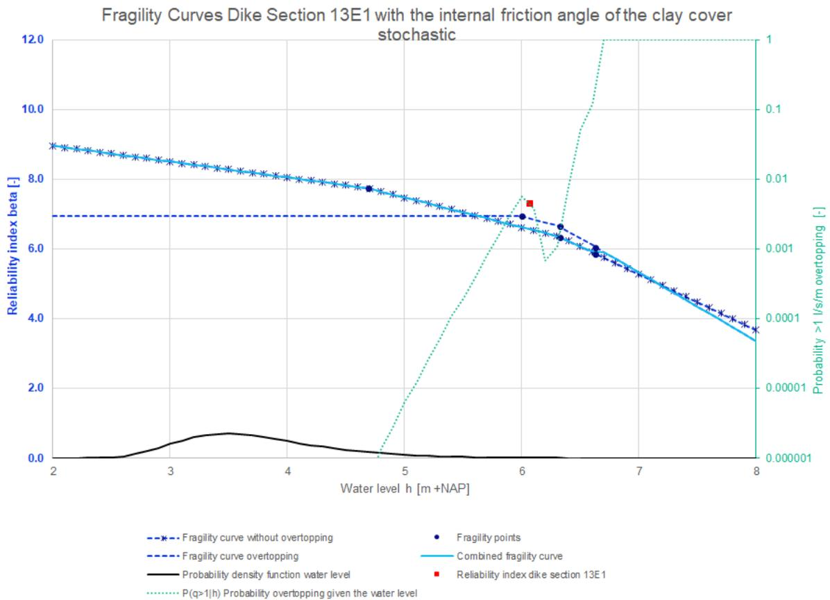
Figure 54: Fragility curves dike section 13E1 with the internal friction angle of the clay cover stochastic
