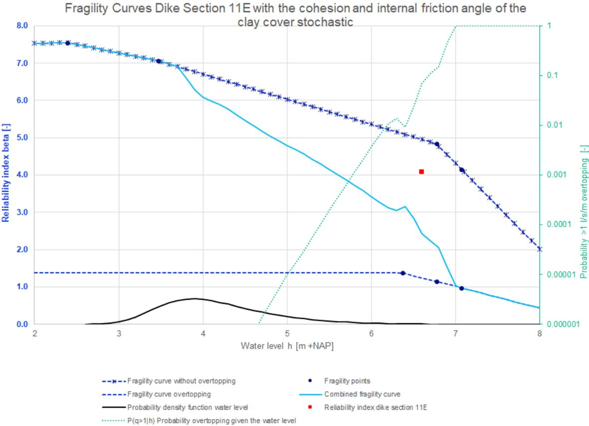
Figure 59: Fragility curves dike section 11E with the cohesion and internal friction angle of the clay cover stochastic
