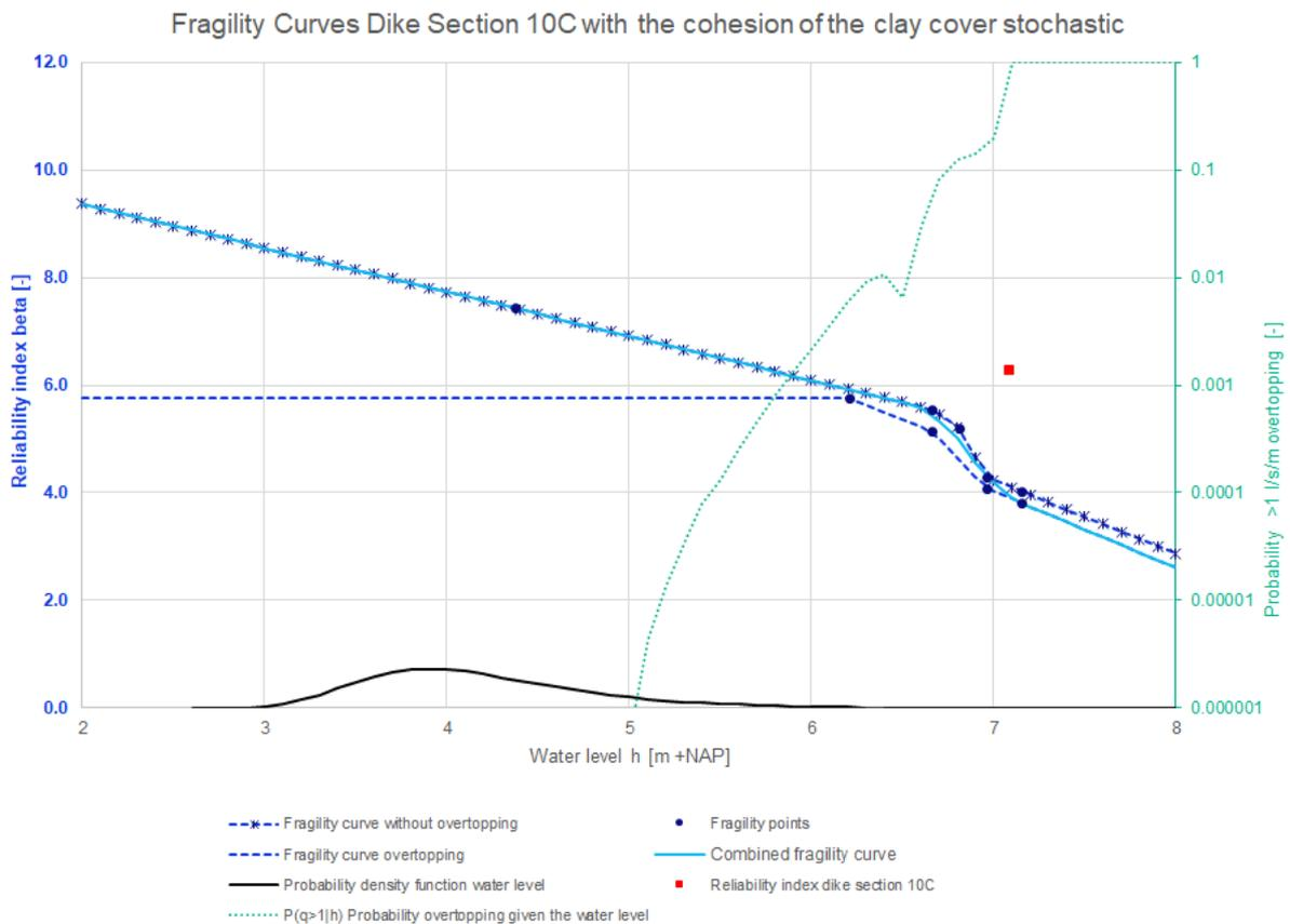
Figure 42: Fragility curves dike section 10C with the cohesion of the clay cover stochastic
