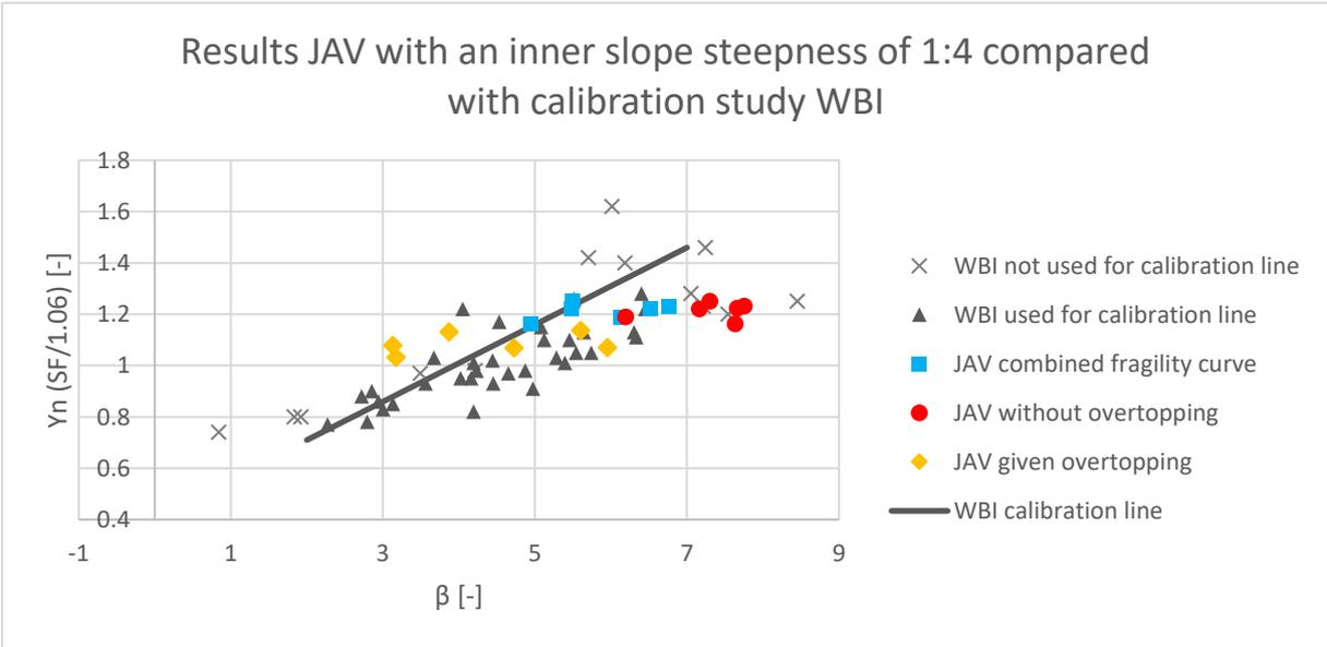
Figure 105: The results of the calculations of JAV with an inner slope steepness of 1:4 compared with the calibration study of WBI. The vertical position of the results of JAV from the combined fragility curves (blue squares) are determined based on the semi-probabilistic results without overtopping
