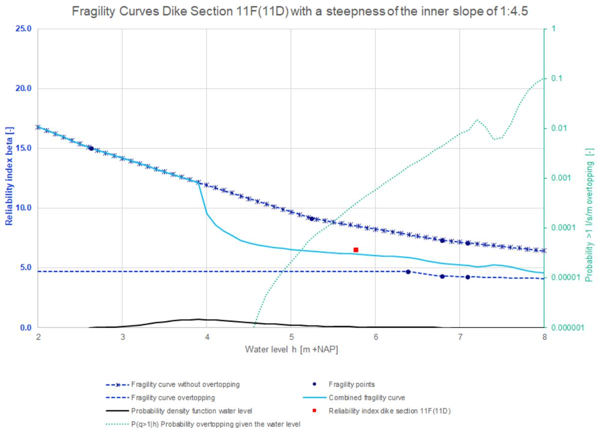
Figure 109: Fragility curves dike section 11F(11D) with a steepness of the inner slope of 1:4.5
