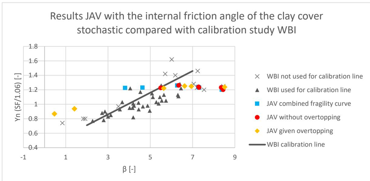
Figure 56: The results of the calculations of JAV with the internal friction angle of the clay cover stochastic compared with the calibration study of WBI. The vertical position of the results of JAV from the combined fragility curves (blue squares) are determined based on the semi-probabilistic results without overtopping
