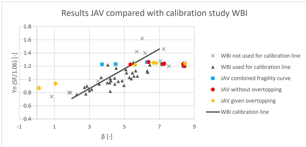
Figure 21: Results of the basis calculations of JAV compared with the calibration study of WBI. The vertical position of the results of JAV from the combined fragility curves (blue squares) are determined based on the semi-probabilistic results without overtopping
