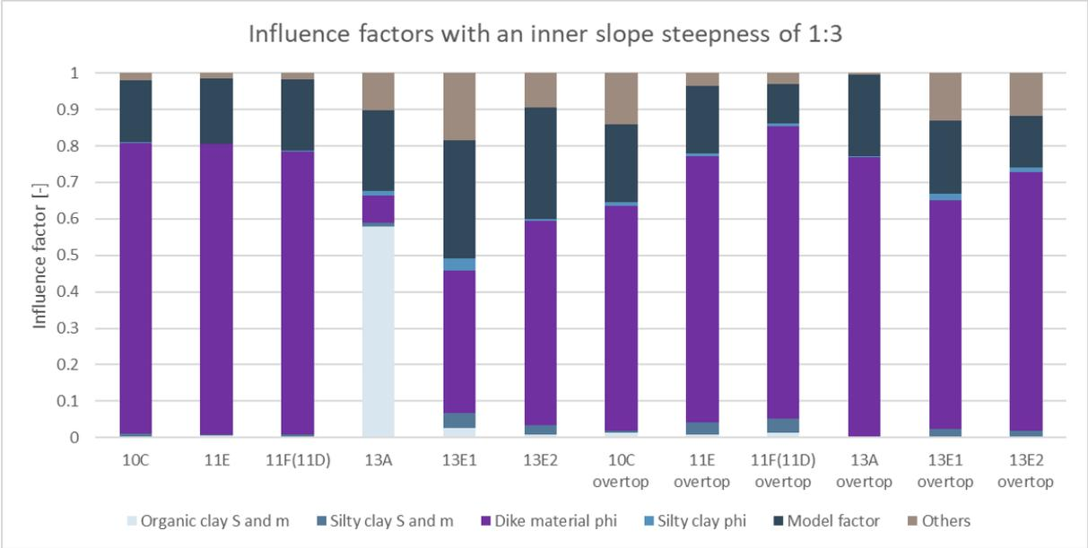
Figure 28: Influence factors with an inner slope steepness of 1:3 at WBN without overtopping and at the 1 l/s/m overtopping water level with overtopping
