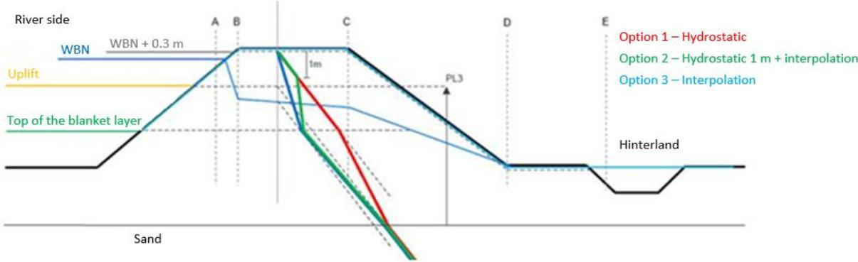
Figure 16: Schematization of the pore water pressure distribution with overtopping (Broere, 2022)
