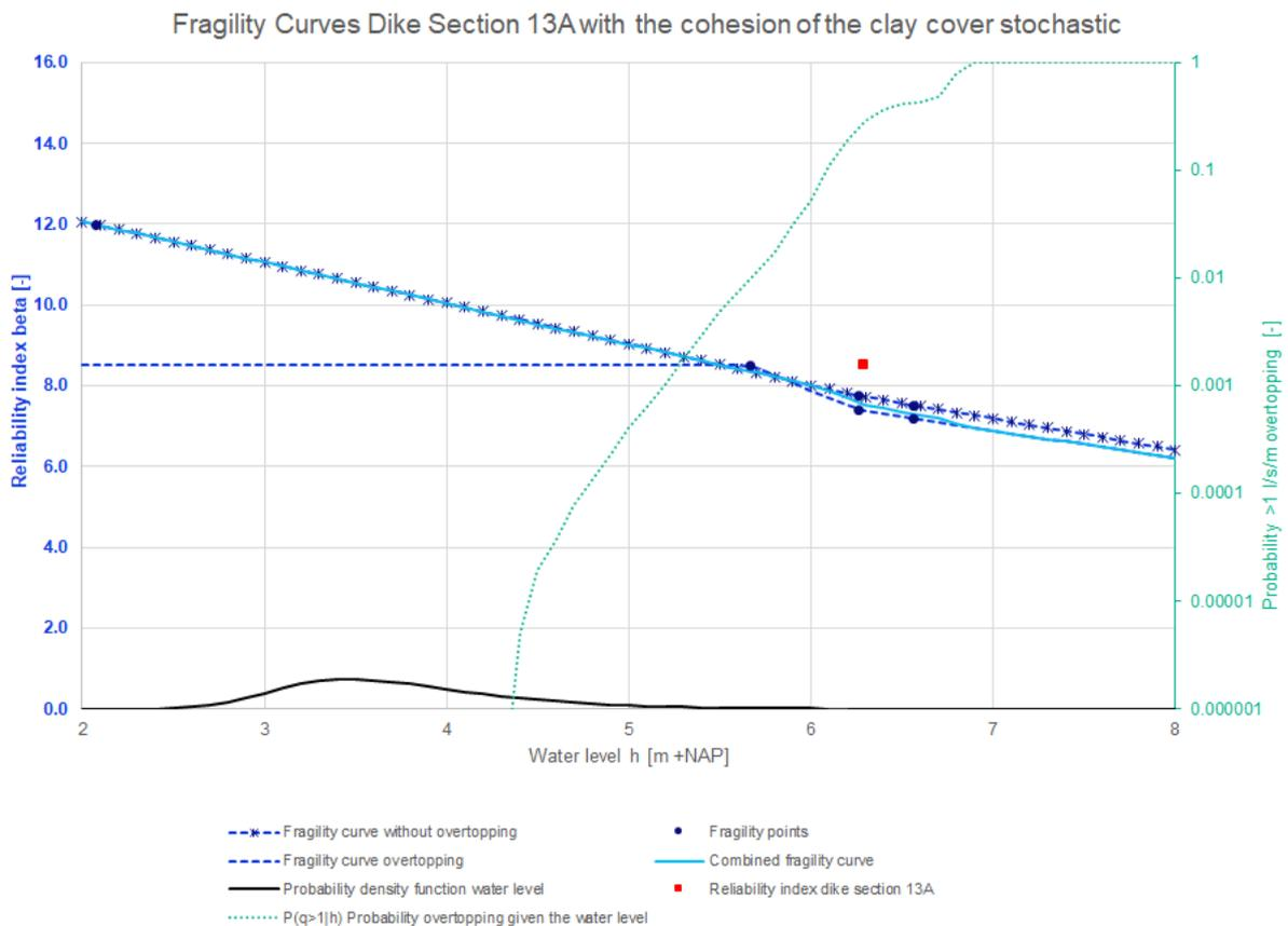
Figure 45: Fragility curves dike section 13A with the cohesion of the clay cover stochastic
