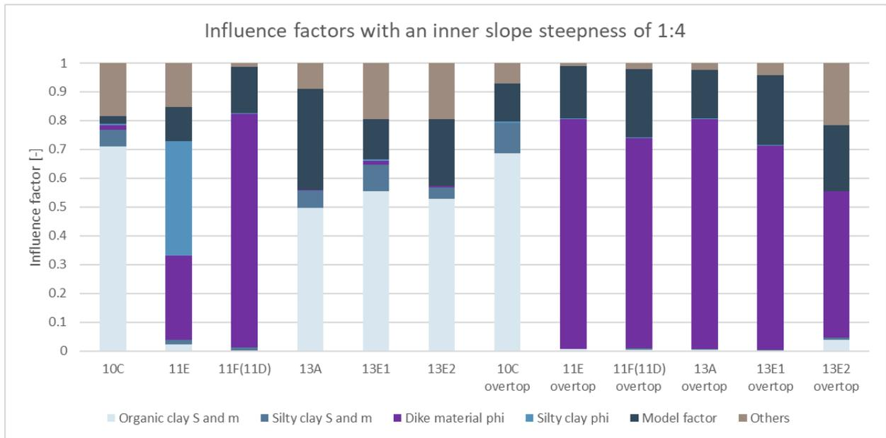
Figure 106: Influence factors with an inner slope steepness of 1:4 at WBN without overtopping and at the 1 l/s/m overtopping water level with overtopping
