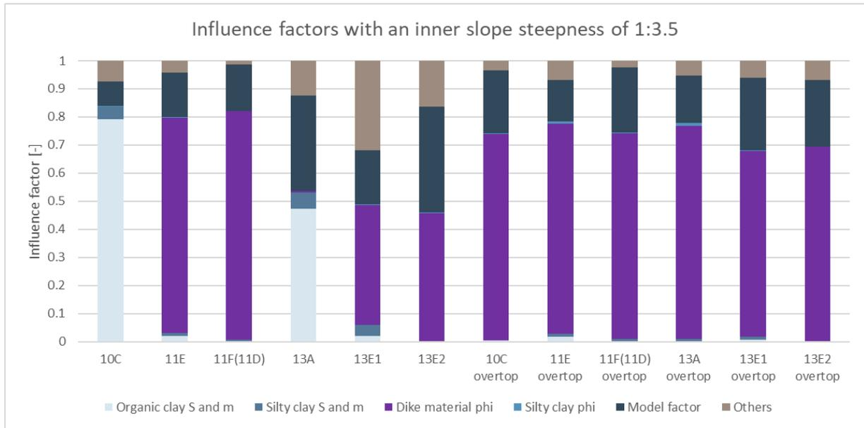
Figure 98: Influence factors with an inner slope steepness of 1:3.5 at WBN without overtopping and at the 1 l/s/m overtopping water level with overtopping
