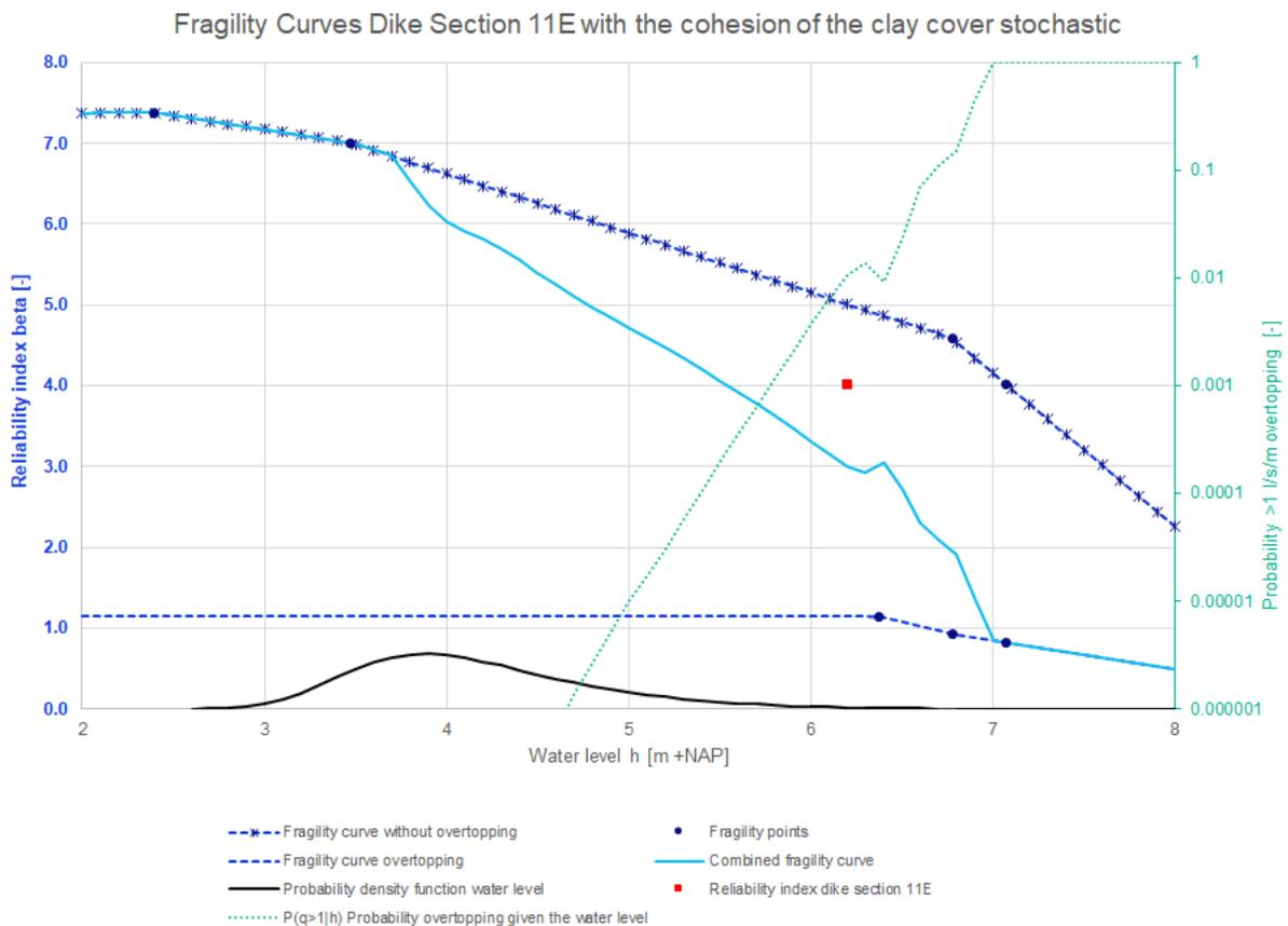
Figure 43: Fragility curves dike section 11E with the cohesion of the clay cover stochastic
