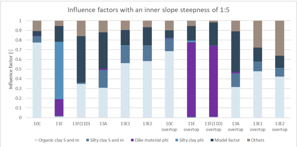
Figure 29: Influence factors with an inner slope steepness of 1:5 at WBN without overtopping and at the 1 l/s/m overtopping water level with overtopping
