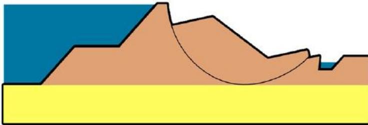
Figure 2: Schematic representation of instability of the inner slope (Jonkman, Jorissen, Schweckendiek, & Van den Bos, 2021)
