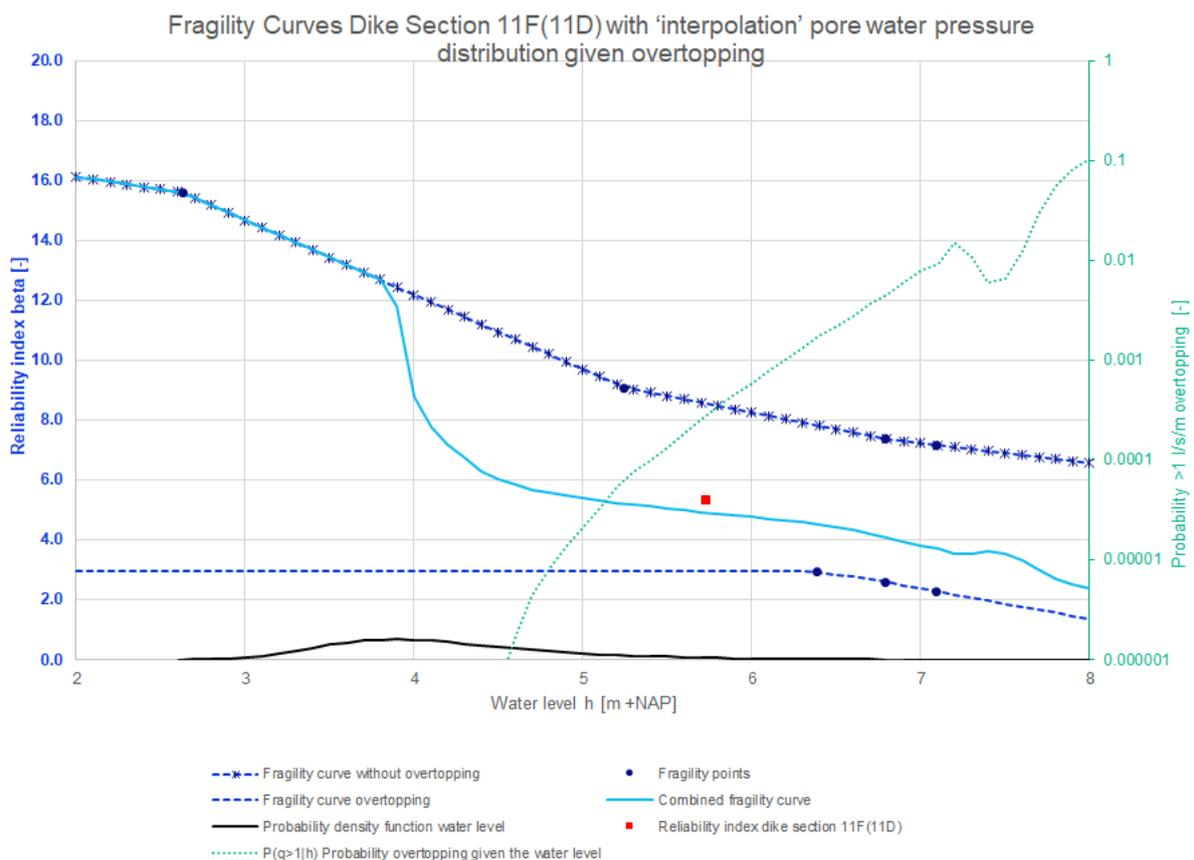
Figure 74: Fragility curves dike section 11F(11D) with ‘interpolation’ pore water pressure distribution given overtopping
