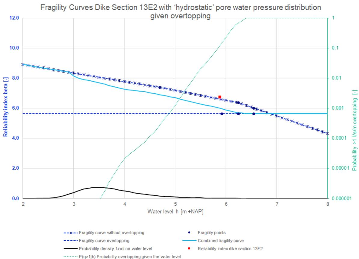
Figure 70: Fragility curves dike section 13E2 with 'hydrostatic' pore water pressure distribution given overtopping
