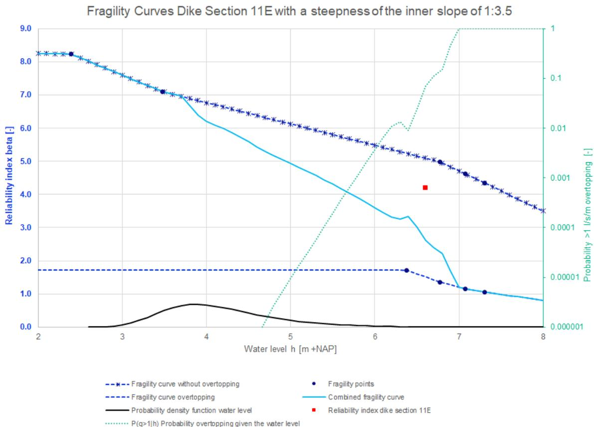
Figure 92: Fragility curves dike section 11E with a steepness of the inner slope of 1:3.5
