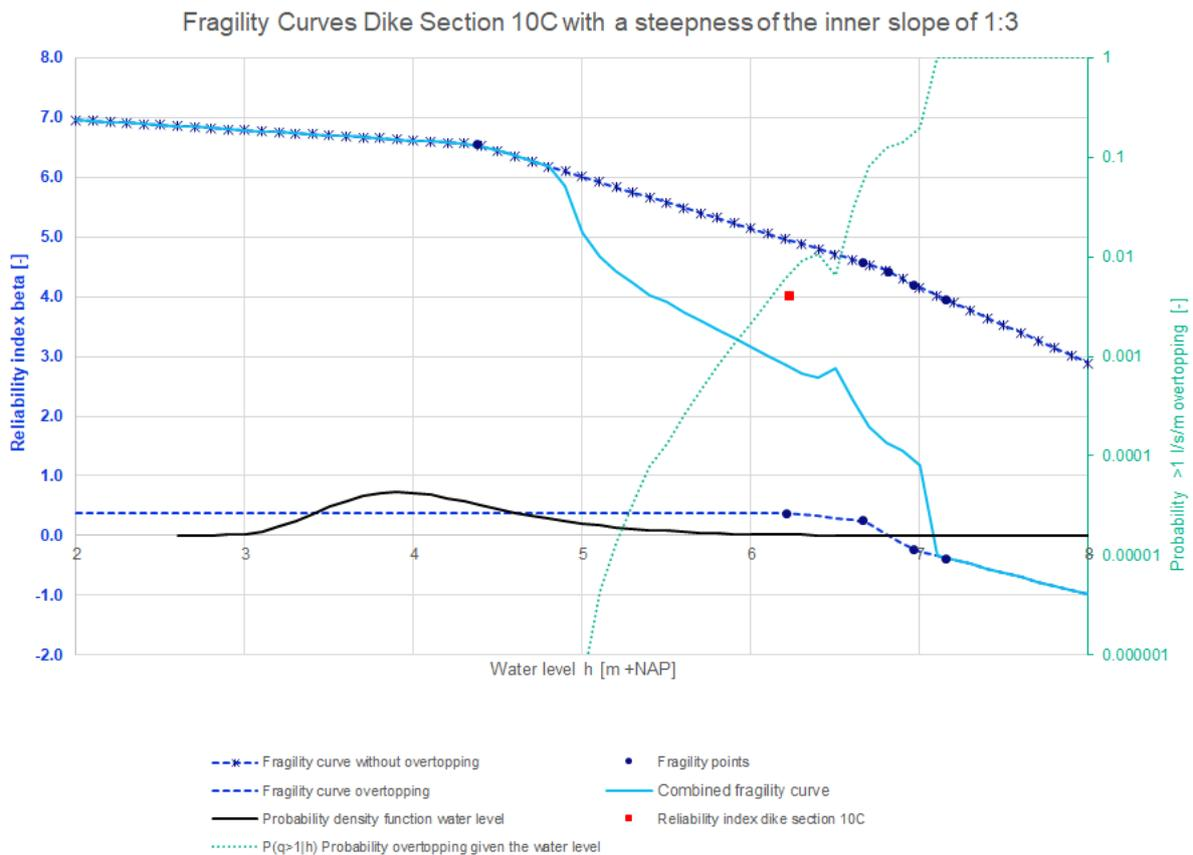
Figure 85: Fragility curves dike section 10C with a steepness of the inner slope of 1:3
