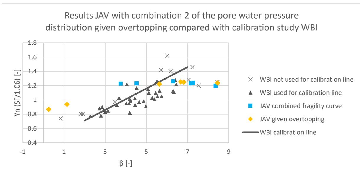
Figure 82: The results of the calculations of JAV with combination 2 of the pore water pressure distribution given overtopping compared with the calibration study of WBI. The vertical position of the results of JAV from the combined fragility curves (blue squares) are determined based on the semi-probabilistic results without overtopping
