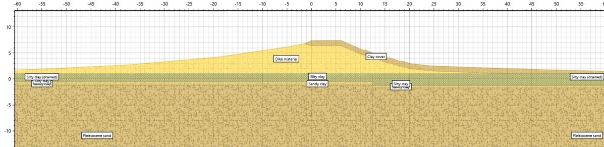
Figure 11: Schematization of dike section 11E
