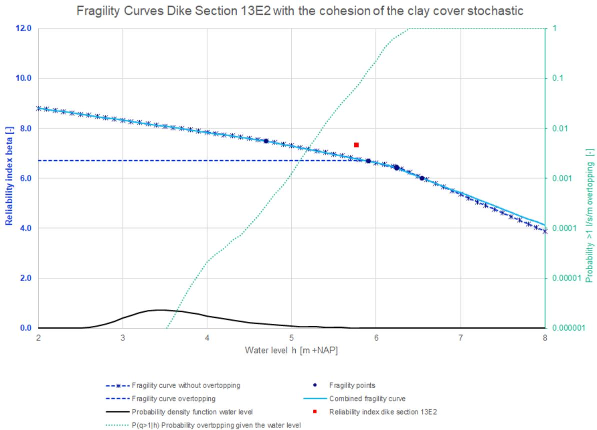
Figure 47: Fragility curves dike section 13E2 with the cohesion of the clay cover stochastic
