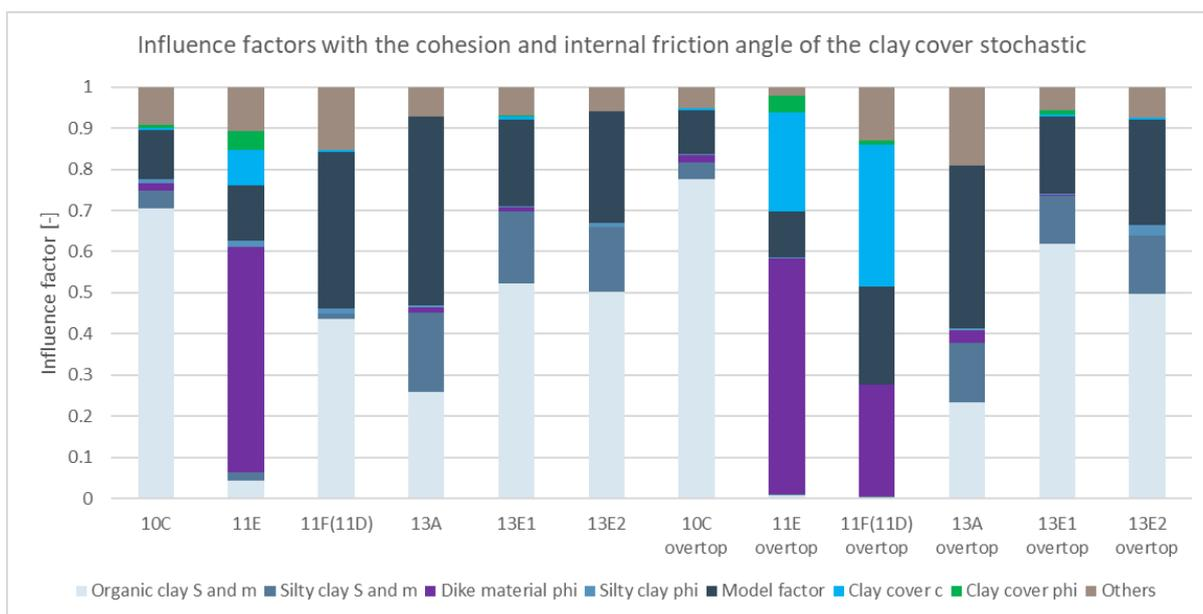
Figure 25: Influence factors with the cohesion and internal friction angle of the clay cover stochastic at WBN without overtopping and at the 1 l/s/m overtopping water level with overtopping
