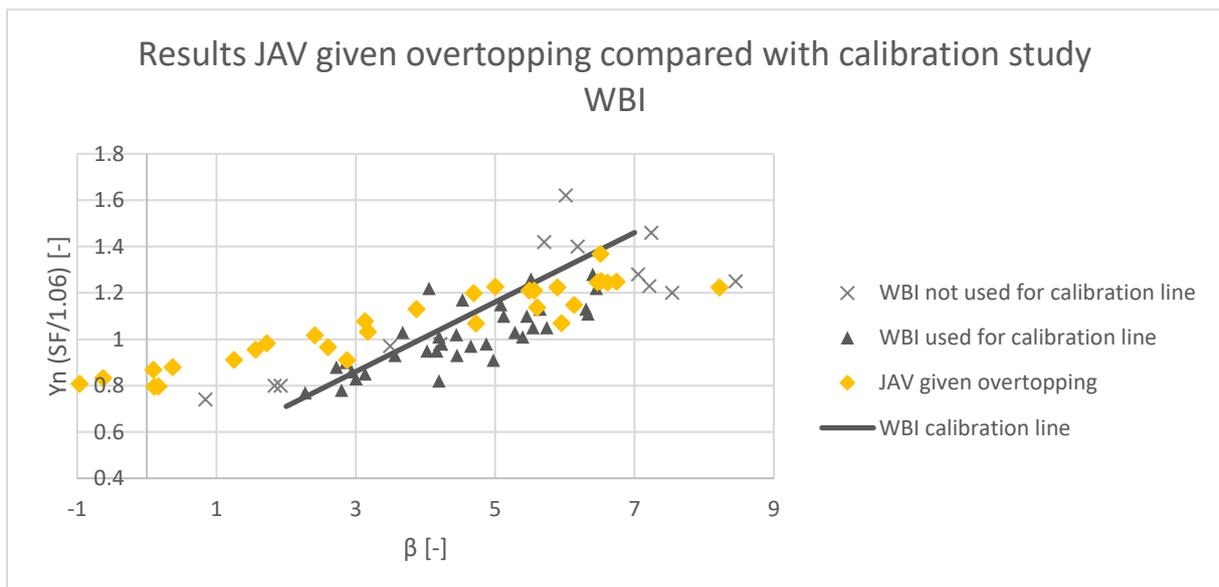
Figure 33: The results of the calculations of JAV given overtopping with different slopes compared with the calibration study of WBI
