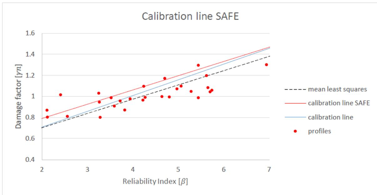
Figure 34: Calibration lines from the WBI calibration study (blue) and SAFE (red) (Prins, 2021)
