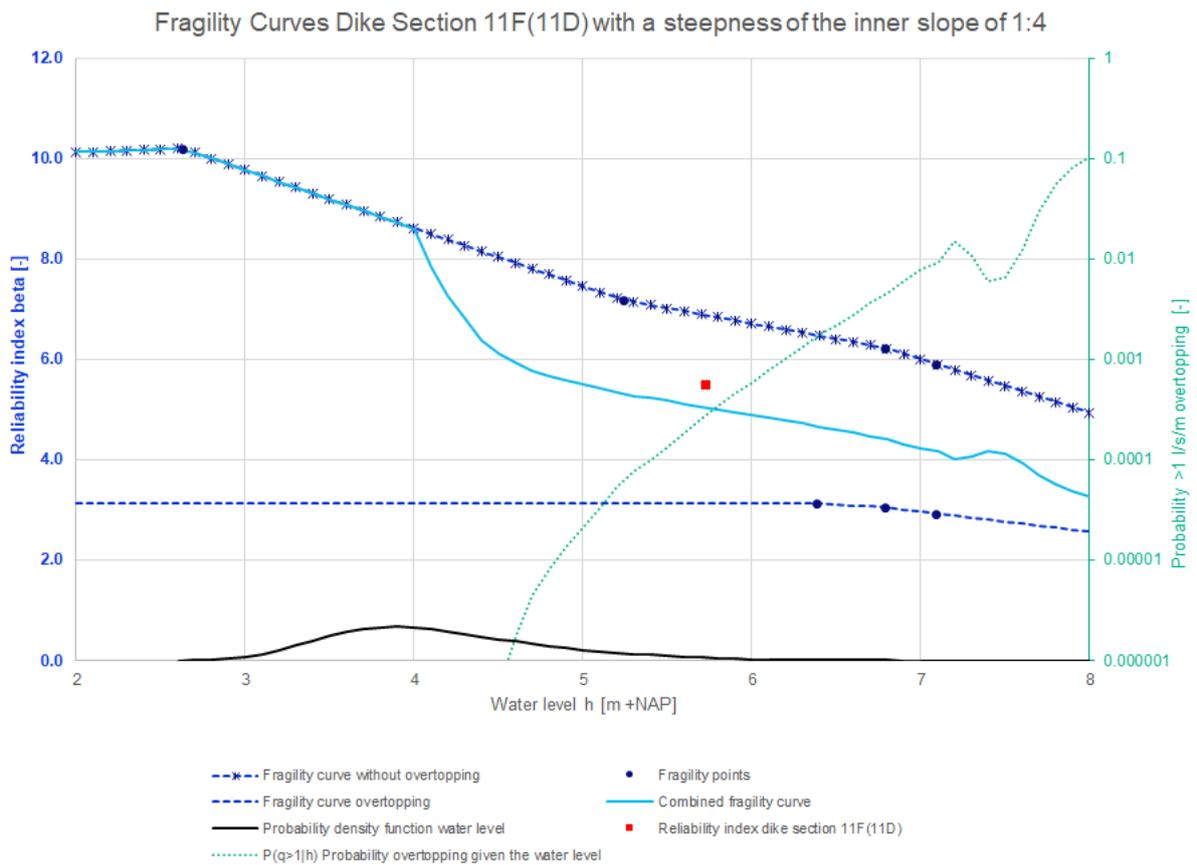
Figure 101: Fragility curves dike section 11F(11D) with a steepness of the inner slope of 1:4
