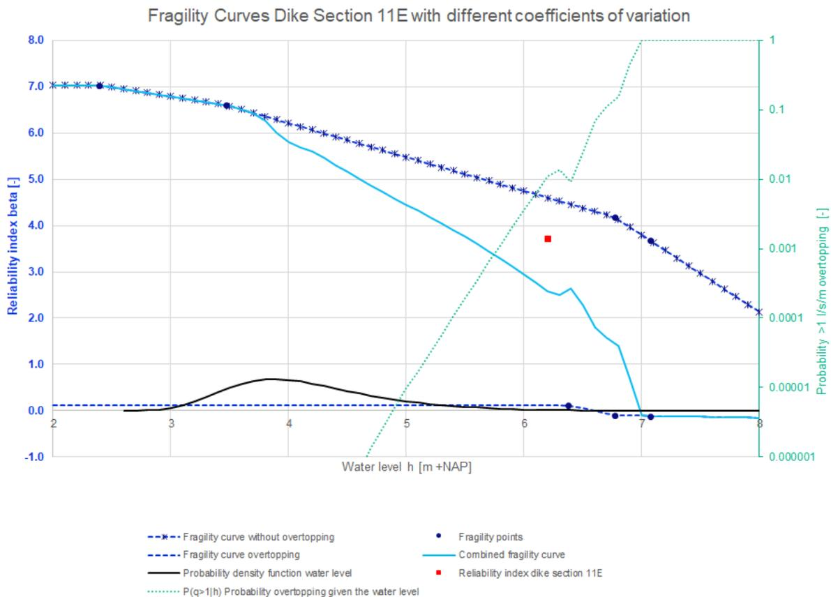
Figure 122: Fragility curves dike section 11E with different coefficients of variation
