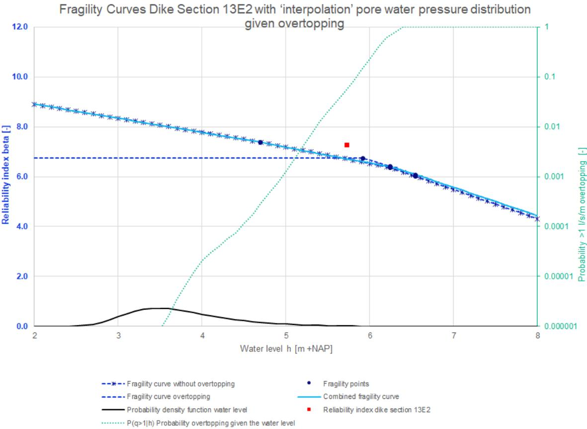
Figure 77: Fragility curves dike section 13E2 with 'interpolation' pore water pressure distribution given overtopping
