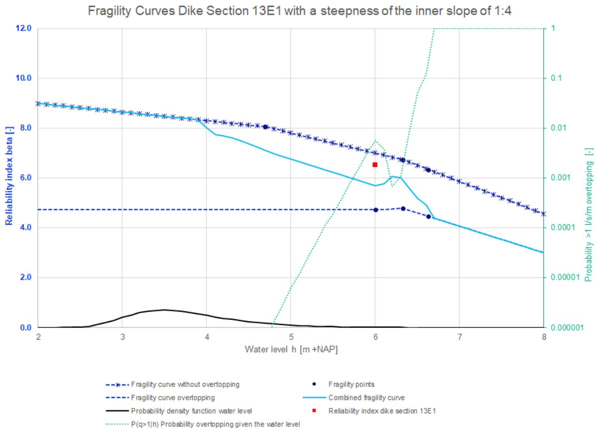
Figure 103: Fragility curves dike section 13E1 with a steepness of the inner slope of 1:4
