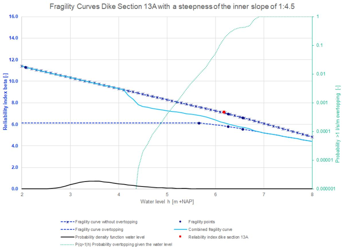
Figure 110: Fragility curves dike section 13A with a steepness of the inner slope of 1:4.5
