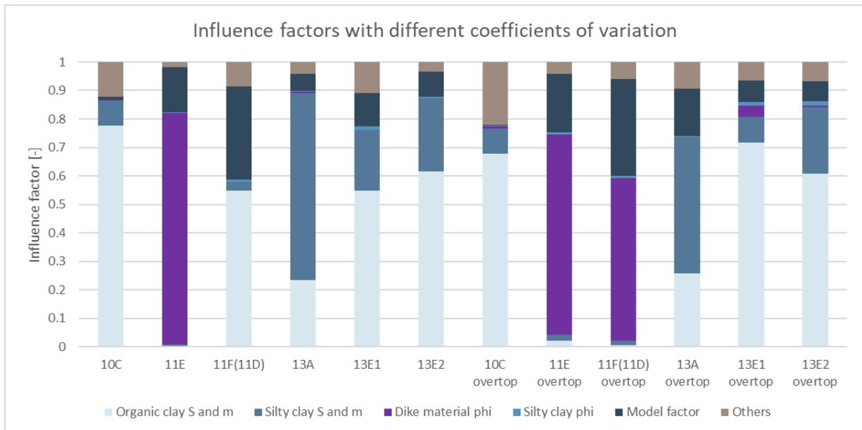
Figure 128: Influence factors with different coefficients of variation at WBN without overtopping and at the 1 l/s/m overtopping water level with overtopping
