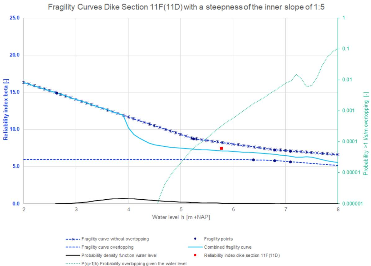
Figure 117: Fragility curves dike section 11F(11D) with a steepness of the inner slope of 1:5
