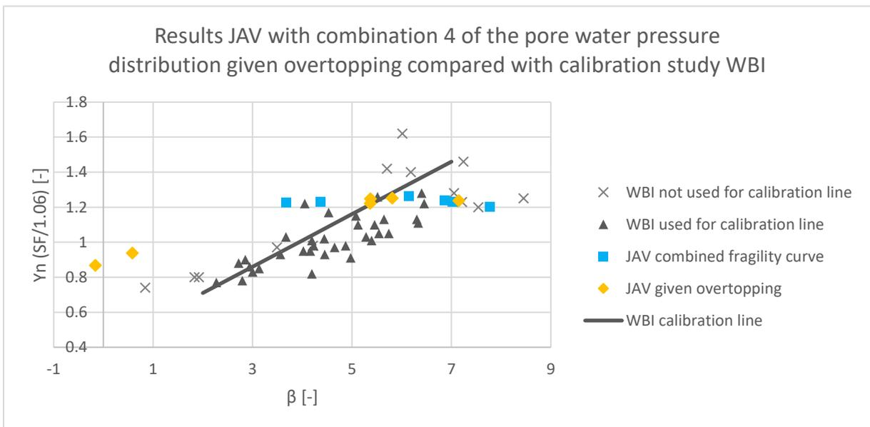
Figure 84: The results of the calculations of JAV with combination 4 of the pore water pressure distribution given overtopping compared with the calibration study of WBI. The vertical position of the results of JAV from the combined fragility curves (blue squares) are determined based on the semi-probabilistic results without overtopping
