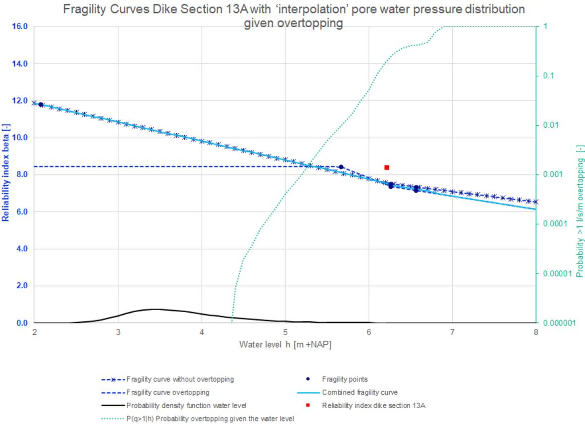
Figure 75: Fragility curves dike section 13A with ‘interpolation’ pore water pressure distribution given overtopping
