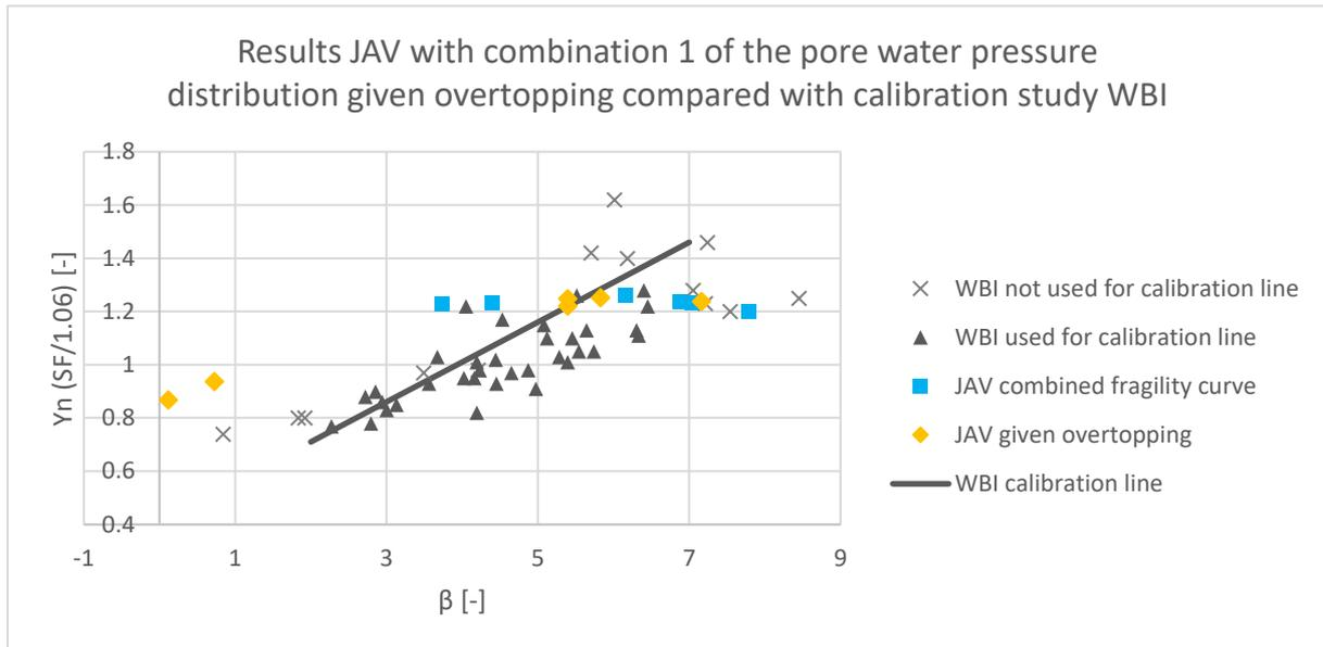
Figure 81: The results of the calculations of JAV with combination 1 of the pore water pressure distribution given overtopping compared with the calibration study of WBI. The vertical position of the results of JAV from the combined fragility curves (blue squares) are determined based on the semi-probabilistic results without overtopping
