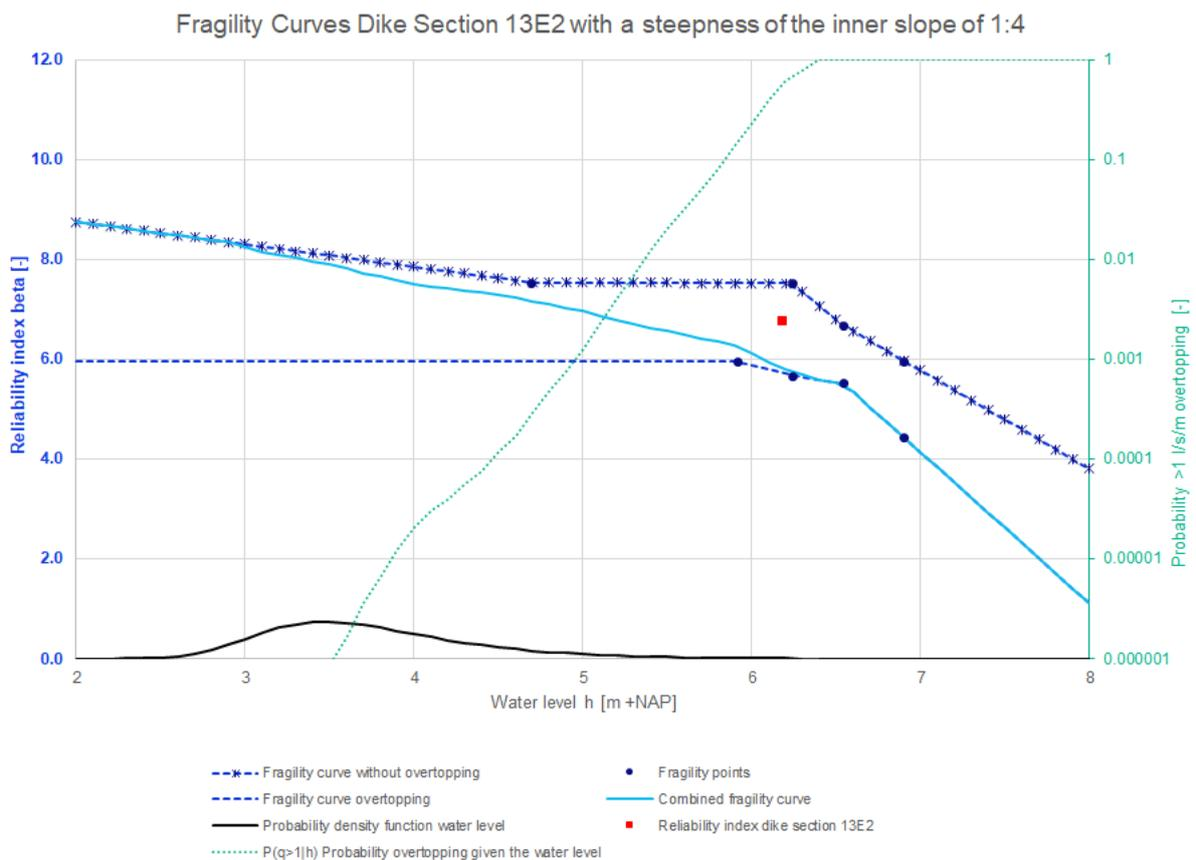
Figure 104: Fragility curves dike section 13E2 with a steepness of the inner slope of 1:4
