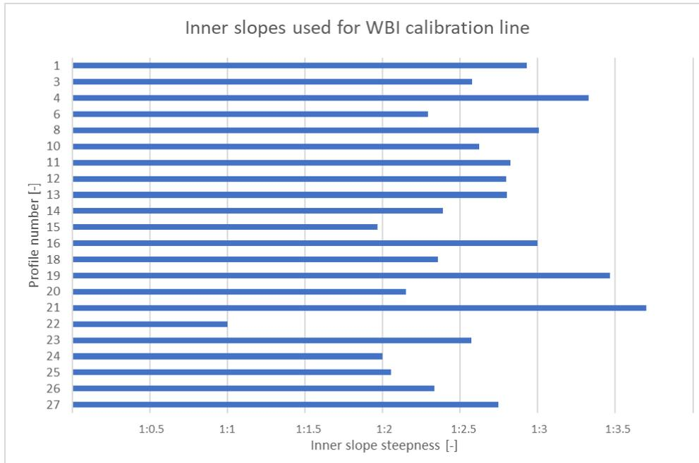
Figure 19: Inner slope steepness used during WBI calibration study
