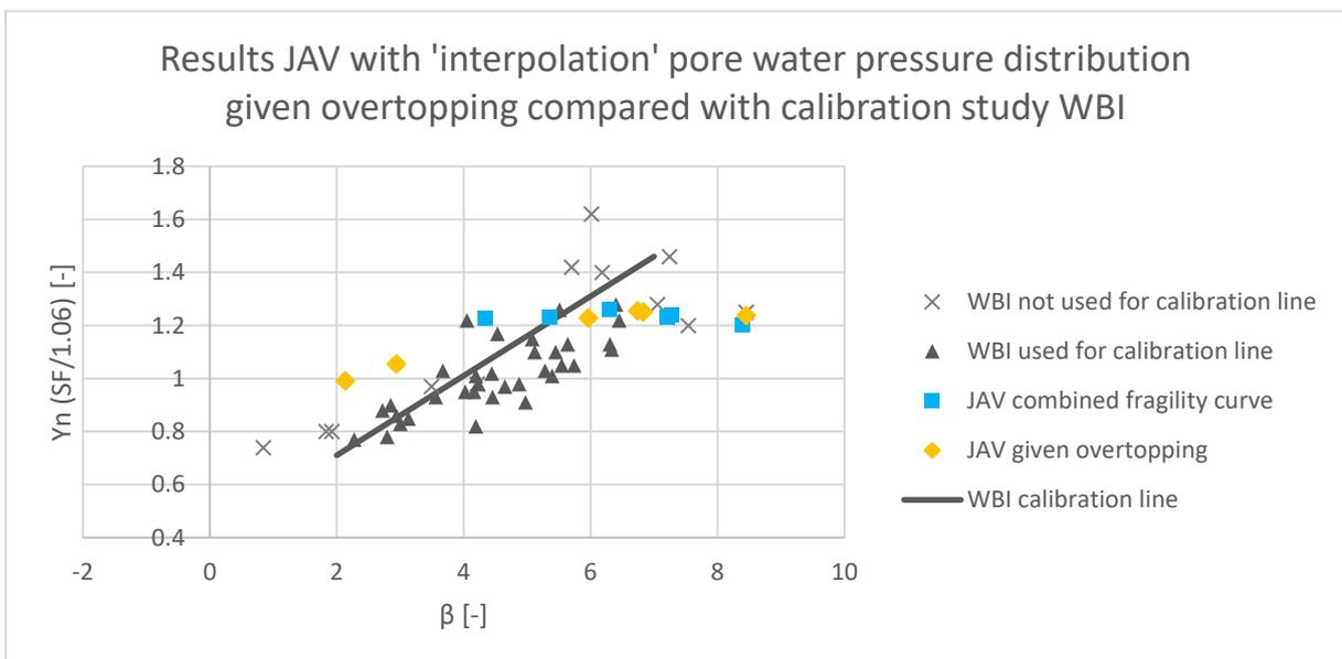
Figure 80: The results of the calculations of JAV with 'interpolation' pore water pressure distribution given overtopping compared with the calibration study of WBI. The vertical position of the results of JAV from the combined fragility curves (blue squares) are determined based on the semi-probabilistic results without overtopping
