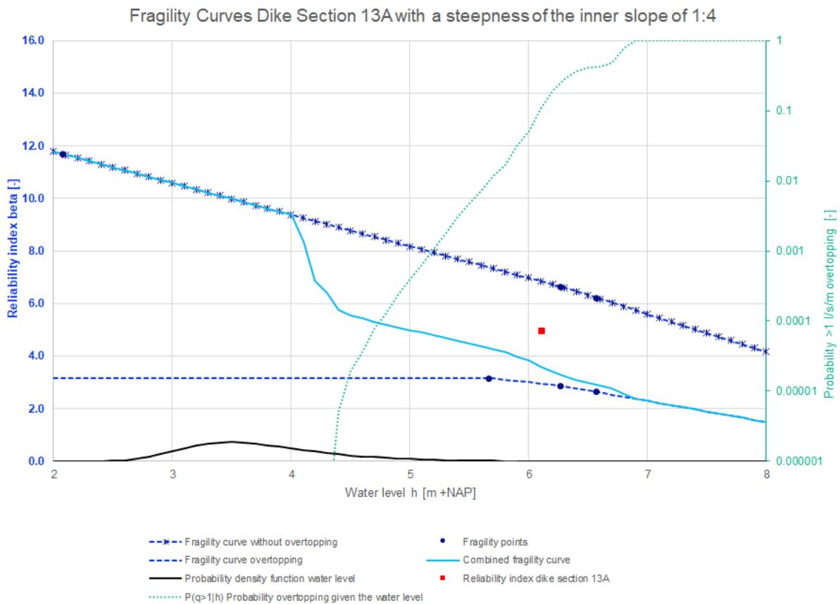
Figure 102: Fragility curves dike section 13A with a steepness of the inner slope of 1:4
