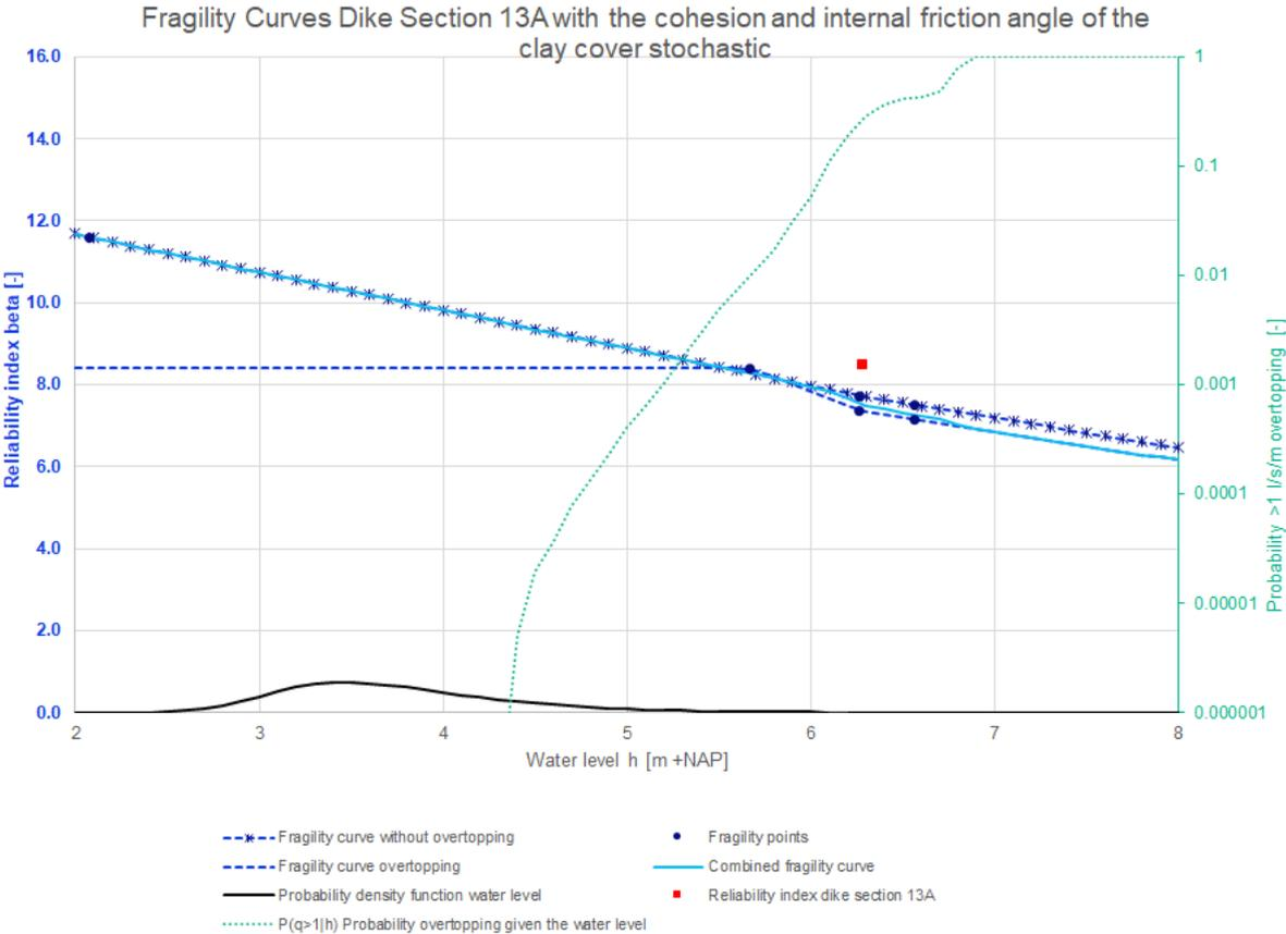
Figure 61: Fragility curves dike section 13A with the cohesion and internal friction angle of the clay cover stochastic
