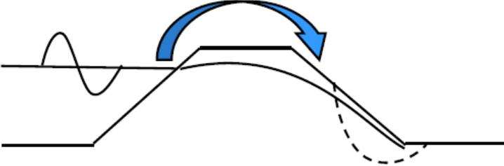
Figure 3: Schematic representation of inner slope stability with overtopping (De Visser & Jongejan, 2018)
