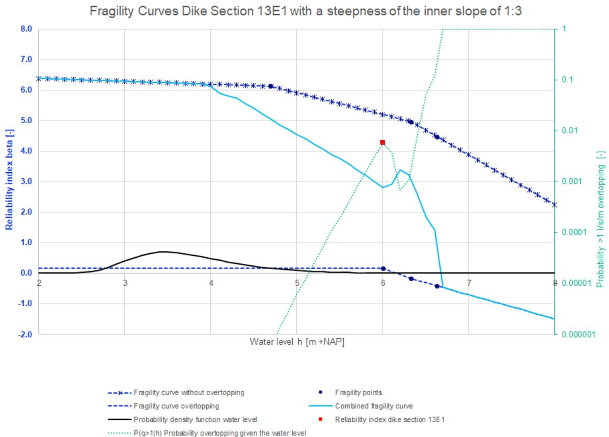
Figure 89: Fragility curves dike section 13E1 with a steepness of the inner slope of 1:3
