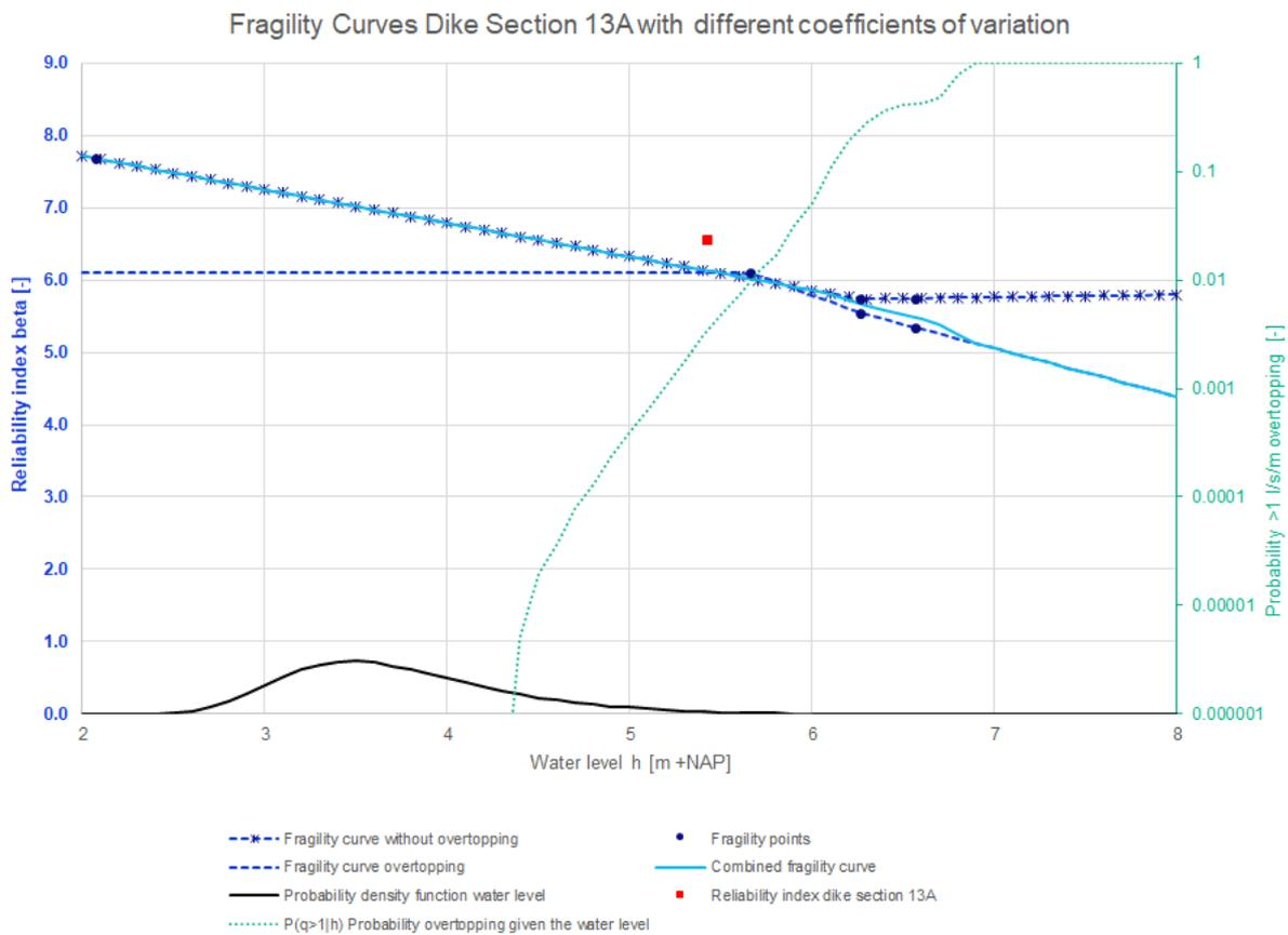
Figure 124: Fragility curves dike section 13A with different coefficients of variation
