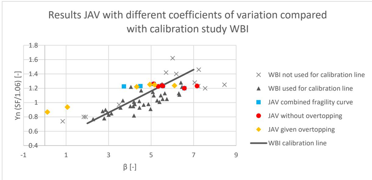
Figure 127: Results of JAV with different coefficients of variation compared with the calibration study of WBI. The vertical position of the results of JAV from the combined fragility curves (blue squares) are determined based on the semi-probabilistic results without overtopping
