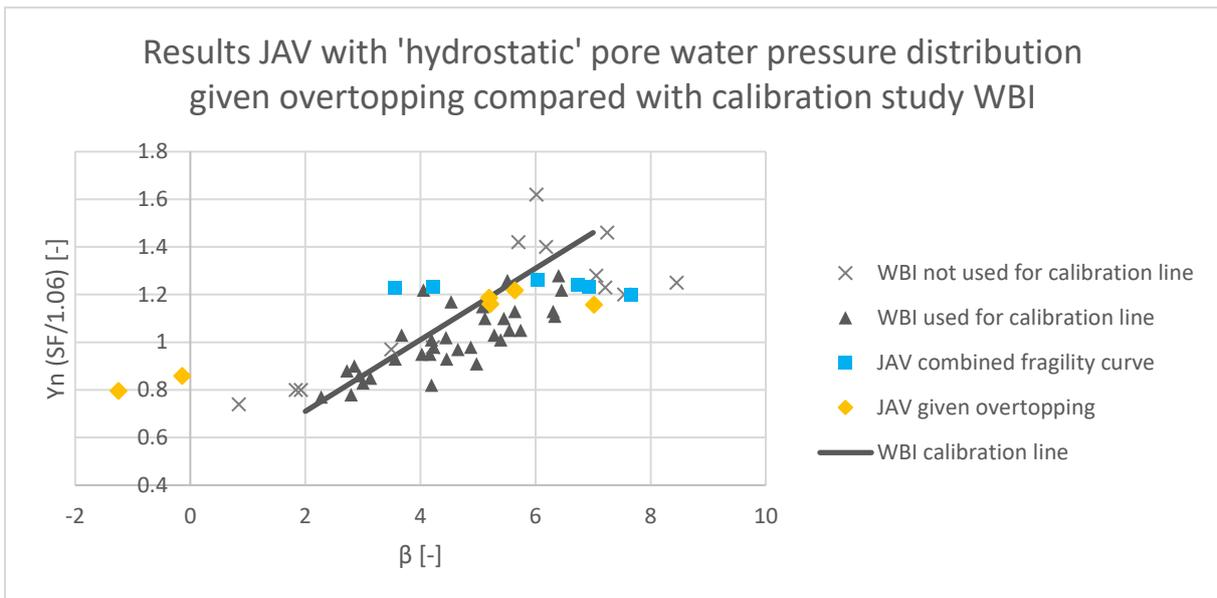
Figure 79: The results of the calculations of JAV with 'hydrostatic' pore water pressure distribution given overtopping compared with the calibration study of WBI. The vertical position of the results of JAV from the combined fragility curves (blue squares) are determined based on the semi-probabilistic results without overtopping
