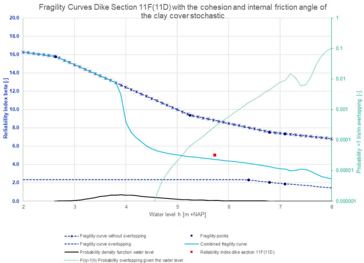
Figure 60: Fragility curves dike section 11F(11D) with the cohesion and internal friction angle of the clay cover stochastic
