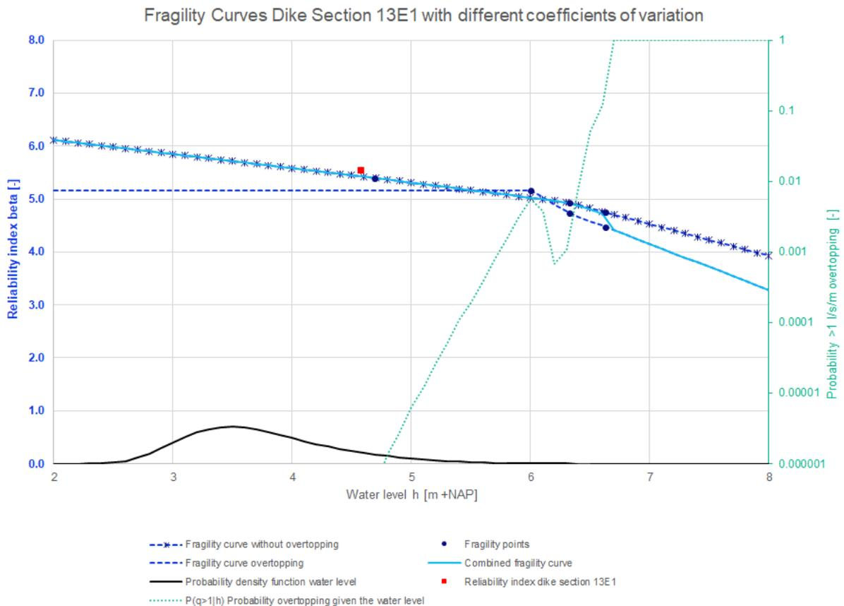
Figure 125: Fragility curves dike section 13E1 with different coefficients of variation
