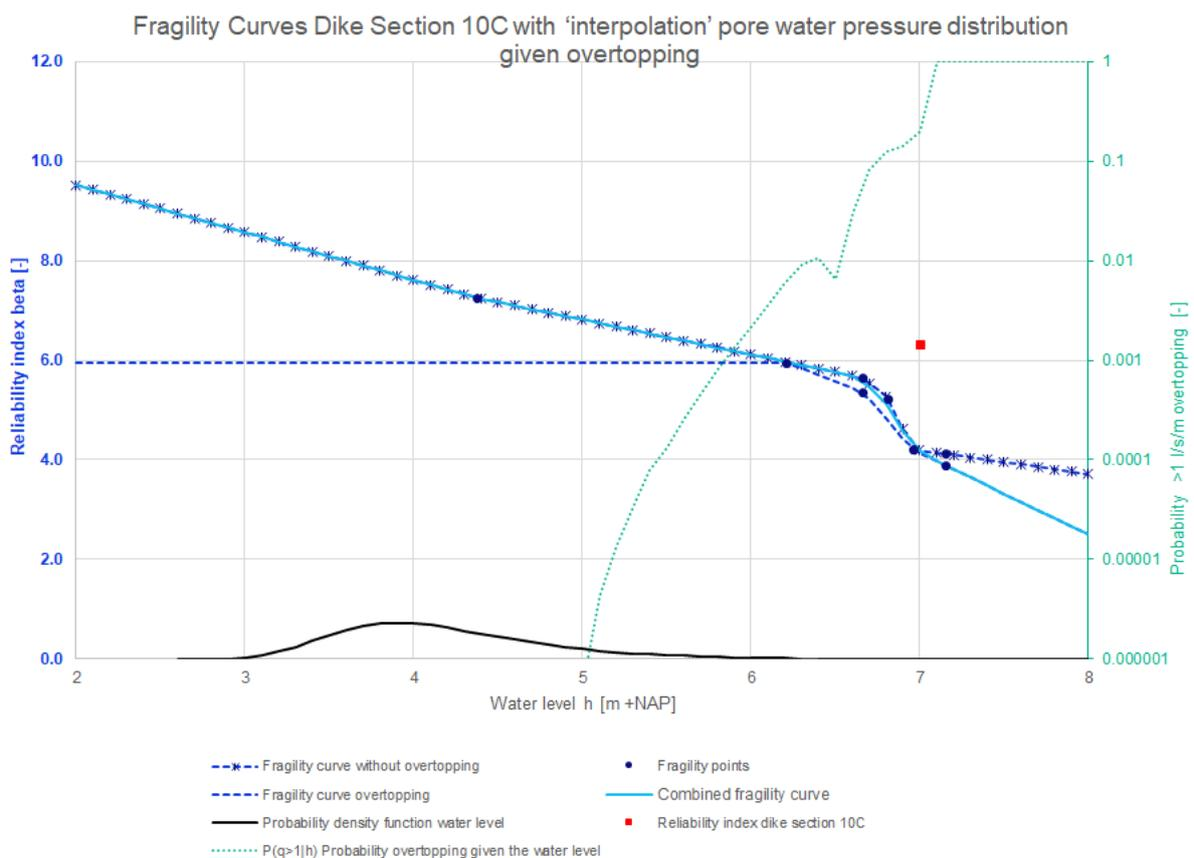
Figure 72: Fragility curves dike section 10C with 'interpolation' pore water pressure distribution given overtopping
