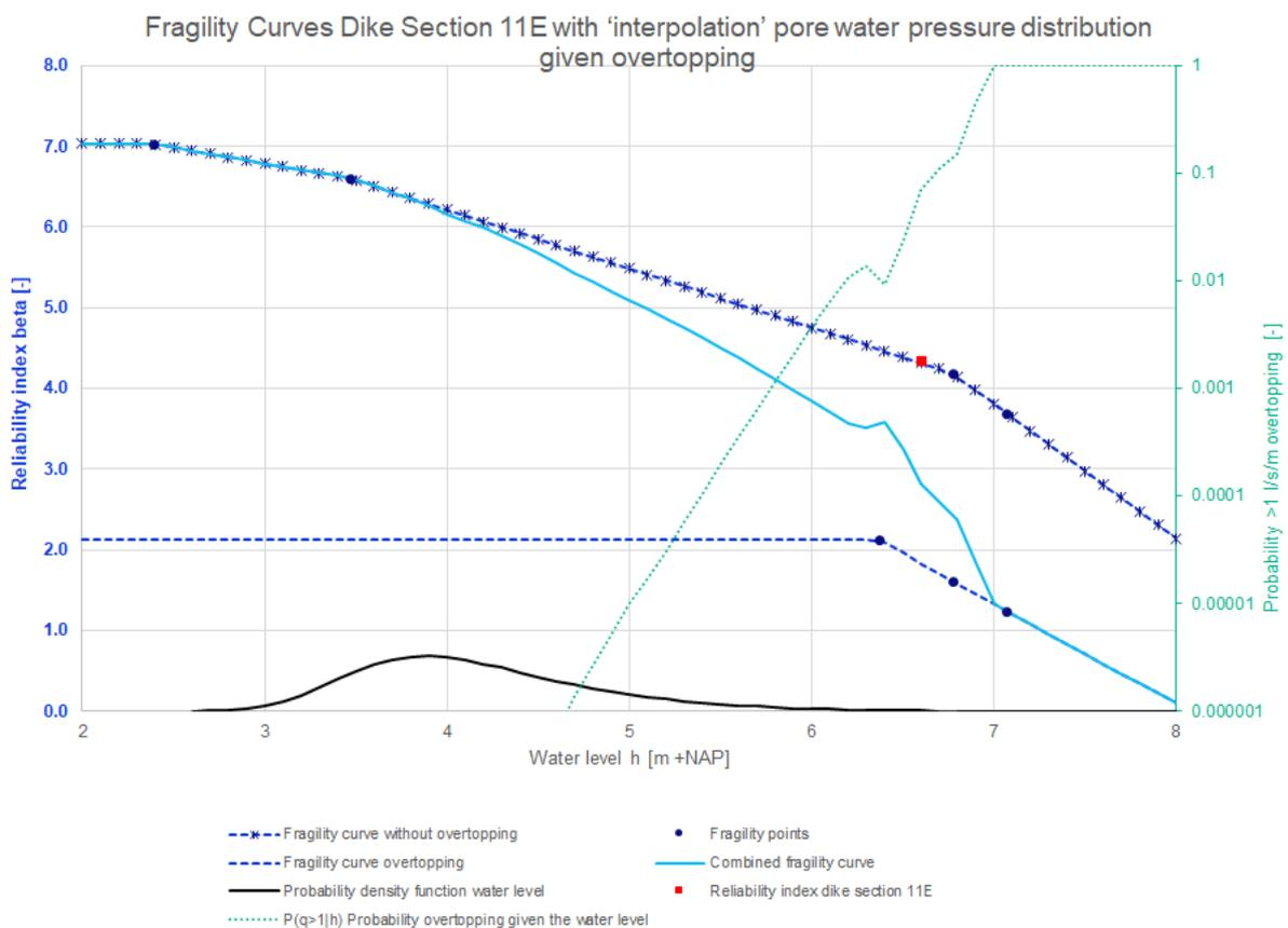
Figure 73: Fragility curves dike section 11E with ‘interpolation’ pore water pressure distribution given overtopping
