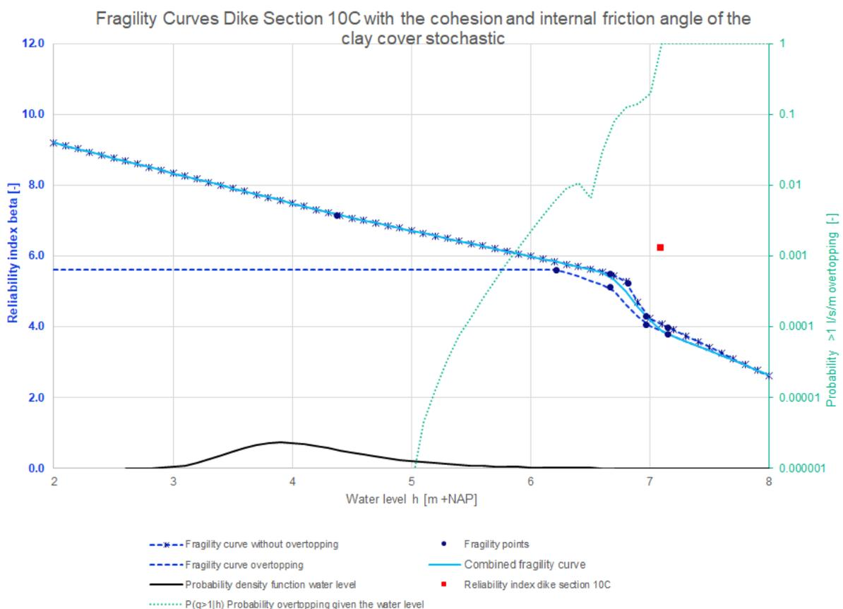
Figure 58: Fragility curves dike section 10C with the cohesion and internal friction angle of the clay cover stochastic
