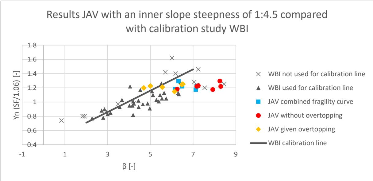
Figure 113: The results of the calculations of JAV with an inner slope steepness of 1:4.5 compared with the calibration study of WBI. The vertical position of the results of JAV from the combined fragility curves (blue squares) are determined based on the semi-probabilistic results without overtopping
