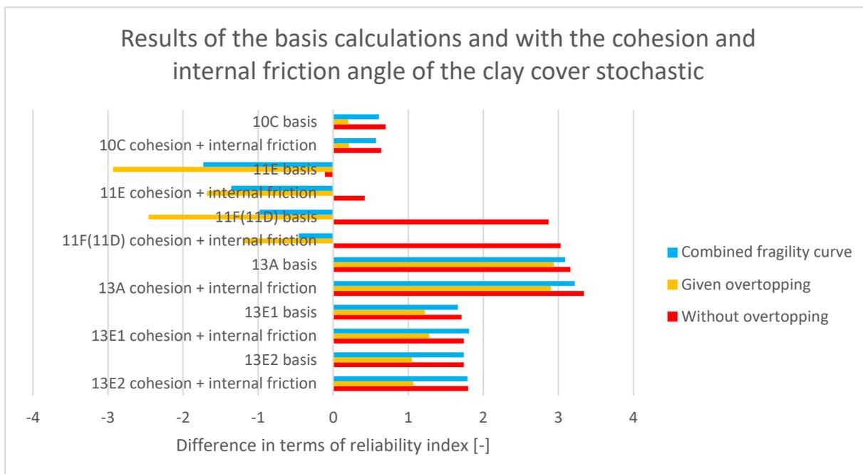
Figure 24: The results of the calculations of JAV with the cohesion and internal friction angle of the clay cover stochastic compared with the calibration study of WBI. The semi-probabilistic results without overtopping are used to determine the difference in terms of reliability index for the combined fragility curves
