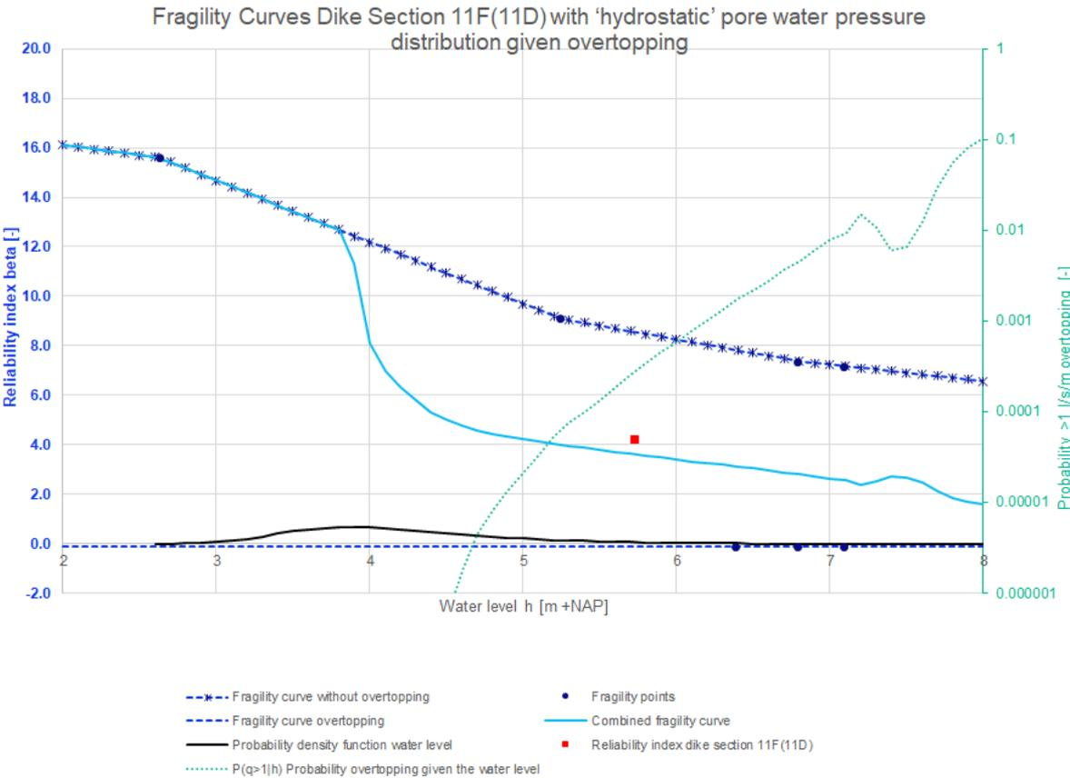
Figure 67: Fragility curves dike section 11F(11D) with 'hydrostatic' pore water pressure distribution given overtopping
