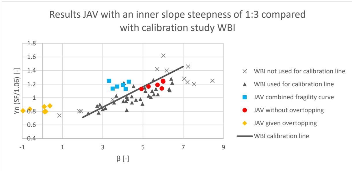
Figure 26: The results of the calculations of JAV with an inner slope steepness of 1:3 compared with the calibration study of WBI. The vertical position of the results of JAV from the combined fragility curves (blue squares) are determined based on the semi-probabilistic results without overtopping
