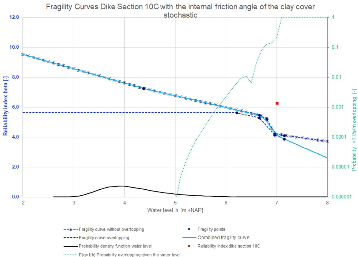
Figure 50: Fragility curves dike section 10C with the internal friction angle of the clay cover stochastic
