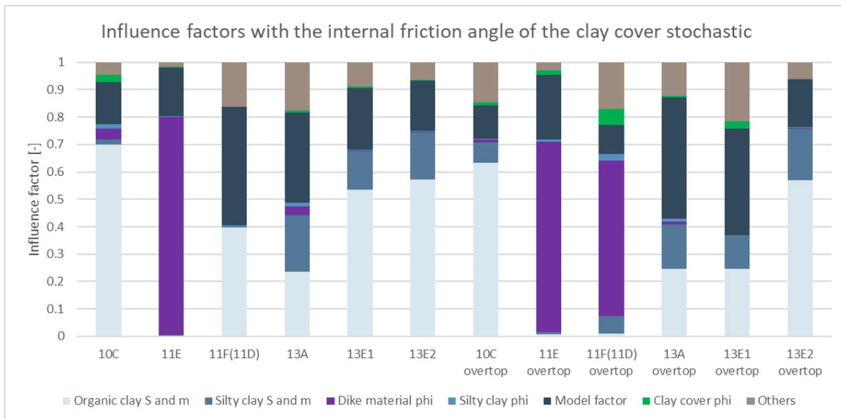
Figure 57: Influence factors with the internal friction angle of the clay cover stochastic at WBN without overtopping and at the 1 l/s/m overtopping water level with overtopping
