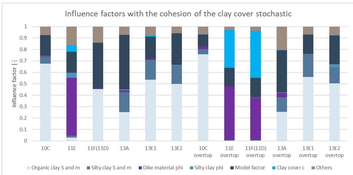
Figure 49: Influence factors with the cohesion of the clay cover stochastic at WBN without overtopping and at the 1 l/s/m overtopping water level with overtopping
