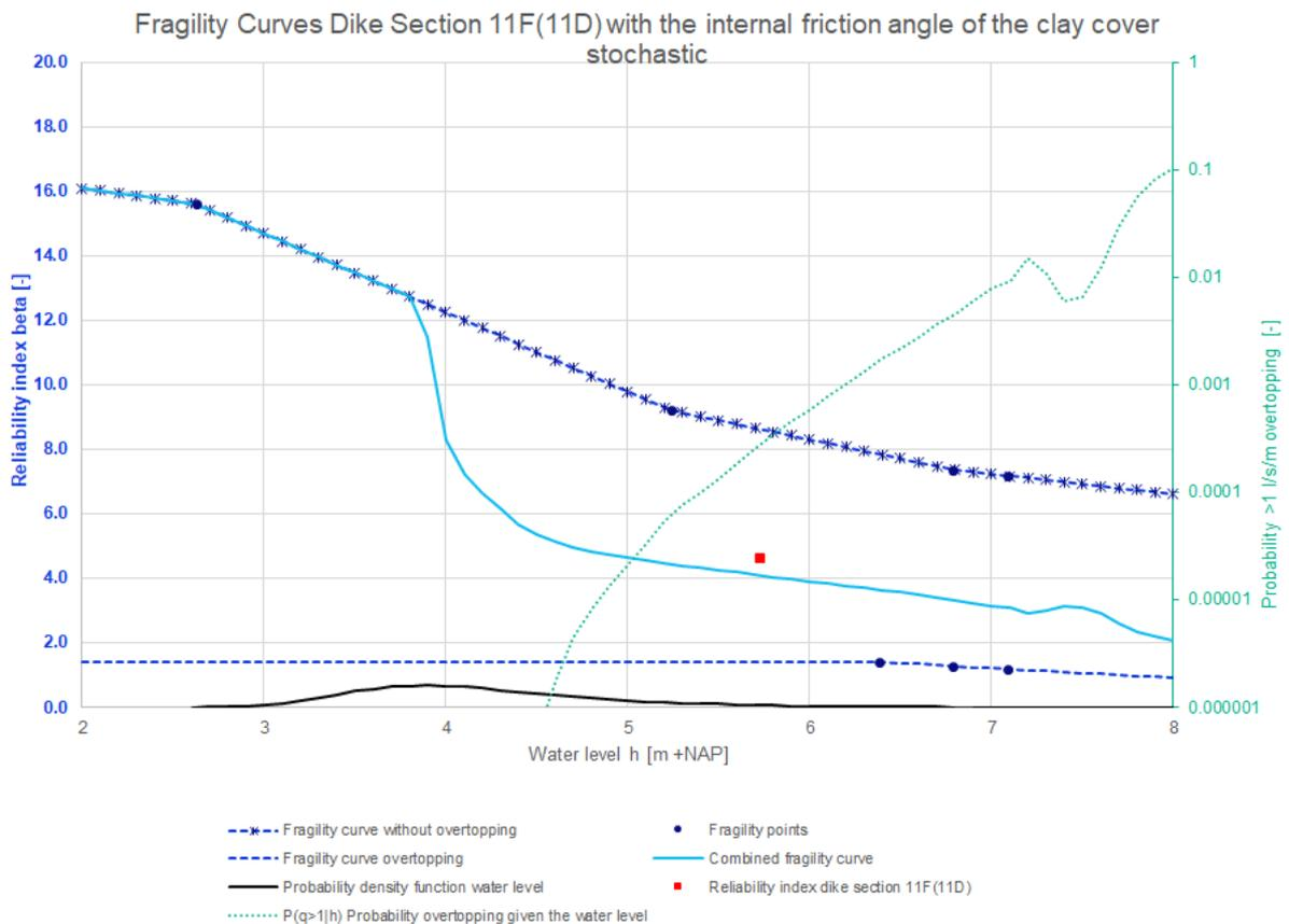
Figure 52: Fragility curves dike section 11F(11D) with the internal friction angle of the clay cover stochastic
