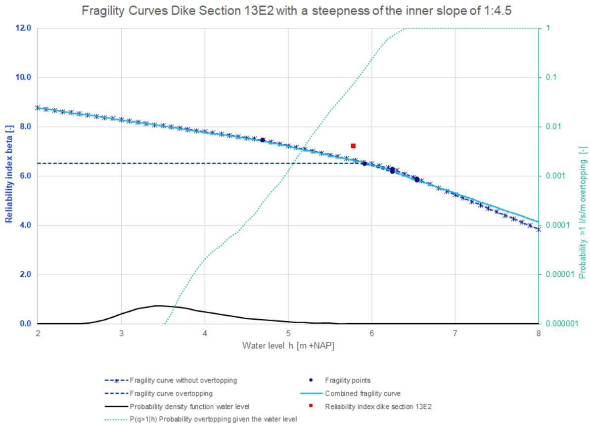
Figure 112: Fragility curves dike section 13E2 with a steepness of the inner slope of 1:4.5
