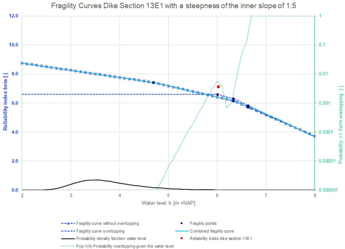
Figure 119: Fragility curves dike section 13E1 with a steepness of the inner slope of 1:5
