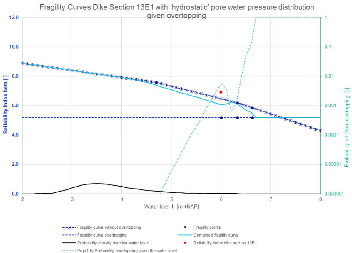
Figure 69: Fragility curves dike section 13E1 with 'hydrostatic' pore water pressure distribution given overtopping
