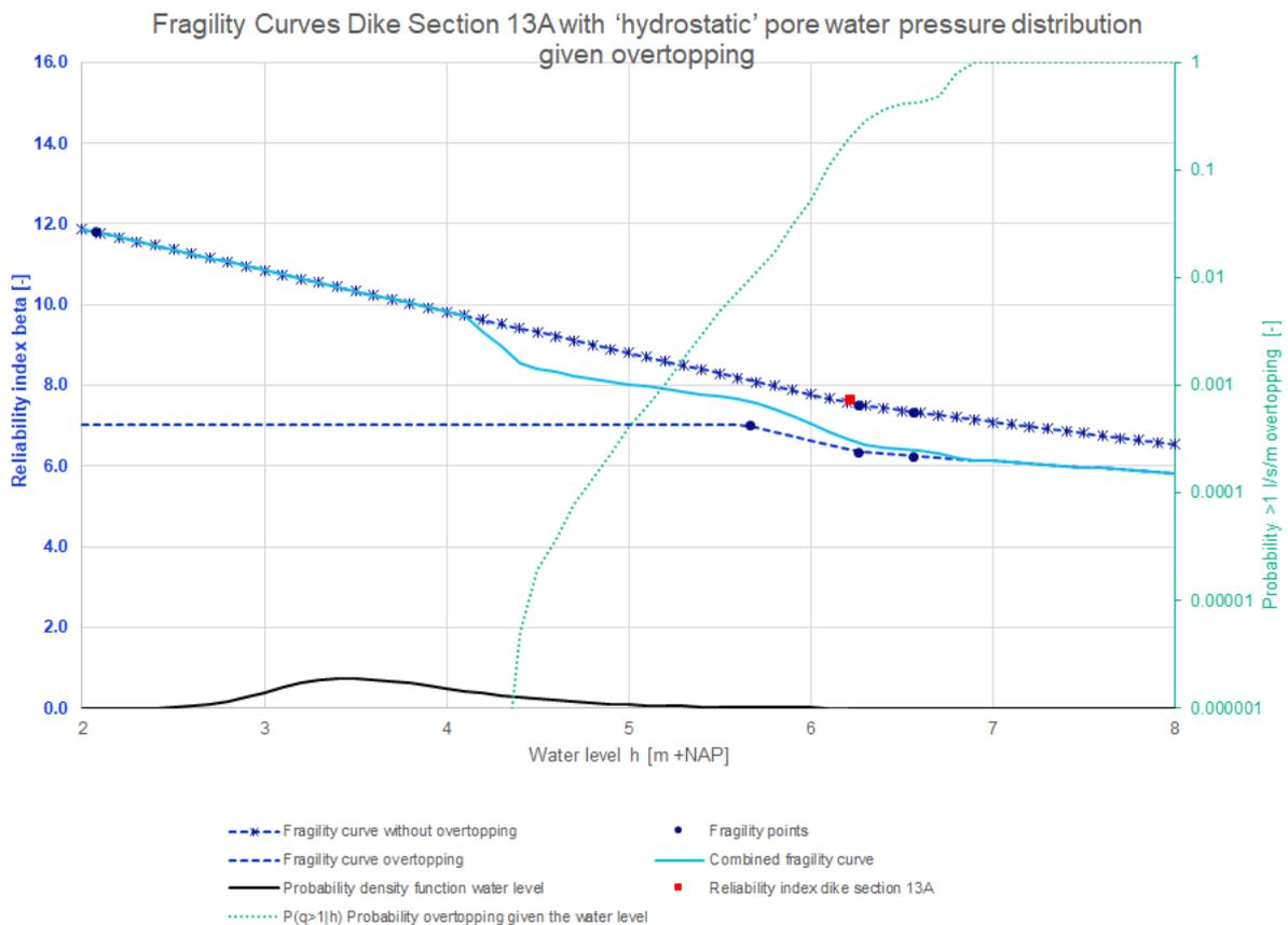
Figure 68: Fragility curves dike section 13A with 'hydrostatic' pore water pressure distribution given overtopping
