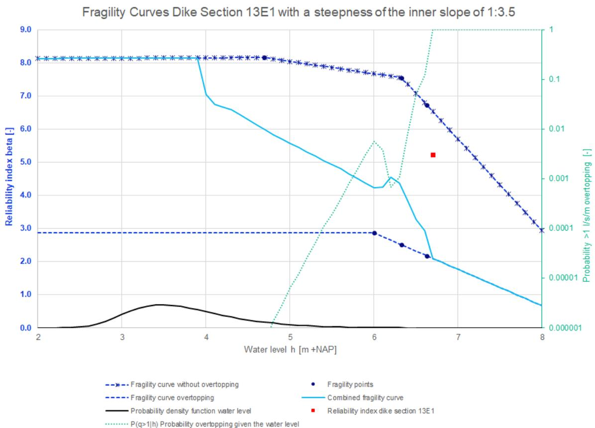
Figure 95: Fragility curves dike section 13E1 with a steepness of the inner slope of 1:3.5
