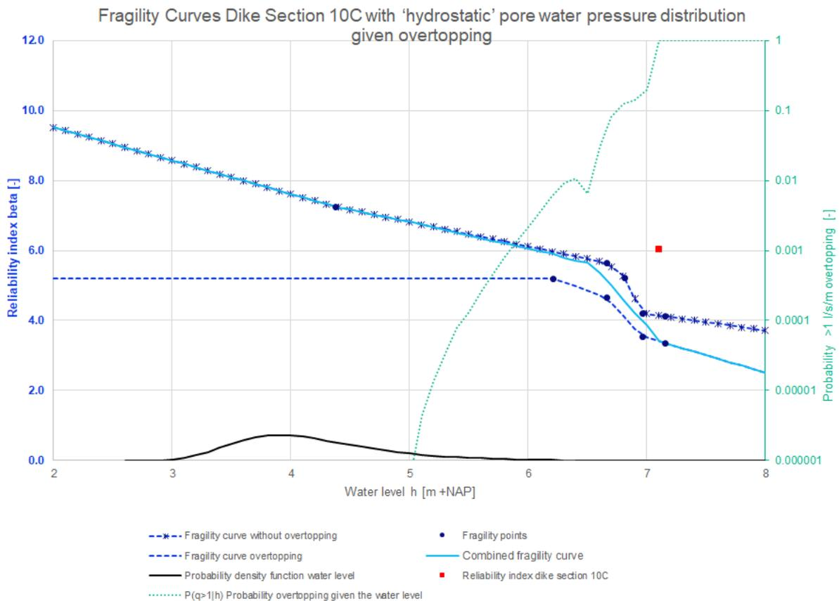
Figure 65: Fragility curves dike section 10C with 'hydrostatic' pore water pressure distribution given overtopping
