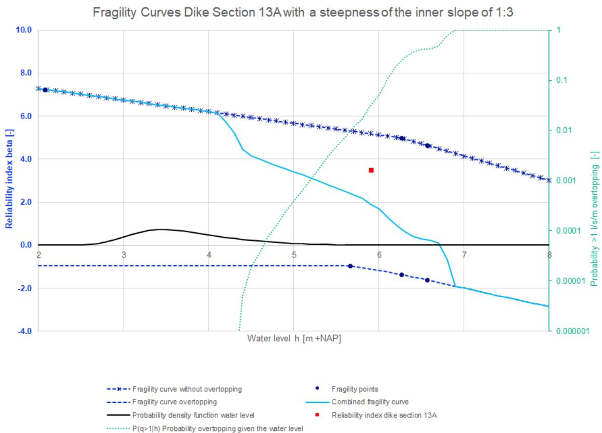
Figure 88: Fragility curves dike section 13A with a steepness of the inner slope of 1:3
