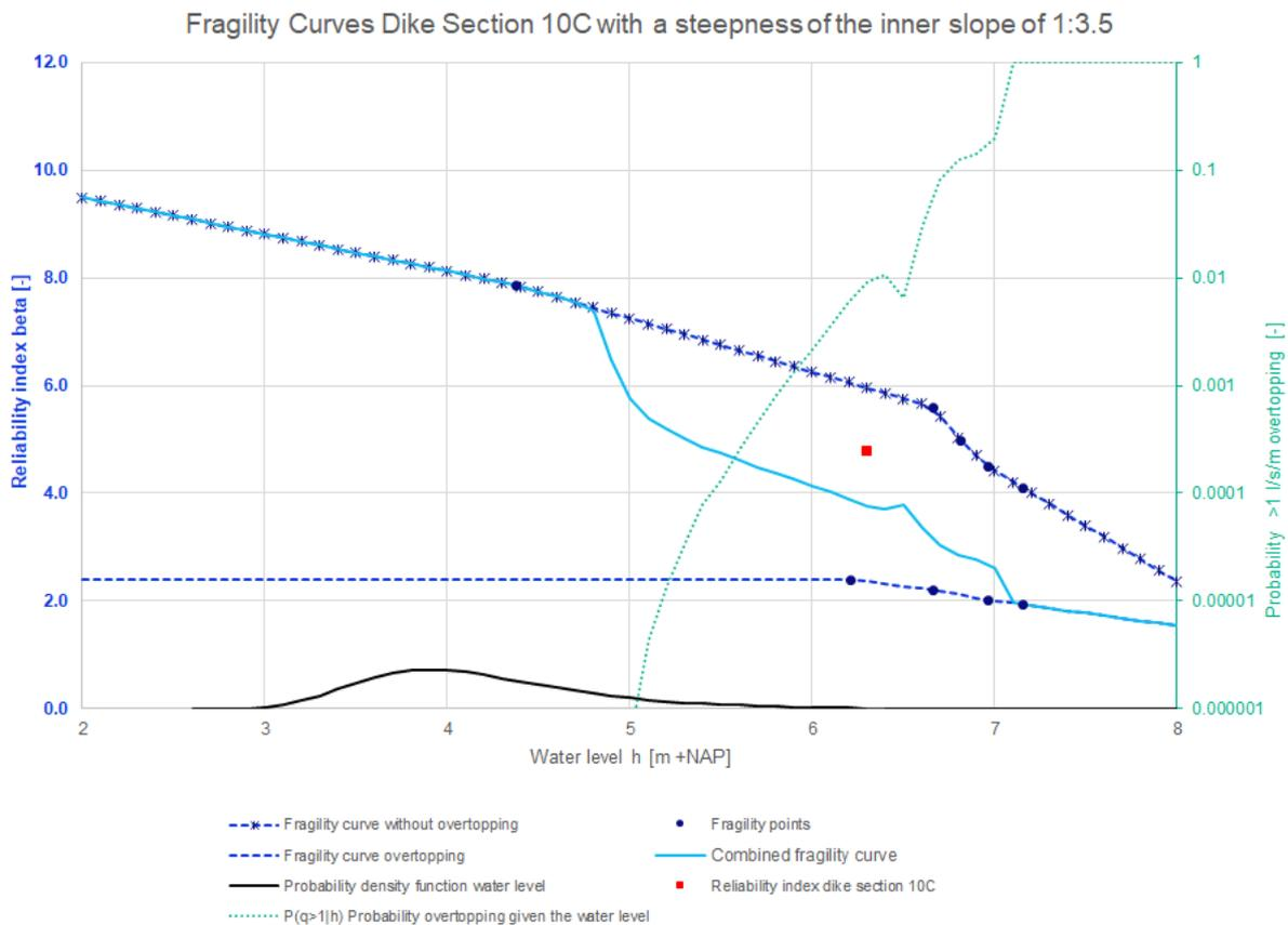
Figure 91: Fragility curves dike section 10C with a steepness of the inner slope of 1:3.5
