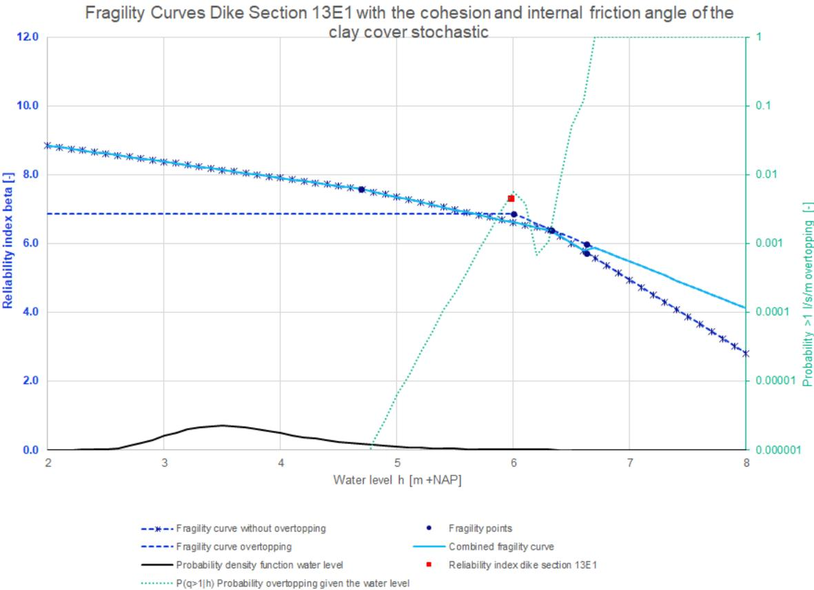
Figure 62: Fragility curves dike section 13E1 with the cohesion and internal friction angle of the clay cover stochastic
