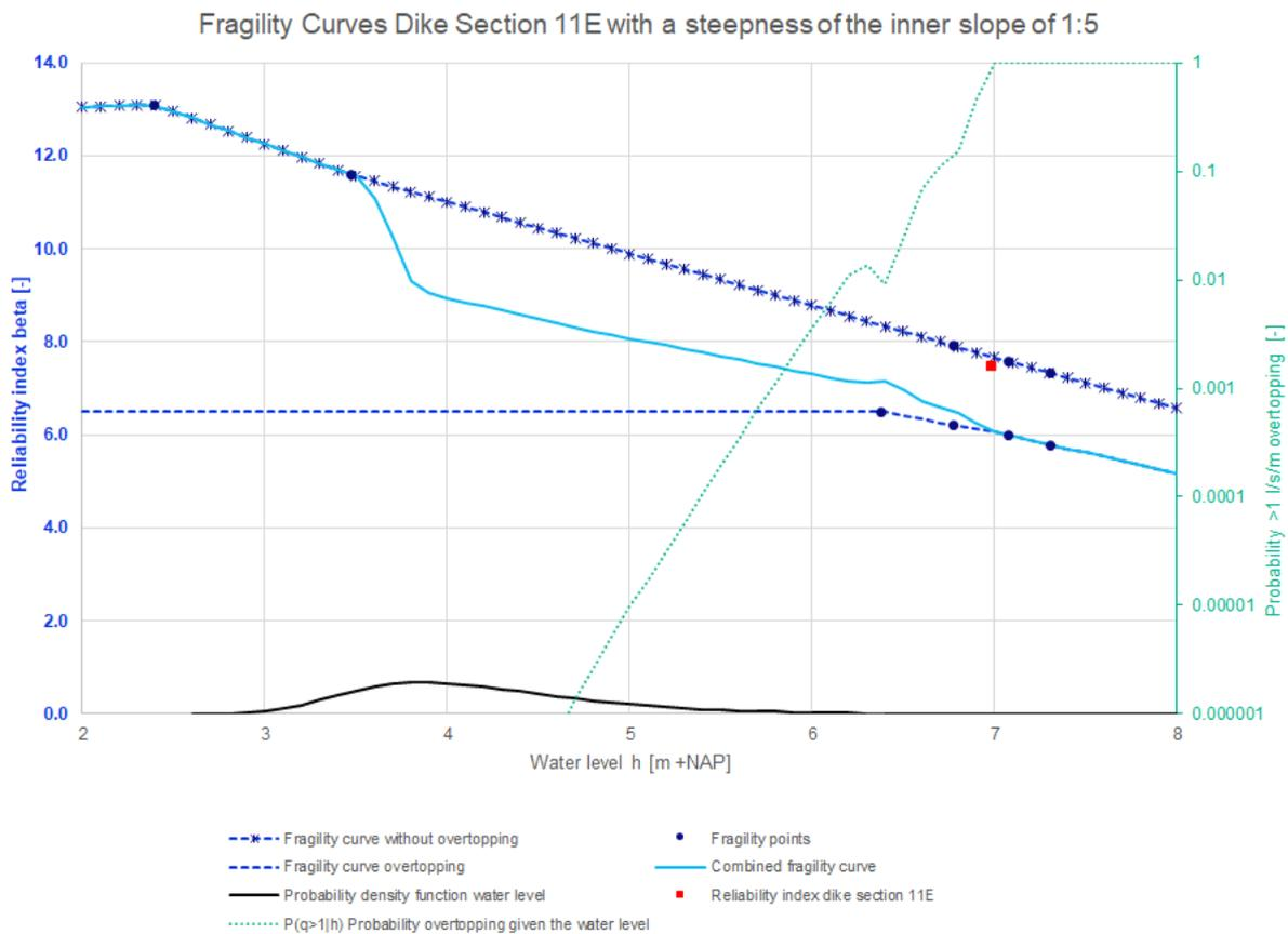
Figure 116: Fragility curves dike section 11E with a steepness of the inner slope of 1:5
