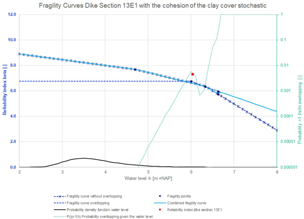
Figure 46: Fragility curves dike section 13E1 with the cohesion of the clay cover stochastic
