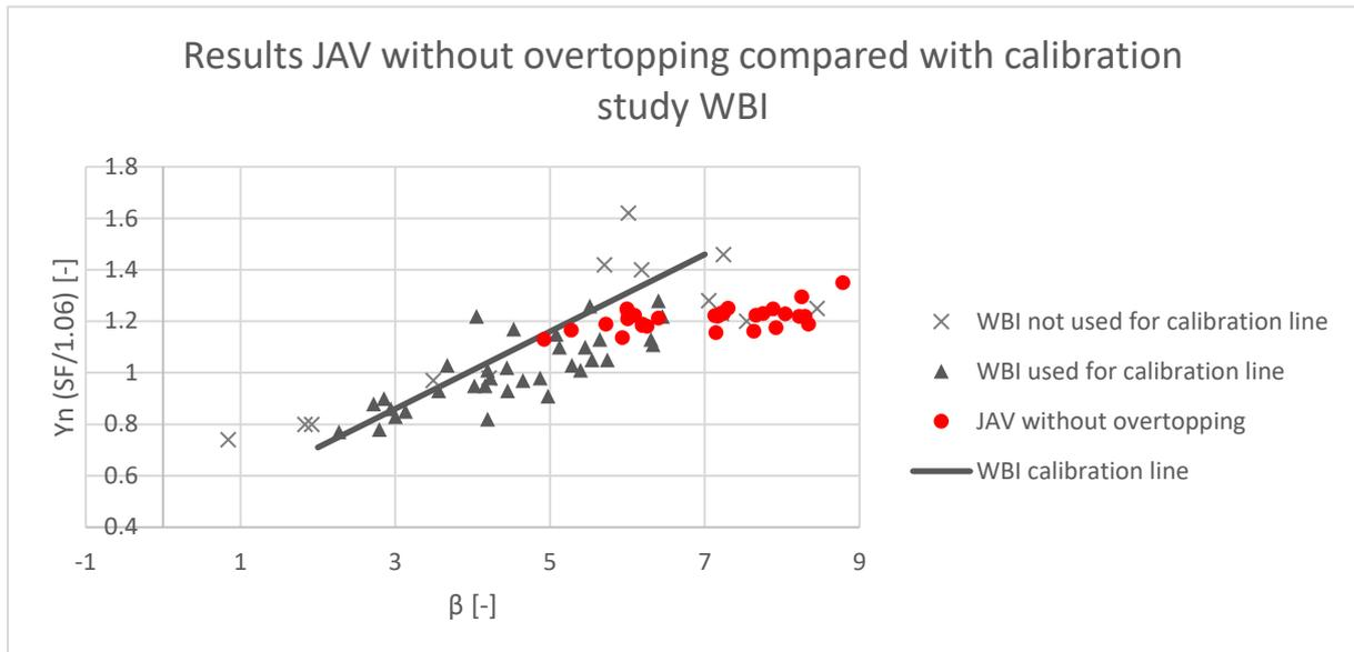
Figure 31: The results of the calculations of JAV without overtopping with different slopes compared with the calibration study of WBI.
