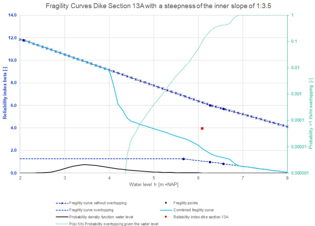
Figure 94: Fragility curves dike section 13A with a steepness of the inner slope of 1:3.5
