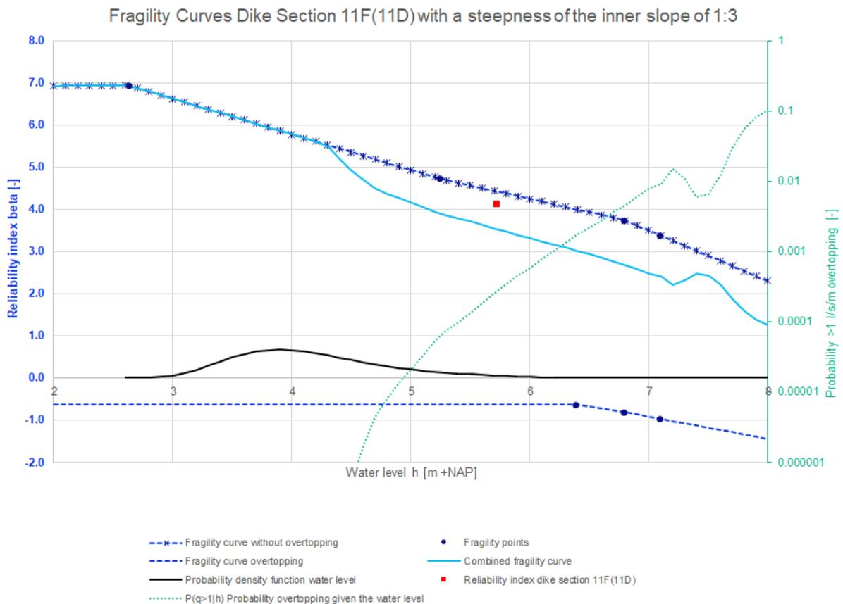
Figure 87: Fragility curves dike section 11F(11D) with a steepness of the inner slope of 1:3
