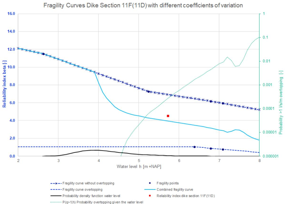
Figure 123: Fragility curves dike section 11F(11D) with different coefficients of variation
