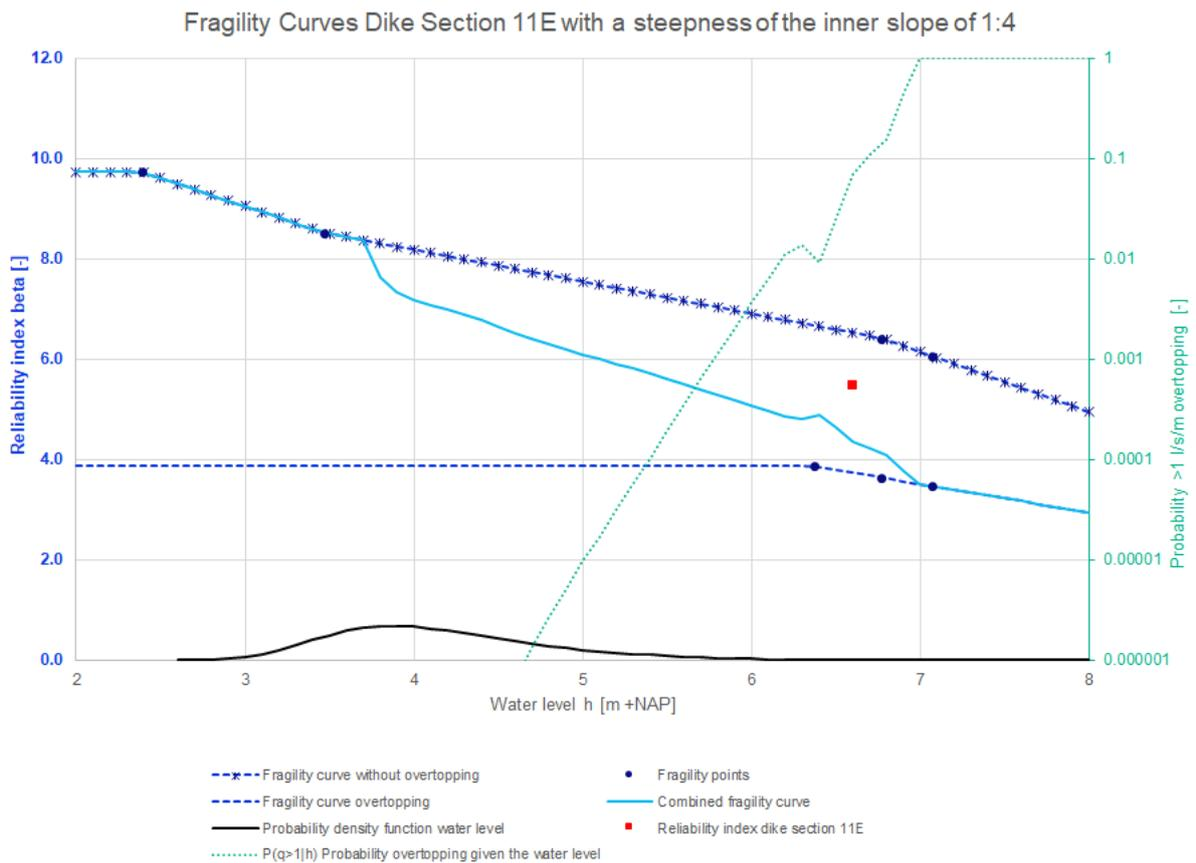
Figure 100: Fragility curves dike section 11E with a steepness of the inner slope of 1:4
