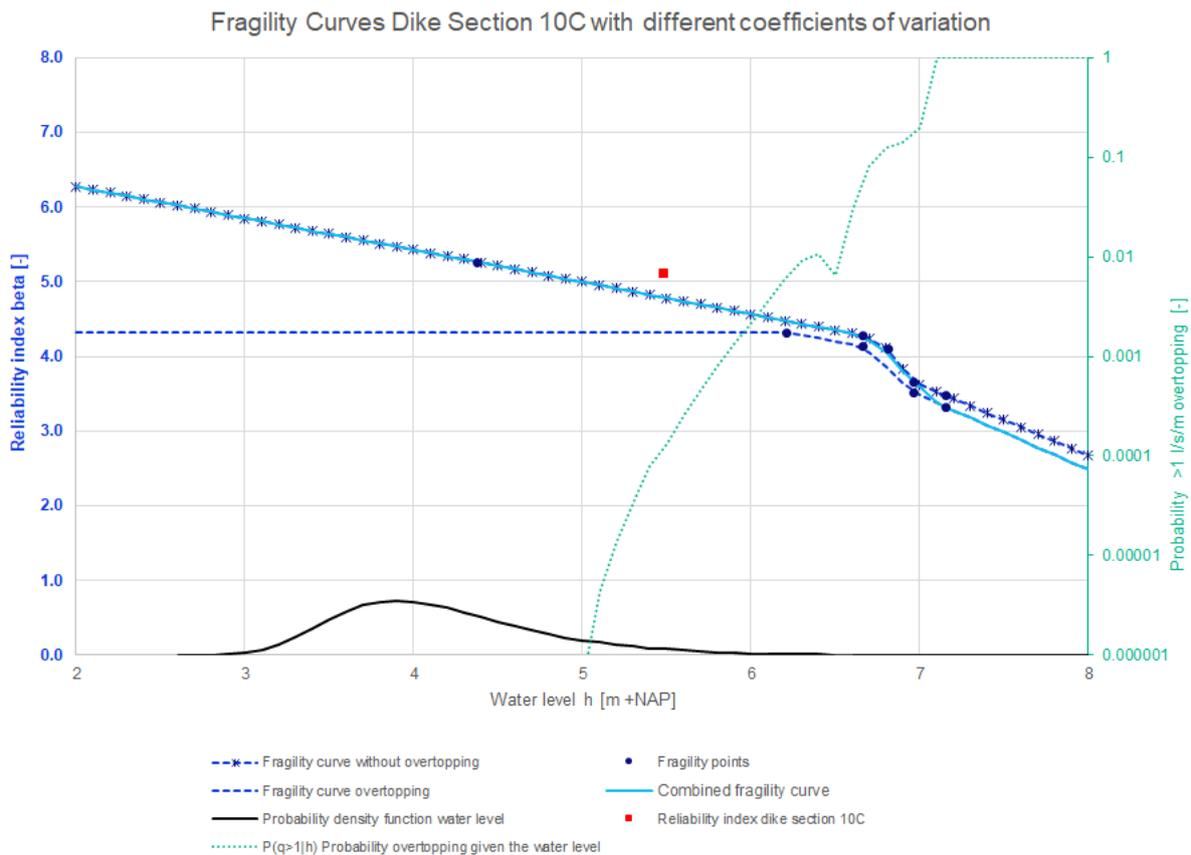
Figure 121: Fragility curves dike section 10C with different coefficients of variation
