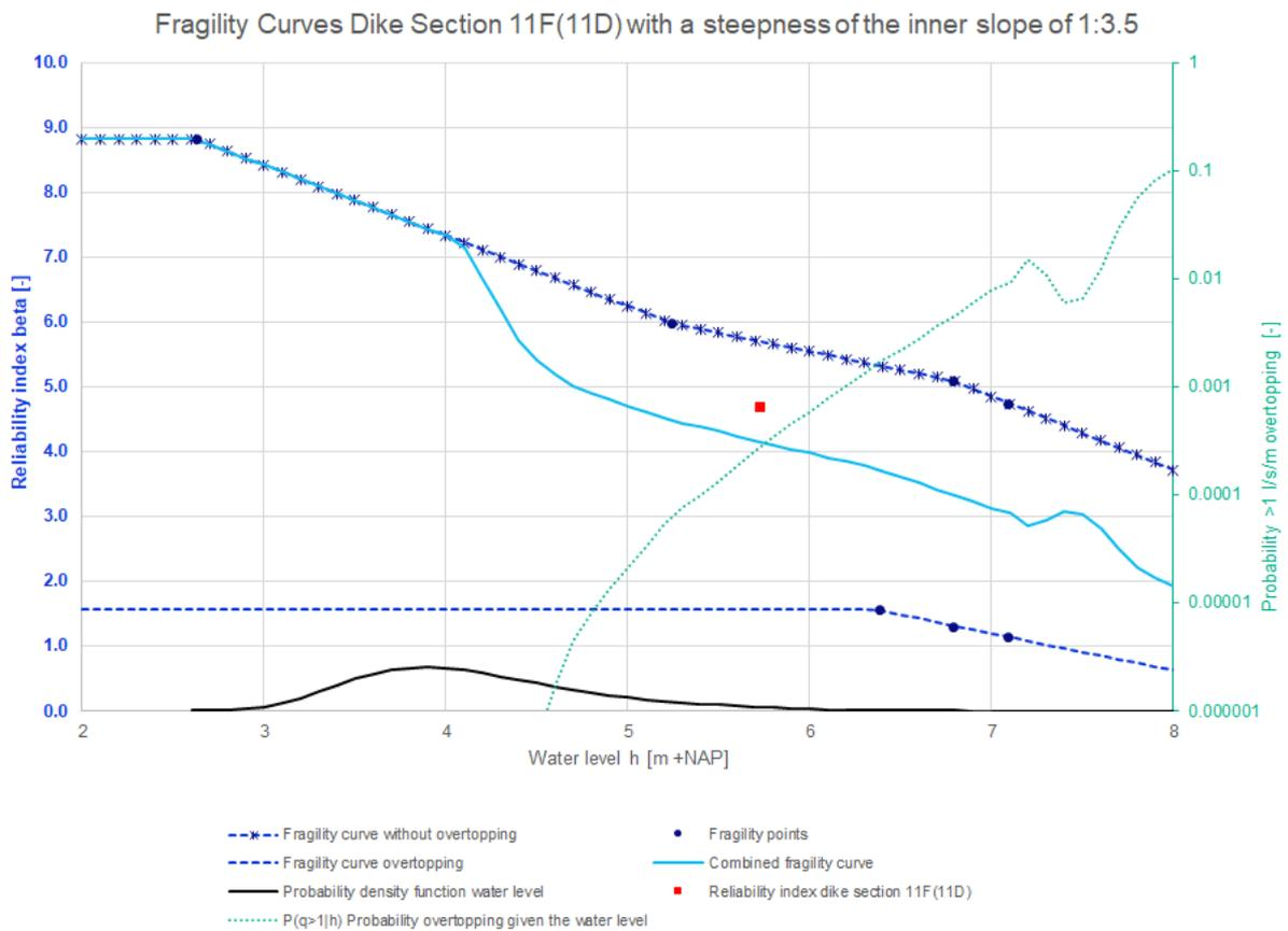
Figure 93: Fragility curves dike section 11F(11D) with a steepness of the inner slope of 1:3.5
