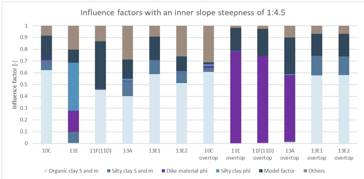
Figure 114: Influence factors with an inner slope steepness of 1:4.5 at WBN without overtopping and at the 1 l/s/m overtopping water level with overtopping
