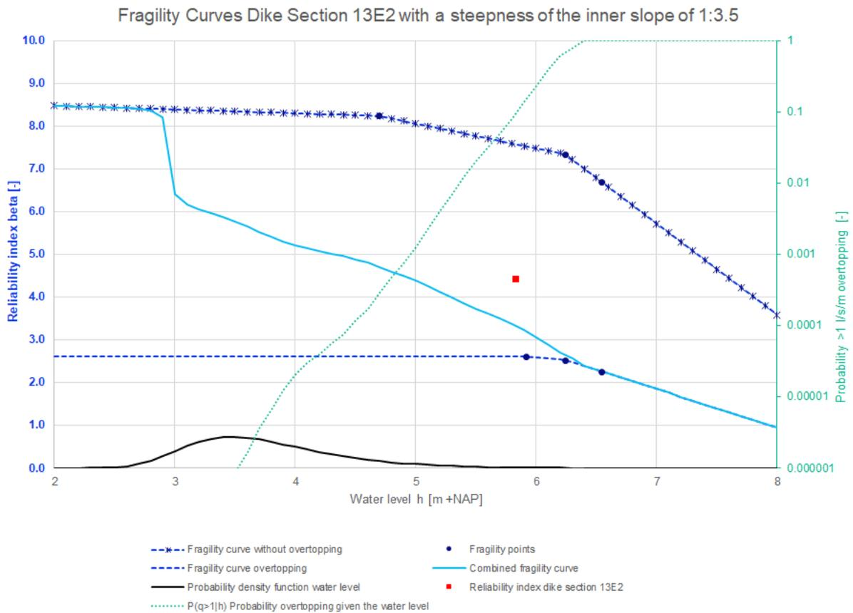
Figure 96: Fragility curves dike section 13E2 with a steepness of the inner slope of 1:3.5
