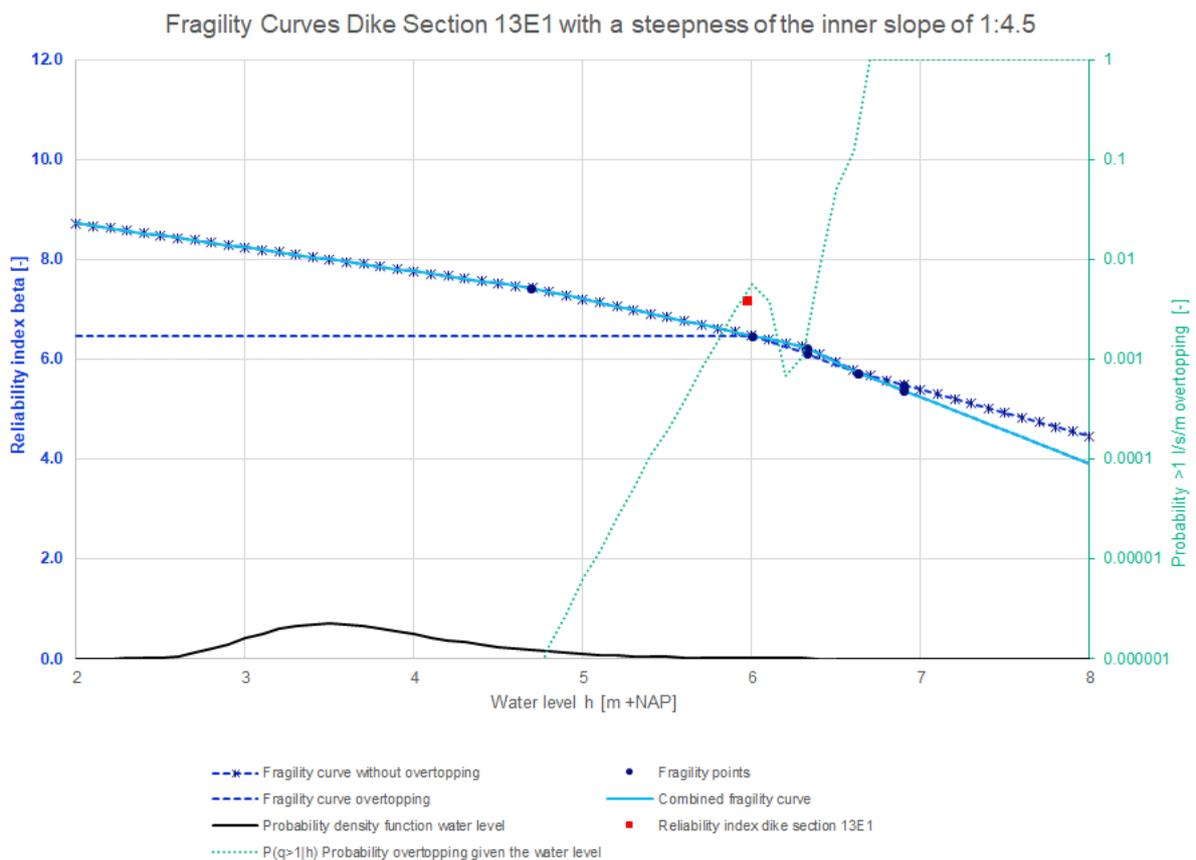
Figure 111: Fragility curves dike section 13E1 with a steepness of the inner slope of 1:4.5
