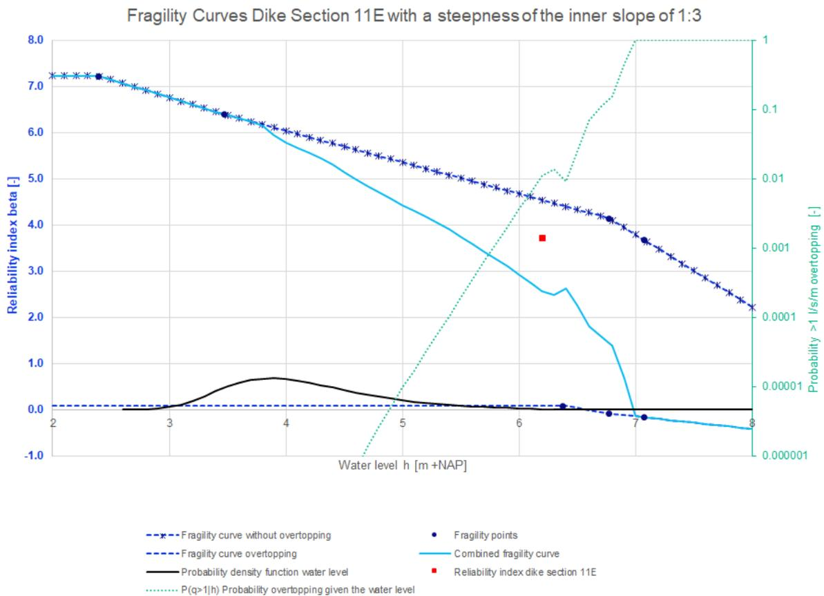
Figure 86: Fragility curves dike section 11E with a steepness of the inner slope of 1:3
