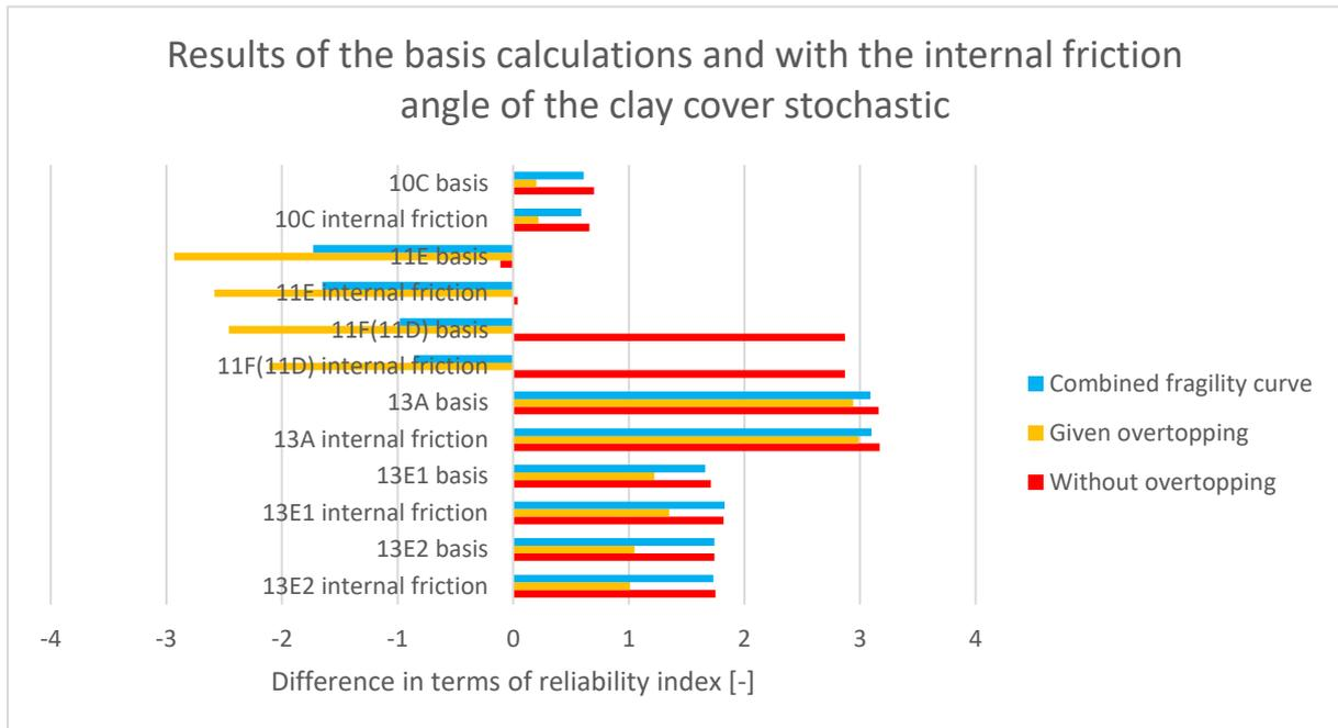
Figure 23: The results of the basis calculations of JAV and with the internal friction angle of the clay cover stochastic compared with the calibration study of WBI. The semi-probabilistic results without overtopping are used to determine the difference in terms of reliability index for the combined fragility curves
