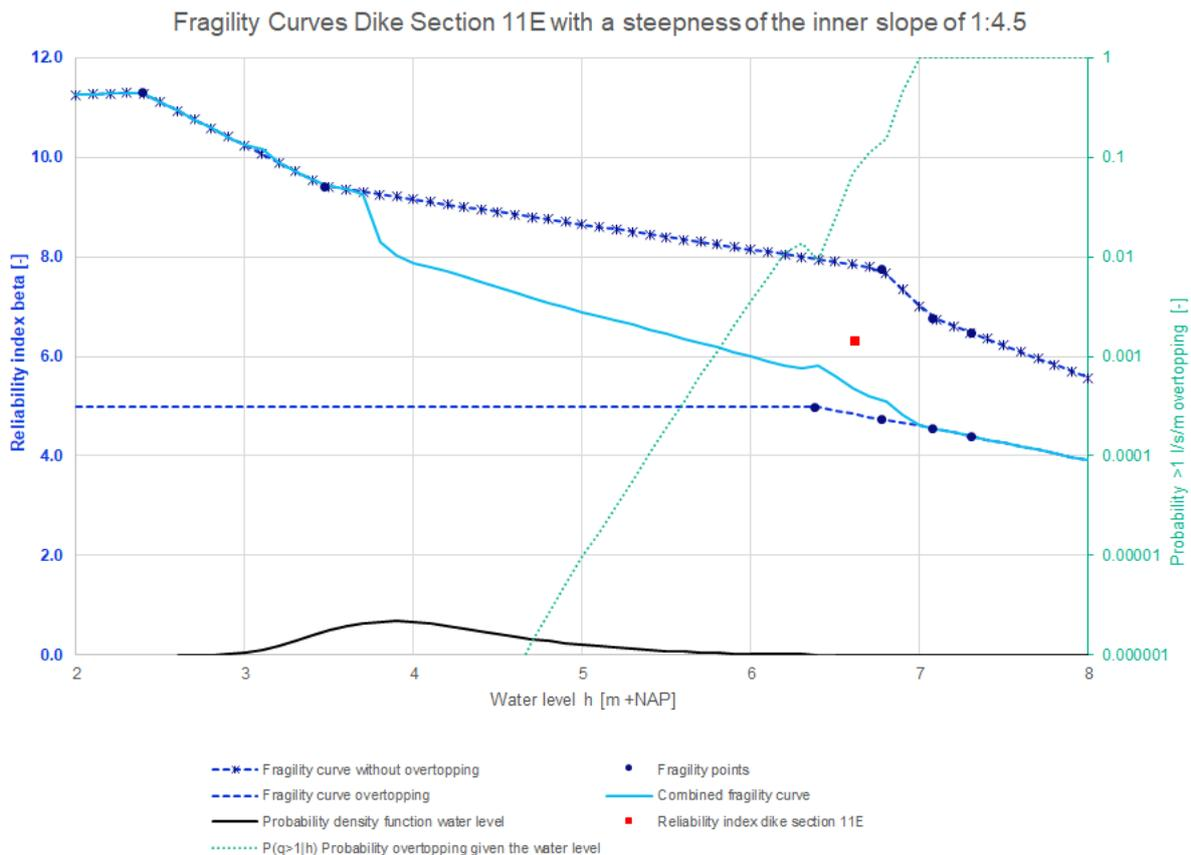
Figure 108: Fragility curves dike section 11E with a steepness of the inner slope of 1:4.5
