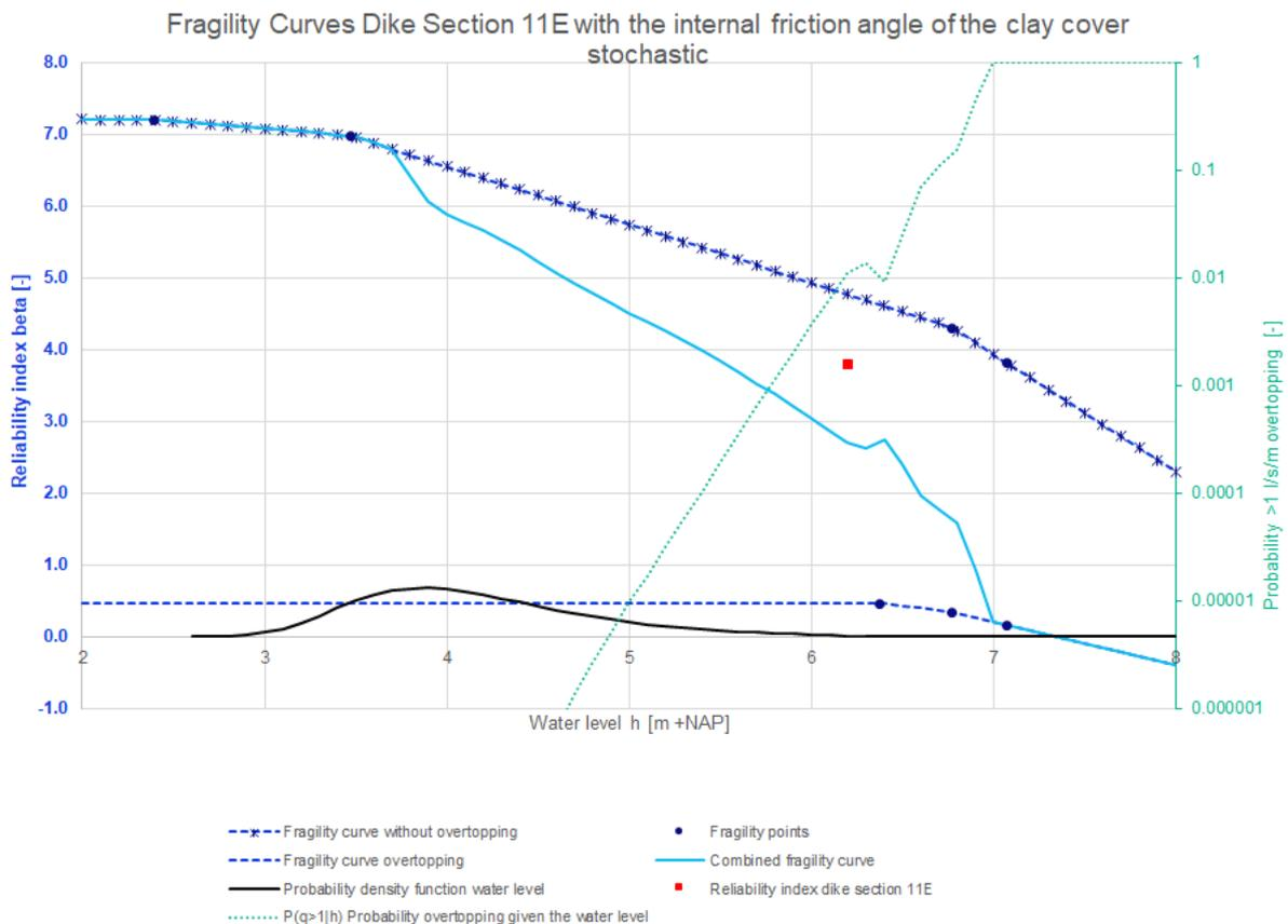
Figure 51: Fragility curves dike section 11E with the internal friction angle of the clay cover stochastic
