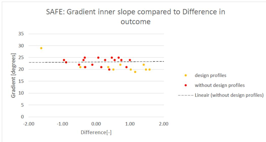
Figure 30: Effect gradient of the inner slope on the difference in reliability index without overtopping for SAFE (Prins, 2021)
