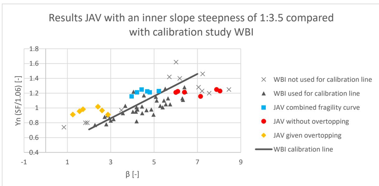
Figure 97: The results of the calculations of JAV with an inner slope steepness of 1:3.5 compared with the calibration study of WBI. The vertical position of the results of JAV from the combined fragility curves (blue squares) are determined based on the semi-probabilistic results without overtopping
