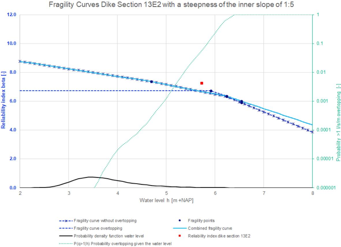
Figure 120: Fragility curves dike section 13E2 with a steepness of the inner slope of 1:5
