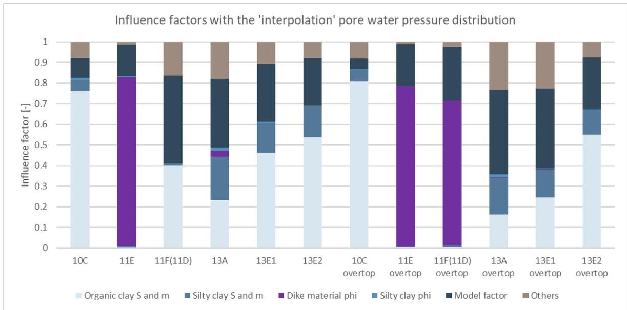
Figure 78: Influence factors with the 'interpolation' pore water pressure distribution at WBN without overtopping and at the 1 l/s/m overtopping water level with overtopping
