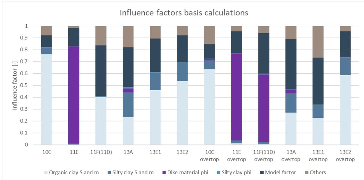
Figure 20: Influence factors basis calculations at WBN without overtopping and at the 1 l/s/m overtopping water level with overtopping
