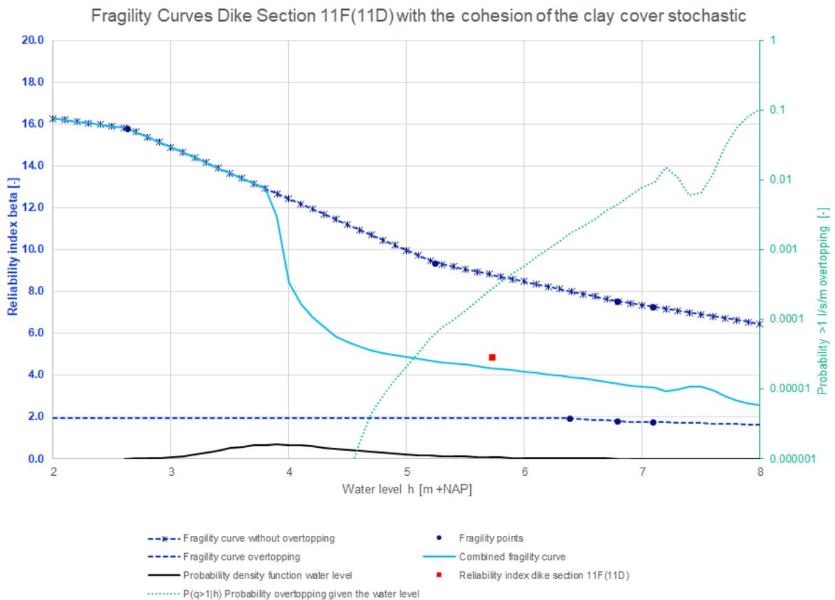
Figure 44: Fragility curves dike section 11F(11D) with the cohesion of the clay cover stochastic
