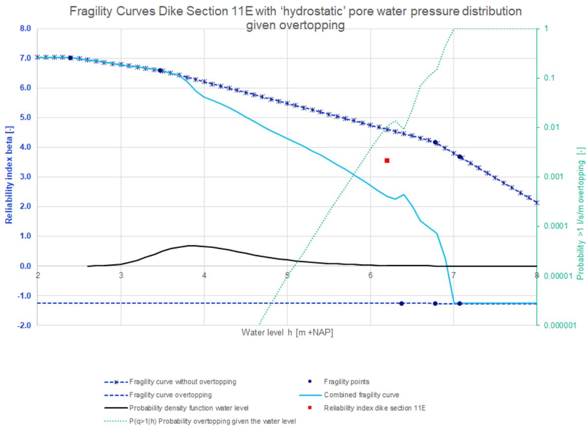
Figure 66: Fragility curves dike section 11E with 'hydrostatic' pore water pressure distribution given overtopping
