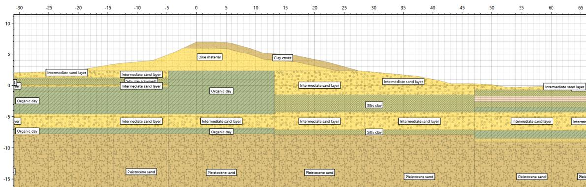
Figure 13: Schematization of dike section 13A
