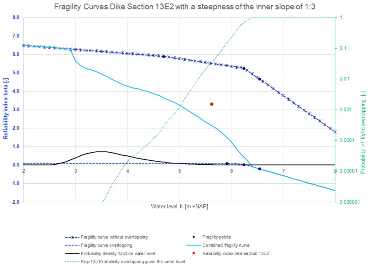
Figure 90: Fragility curves dike section 13E2 with a steepness of the inner slope of 1:3
