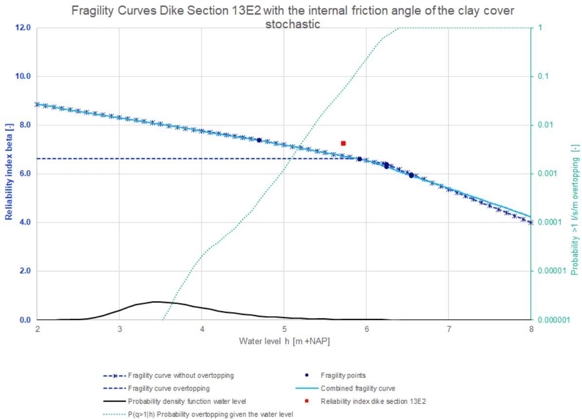
Figure 55: Fragility curves dike section 13E2 with the internal friction angle of the clay cover stochastic
