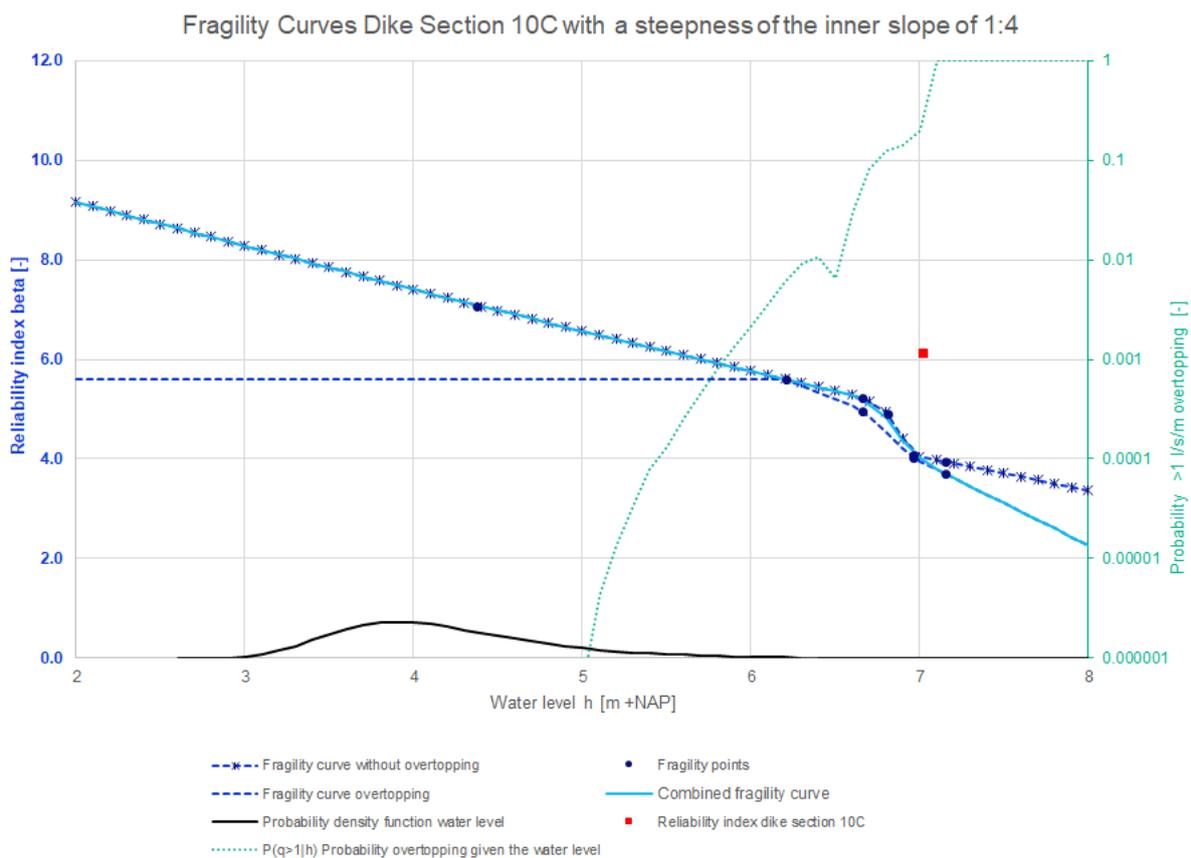
Figure 99: Fragility curves dike section 10C with a steepness of the inner slope of 1:4
