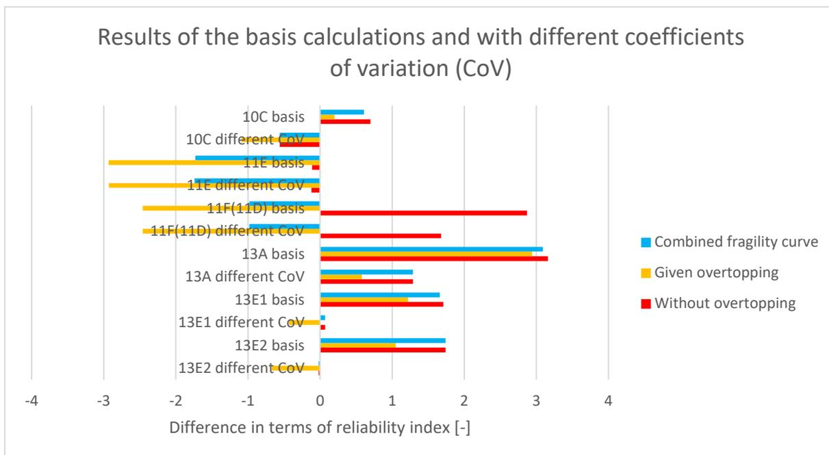
Figure 35: The results of the basis calculations of JAV and with different coefficients of variation compared with the calibration study of WBI. The semi-probabilistic results without overtopping are used to determine the difference in terms of reliability index for the combined fragility curves
