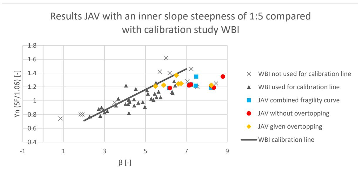
Figure 27: The results of the calculations of JAV with an inner slope steepness of 1:5 compared with the calibration study of WBI. The vertical position of the results of JAV from the combined fragility curves (blue squares) are determined based on the semi-probabilistic results without overtopping
