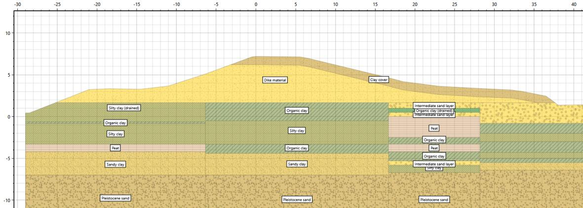
Figure 10: Schematization of dike section 10C
