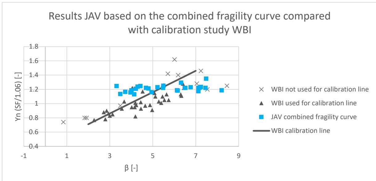
Figure 32: The results of the calculations of JAV based on the combined fragility curves with different slopes compared with the calibration study of WBI. The vertical position of the results of JAV from the combined fragility curves (blue squares) are determined based on the semi-probabilistic results without overtopping
