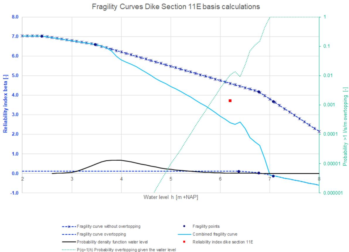
Figure 37: Fragility curves dike section 11E basis calculations
