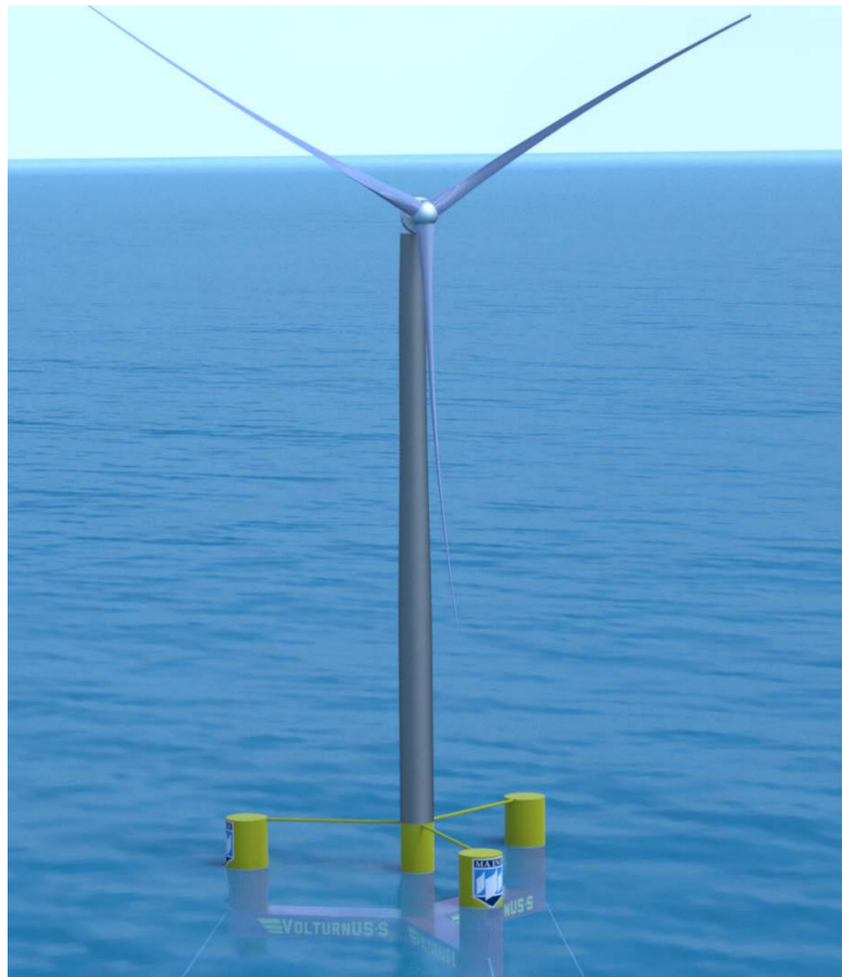
Figure 6.12: The UMaine VoltturnUS-S Reference Platform Designed to Support the IEA-15-240 OWT System Definition. [2]
