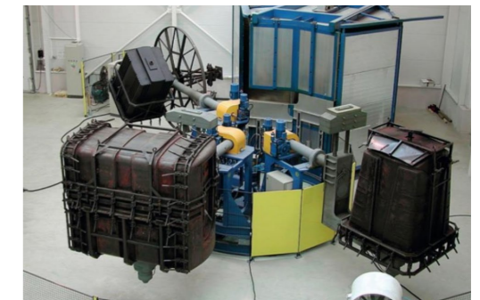
Figure 27: Rotomoulding Source: Elkoplast
