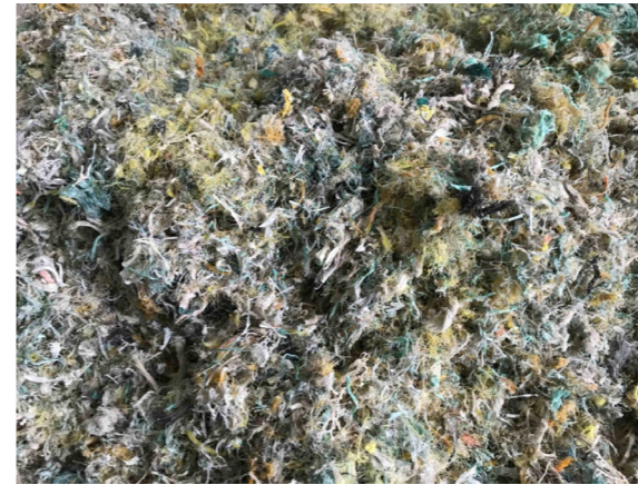
Figure 15: Ocean plastic fluff from fibrous fraction Source: The Ocean Cleanup recycling research
