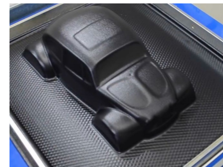
Figure 26: Vacuum forming Source: Formechs
