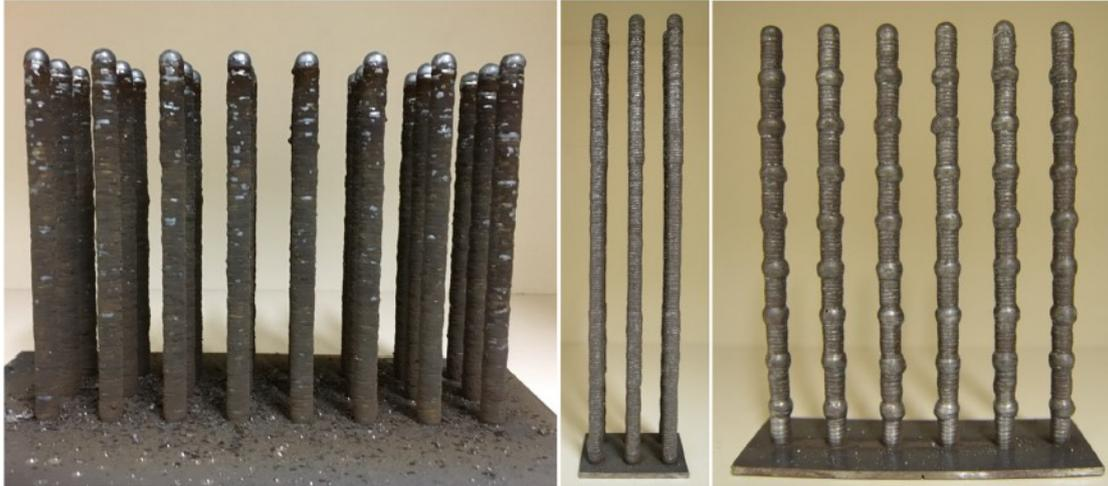
Figure 2.7: Normal(left), improved (middle) and extra profiled (right) additive manufactured steel bars for concrete reinforcement. Taken from Mechtcherine, Grafe, Nerella et al.<sup>[24]</sup>.
