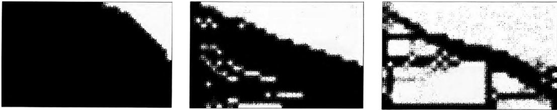
Figure 3.1: Optimisation of a rectangular modelling space. Black areas indicate material, white areas are voids. Taken from Bendsoe and Kikuchi<sup>[25]</sup>
