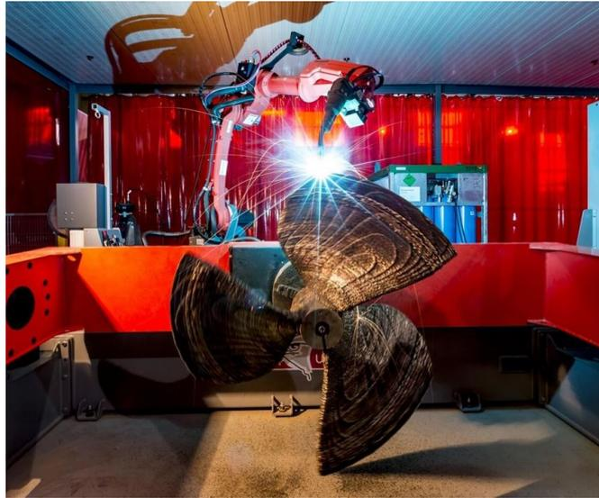
Figure 2.3: Fabrication of a ship's propeller using the WAAM technique
