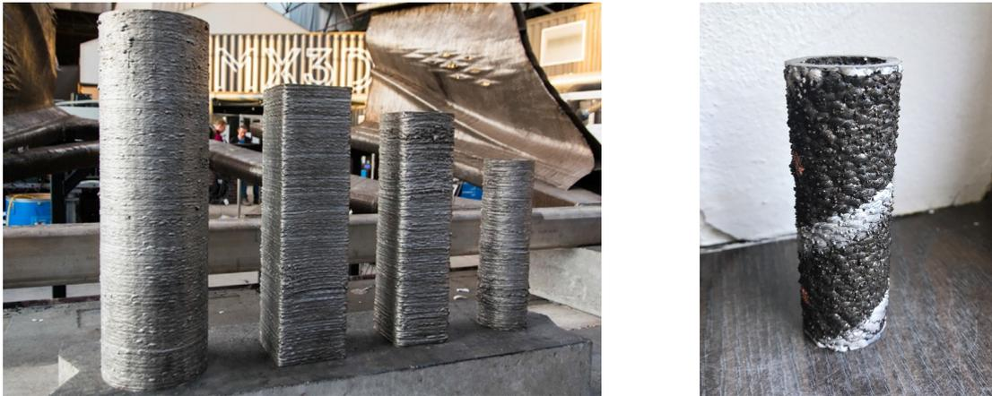
Figure 2.4: Surface finish for continuous(left) compared to dot-by-dot(right) strategy
