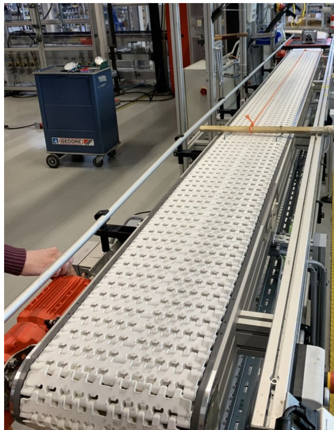
Figure B.1: Stress-Strain curve experiment for the UNI Flex One chain belt
