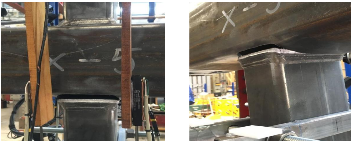
Figure F-3 Failure mode of XS700 \beta 0.857
