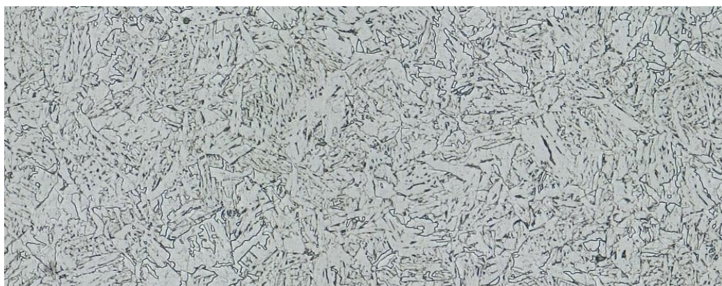
Figure B-8 Microscopy image of the CGHAZ of S355 sample
