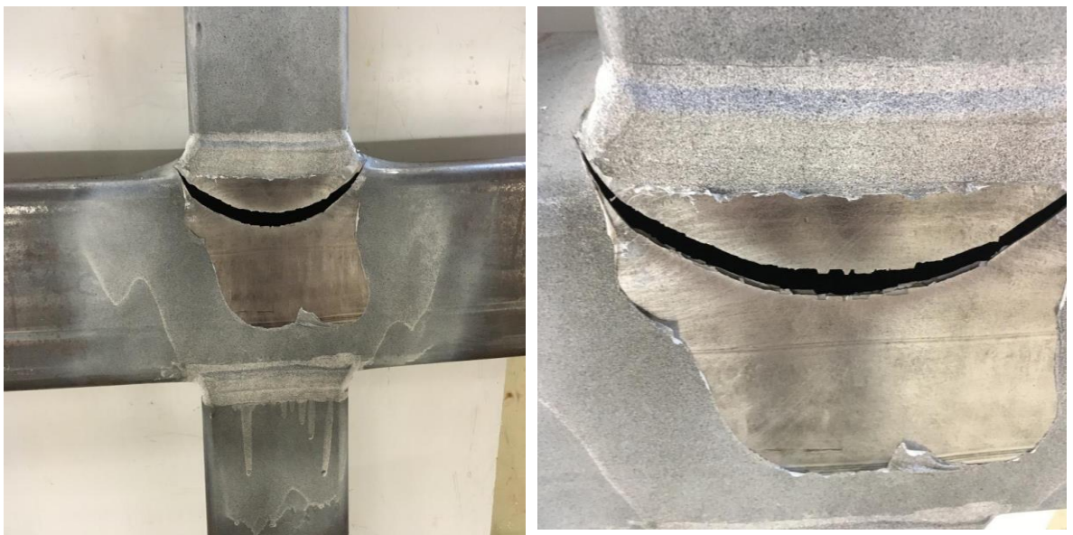
Figure F-5 Failure mode of XS355 \beta 1.0
