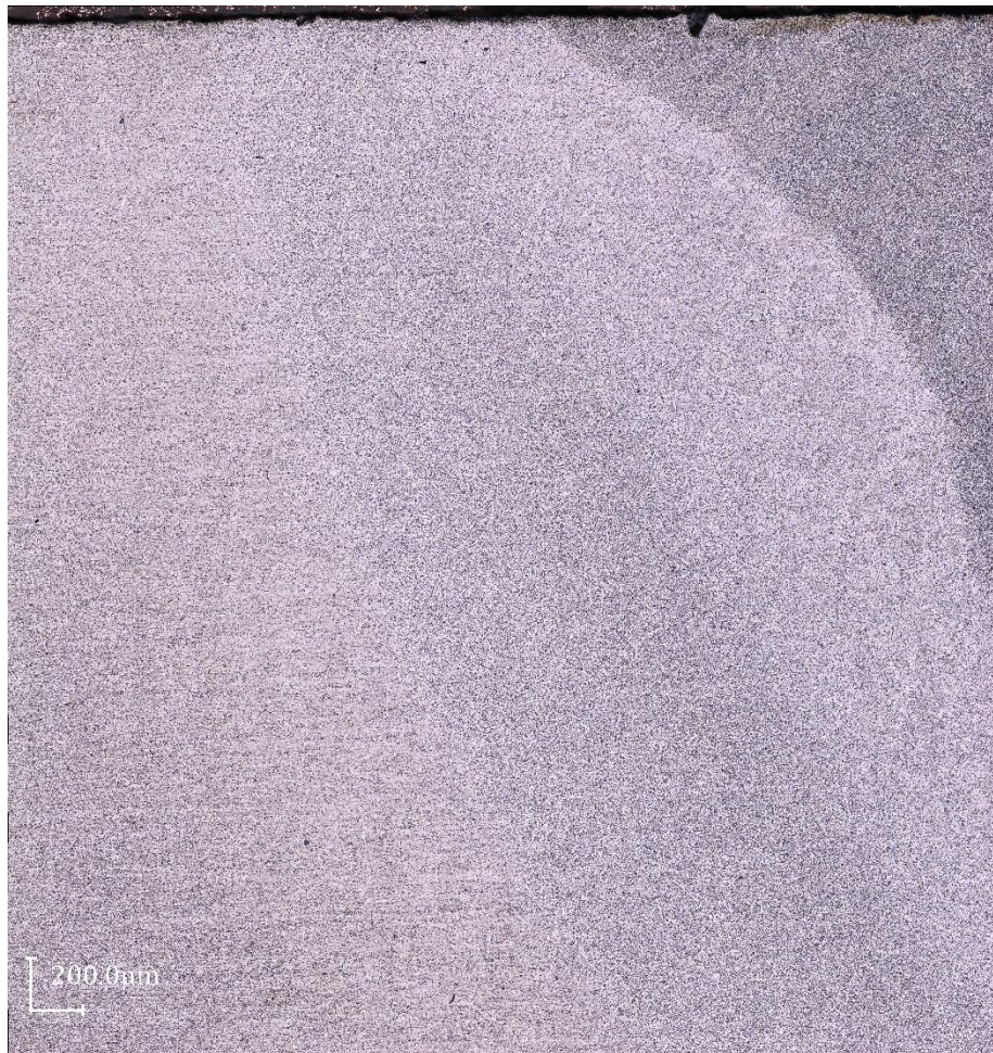
Figure B-1 The microstructure of weld zone of the S700 sample
