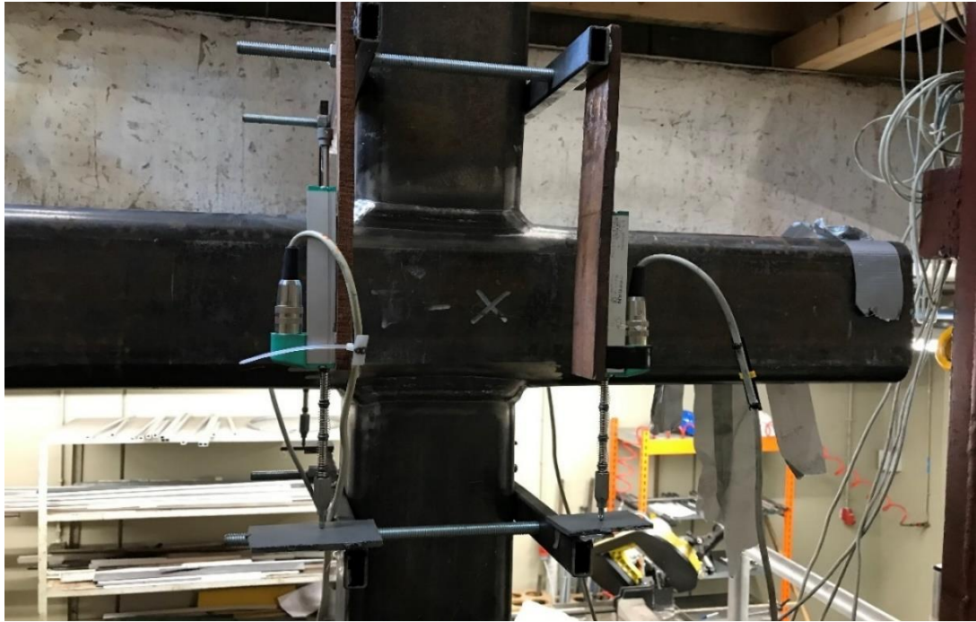
Figure 5-3 Assembled steel frame onto the top and bottom of the braces with four LVDTs
