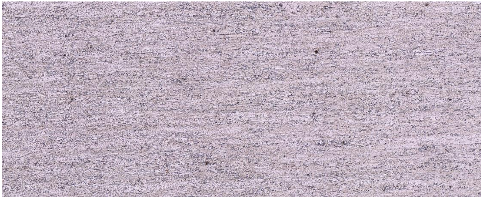
Figure B-5 Microscopy image of the base material of S700 sample
