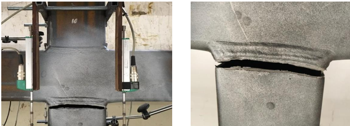
Figure F-2 Failure mode of XS500 \beta 1.0
