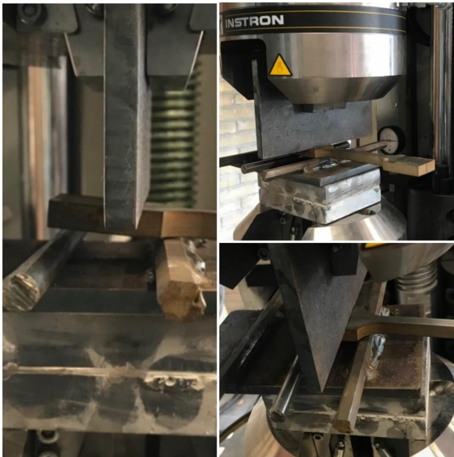
Figure 3-4 Flattening of the grip sections
