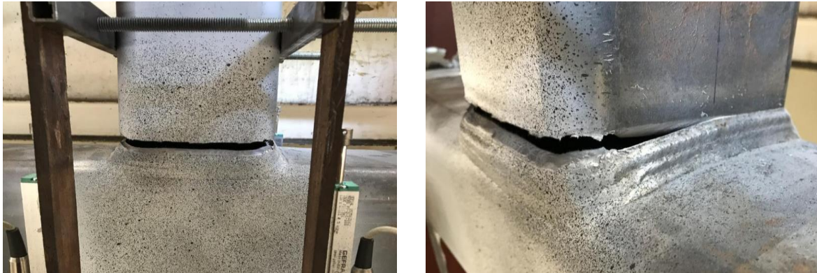
Figure F-1 Failure mode of XS500 \beta 0.875
