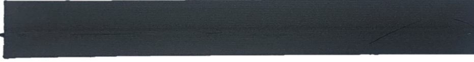
Figure 4.9: A 3D-printed TPU CF sample used for measuring the mechanical properties with a tensile test. This particular sample has a UD material orientation of 0^\circ .
