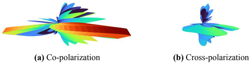
**Figure 3.14:** 3D subarray antenna pattern of benchmark HBF
