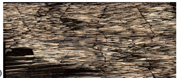
Fig. 4.17. Compressive behaviour of [\pm 27_7/0]_S MR60/M55J carbon layup, a) Pseudo-ductile stress–strain response and b) compressive ply fragmentation in the central 0^\circ plies [178].
