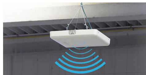
Figure B-6: RFID overhead reader - source: Expo 21xx
