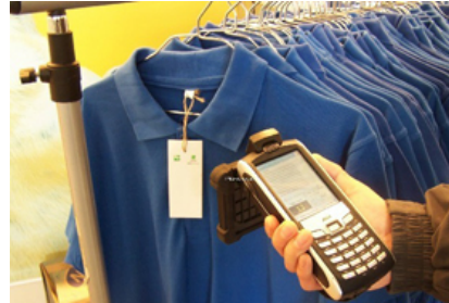
Figure B-2: RFID handheld reader - source: J&J Cooperated
