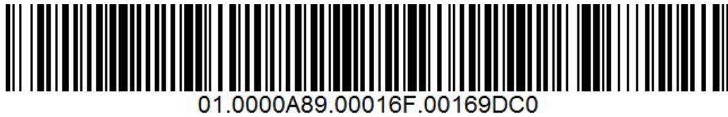
Figure 2-7: The EPC in a regular barcode - source: TEC-IT
