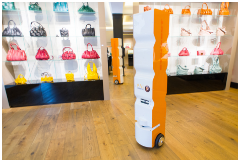
Figure B-3: RFID robot reader - source: Pal robotics
