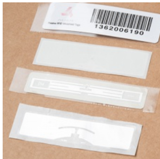
Figure 2-10: Passive RFID tags - source: Sparkfun
