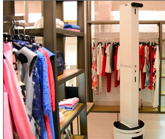
Figure 2-12: An RFID-tag reading robot - source: RFID journal
