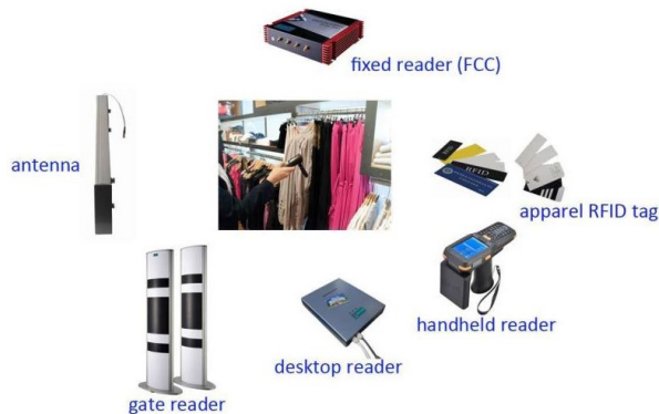
Figure 2-11: Multiple RFID readers used in the apparel industry - source: Vance
