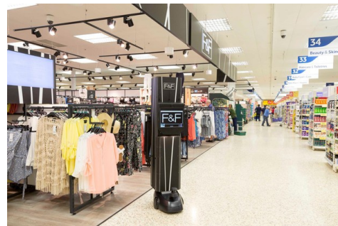
Figure B-4: RFID robot reader - source: RFspot
