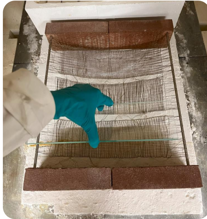
2. Use of bricks & stainless steel bars to set-up the basalt moulds and then place glasses on top
