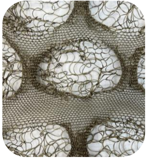
CNC knitted mould
