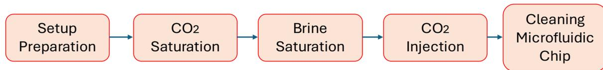
*Figure 3-8 Flowchart of the steps taken during the salt dry-out experiment.*
