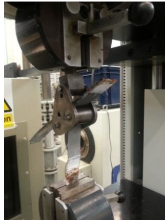
Figure 2: Floating roller peel test set up
