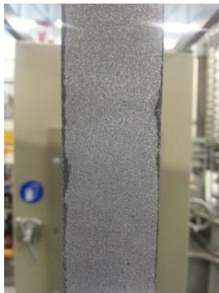
Figure 5: Fractured specimen after peel test
