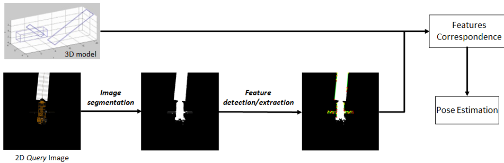
Figure 1. Generic schematic of a feature detection/extraction flow.
