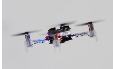
Fig. 9. Crazyflie, a 39-gram MAV from company Bitcraze.
