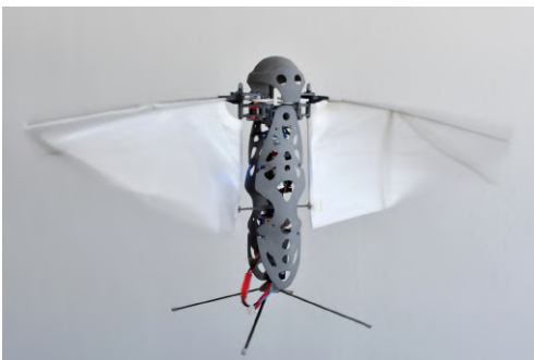
Fig. 8. Flapper, a 100-gram bio-inspired flapping-wing MAV from company Flapper Drones.
