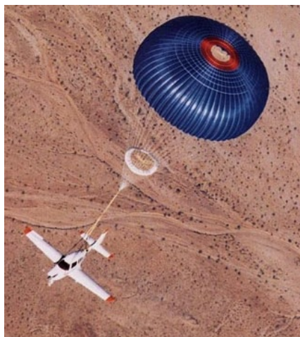
Figure 4.2: Cirrus SR20 Ballistic Parachute
