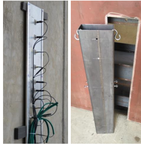
Figure 3. Pressure array (left) and hollow force measurement section (right) before implementation into steel wall
