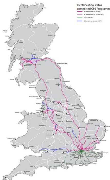
Figure 18 – Electrification of the GB main line network
