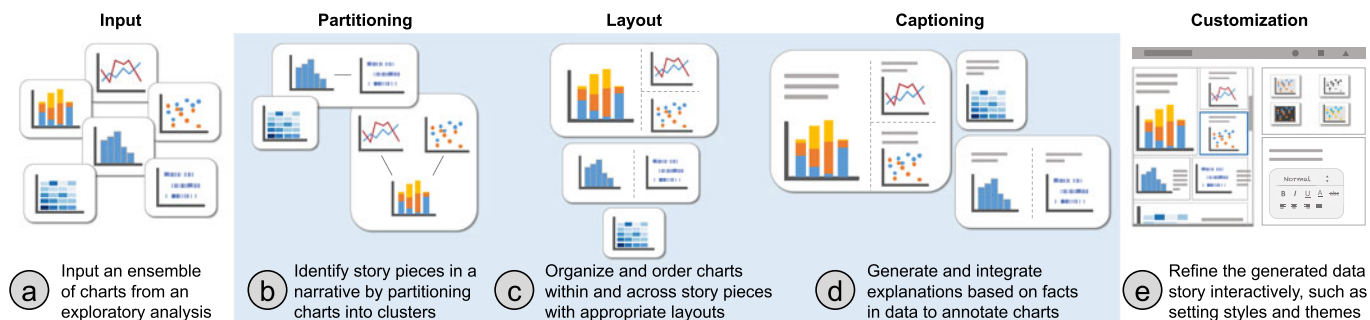
Fig. 1. ChartStory takes an ensemble of user-created charts (a) and automatically generates a data comic (b-d). This is achieved through a back-end pipeline with operations to identify story pieces (b), organize & order story pieces (c), and generate & integrate explanations (d). The user can also interactively edit the captions and layout of the charts, and change the style or appearance of the data comic (e).
