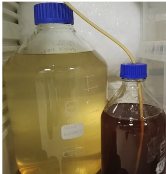
Figure O.1: Colour change of the AnMBR feed solution over after one week.
