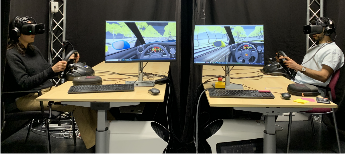
Figure 3: Experimental setup. Two participants taking part in the experiment each with a steering wheel, pedals and VR headsets
