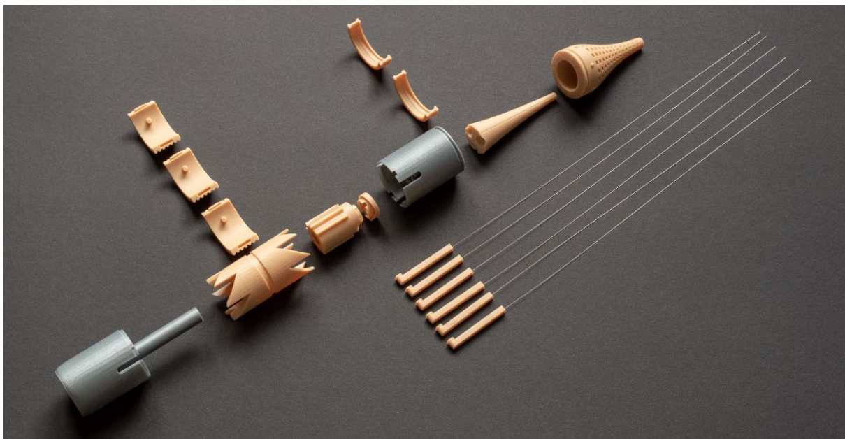
Fig. 19. Exploded view of additive manufactured components. The grey parts, i.e., the housing components, were produced using the fused deposition technology (FDM) technology in polylactic acid (PLA) on the Ultimaker 3. The orange parts, i.e., the actuation and steering unit's internal components and the double cone, were produced using the stereolithography (SLA) technology in Dental Model resin V2 (Formlabs) on the Formlabs Form 3B.
