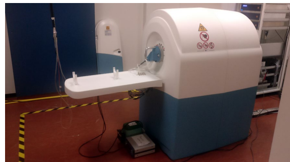
Fig. 20. Photograph of the preclinical 7-T MRI system (MR Solutions Ltd) used in the MR compatibility and ex vivo tests executed in this study. The MRI system is located at the Amsterdam University Medical Centres.
