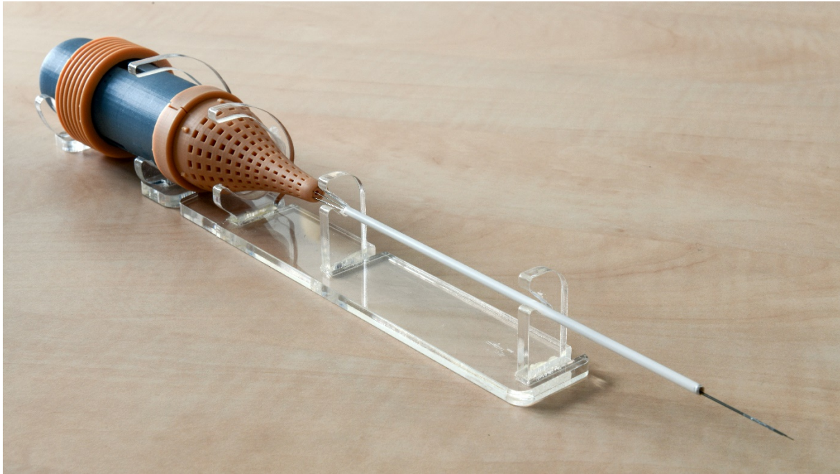
Fig. 23. Photograph of the assembled prototype, the Ovipositor MRI-Needle. A transparent polymethyl methacrylate (PMMA) support structure supports the prototype. A white polylactic acid (PLA) guide tube supports the needle in the support structure.
