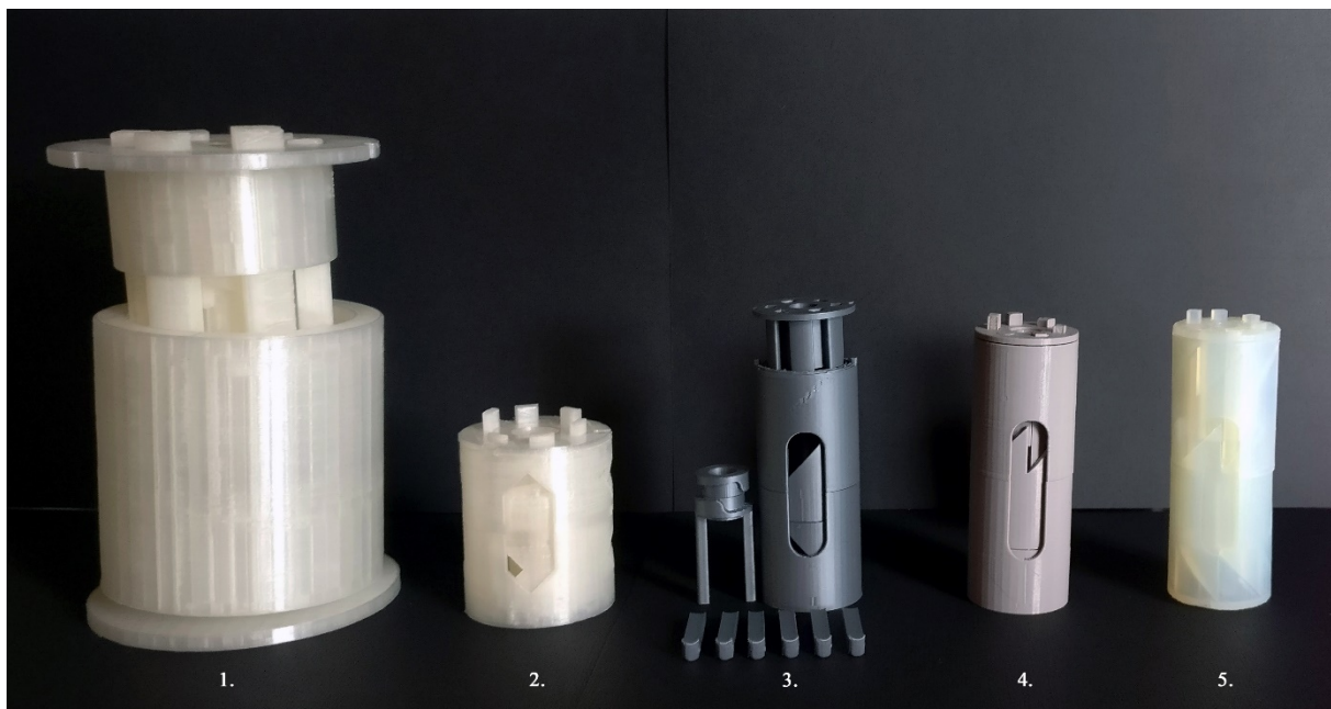
Fig. E-11. Photograph of the five iterations of the actuation unit using additive manufacturing. Prototype 1 and prototype 2 were FDM printed in PLA using the Ultimaker 2. Prototype 3, and prototype 4 are FDM printed in polyethylene terephthalate glycol (PETG) using the Prusa. Prototype 5 is SLA printed in Durable Resin using the Formlabs 3B.
