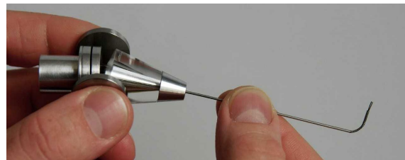
Fig. 10. Photograph of the I-Flex, a steerable surgical instrument prototype that applies a global steering mechanism to steer the tip of the instrument. Adapted with permission from [59].
