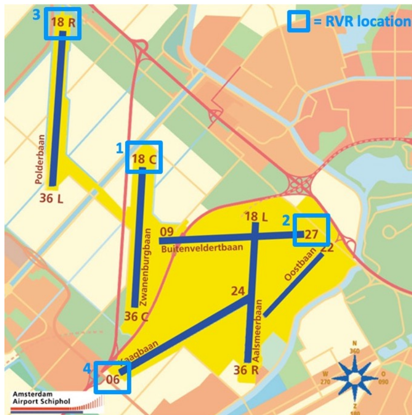
Figure 3.12: Locations of the four RVR observations at Schiphol airport visible as blue boxes around the measuring locations. The numbers next to the boxes correspond to location names used in this research
