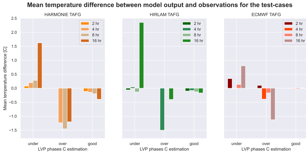
Figure 4.18: Mean temperature difference between TAFG and observations for the test cases. The panels represent the TAFG output for the three input NWP models. The x-axis are the type of estimation for the LVP phase C. The y-axis represent the difference between the modelled and observed temperature. The results are obtained for all four lead times as indicated in the legend.
