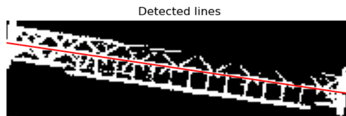
Figure 4.28: Detected line by a Hough transform. The angle of the detected line is the orientation of the gantry in the horizontal plane.
