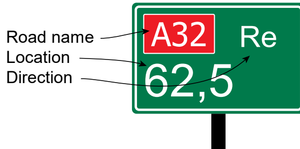
Figure 4.45: A hectometer sign. The signs are placed every 100 meters along the highways. 'Re' stands for right and 'Li' stands for left.
