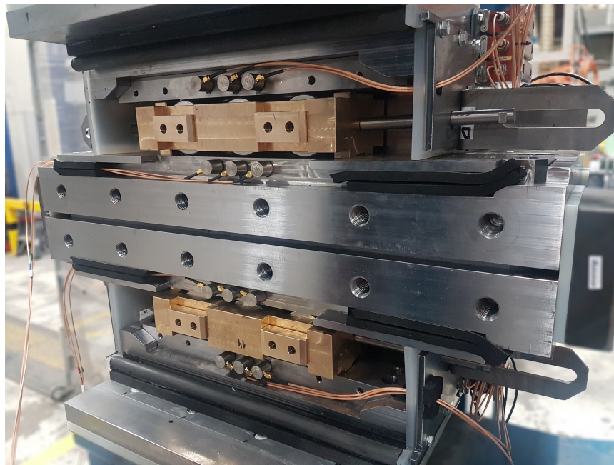
Figure 3.4: Picture of turret bearing test set-up with cover plates removed.
