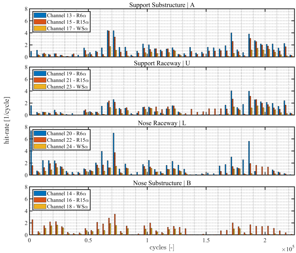
Figure 3.5: Ultrasonic activity in the top chamber separated in graphs per location: support substructure (top), support raceway (upper-middle), nose raceway (lower-middle), and nose substructure (bottom).
