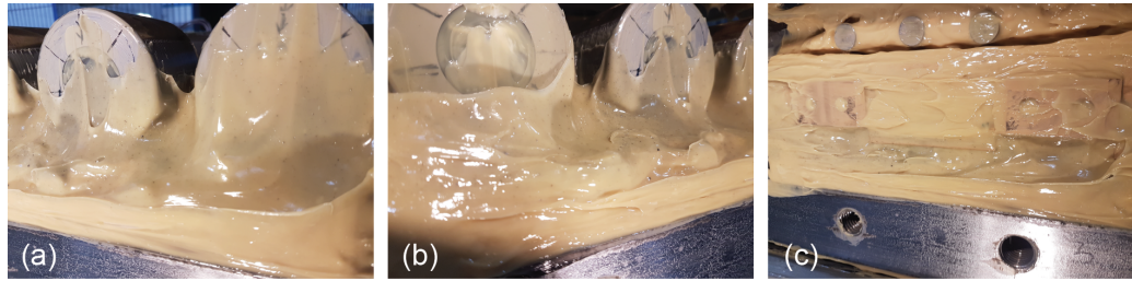
Figure B.3: Inspection of contaminated lubrication after the sample (iii) test, showing; (a–b) The noticeable contamination in the lubrication around the rollers, and (c) around (primarily the bottom of) the cage.
