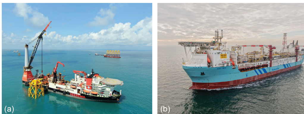
Figure 1.1: Typical examples of highly-loaded low-speed roller bearings in the offshore industry; (a) the offshore mast crane on deepwater construction vessel “Aegir” containing a slew bearing to yaw the boom and sheave bearings to guide the hoisting wire ropes, and (b) the single point mooring turret of “Aoka Mizu” FPSO containing a toothless slew bearing to allow for rotation of the vessel around the seafloor-fixed mooring chains. Courtesy of (a) Heerema Marine Contractors, and (b) Bluewater Energy Services.
