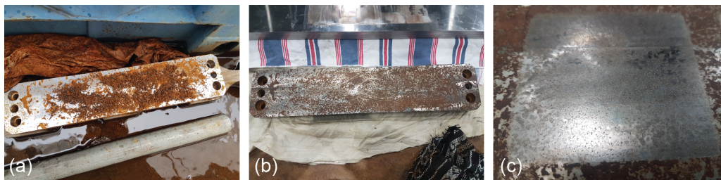
Figure B.7: Several stages of the corrosion test raceway, showing; (a) Initiation of the corrosion process, (b) the corrosion coverage prior to testing, and (c) the resulting abrasion of corrosion in the contact area after the test.
