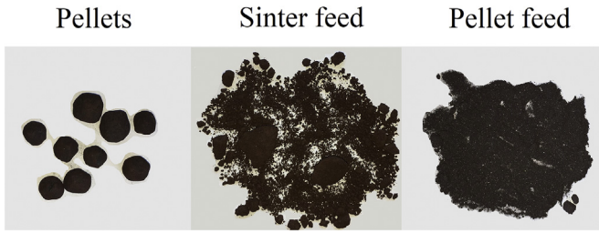
Fig. 3. Various size range in iron ore products; pellets, sinter feed and pellet feed [19].
