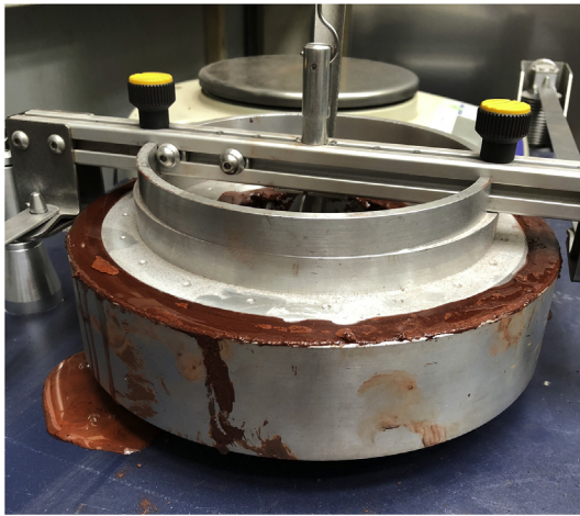
Fig. 16. Excessive water leaving the sinter feed sample in the wet test condition ( MC_{as,rec+4\%} ).
