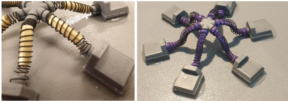
Fig. 10 Hoses are included to prevent the springs from hooking in between the spring windings. (A) rigid bamboo straws (B) stretchable balloons
