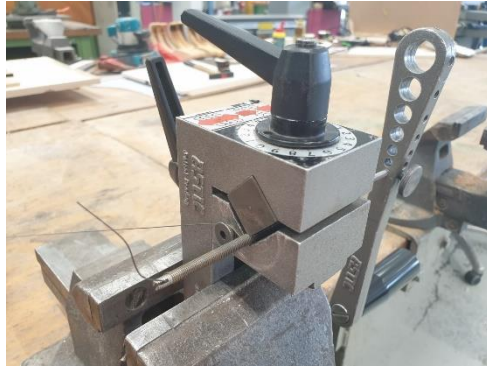
Fig. 2 The springs are wound manually with a spring winder.
