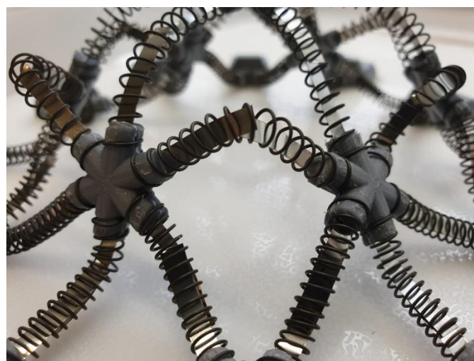
Fig. 9 The flexures hook in-between the spring windings, making it difficult to push the mechanism back in plane.
