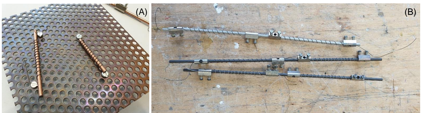
Fig. 1 (A) Method 1: winding wire around rod and clamping with bolts and nuts on plate. (B) Method 2: winding wire around rod and clamping with terminal blocks. This method is chosen and improved.
