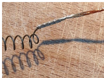
Fig. 21 SMA spring crimped with tinned Litz wire to ensure sufficient electrical connection
