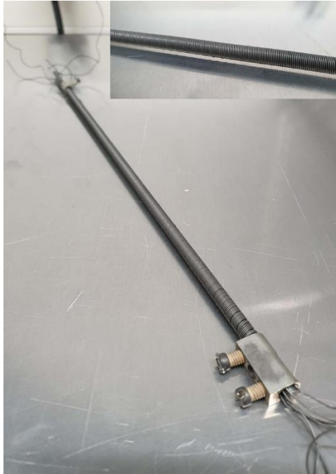
Fig. 3 The pitch angle can be set with the number of windings that are placed on one rod.
