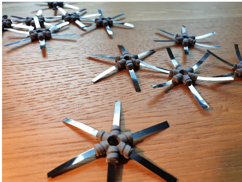
Fig. 7 The resulting connectors with threaded ends to connect the springs and with flexures glued in between to prevent in-plane rotation.
