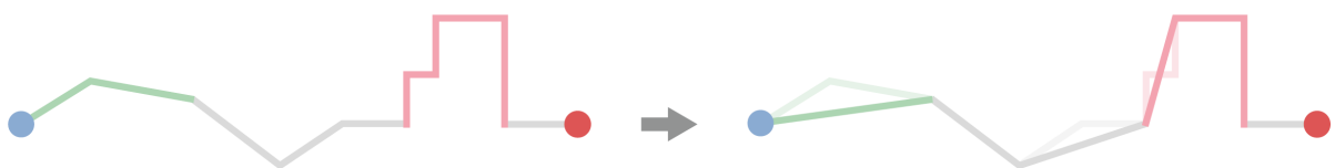
Figure 7.1: Simplification by Douglas-Peucker (Green: Grass, Grey: Road, Pink: Building, Red Dot: Source Point, Blue Dot: Receiver)
