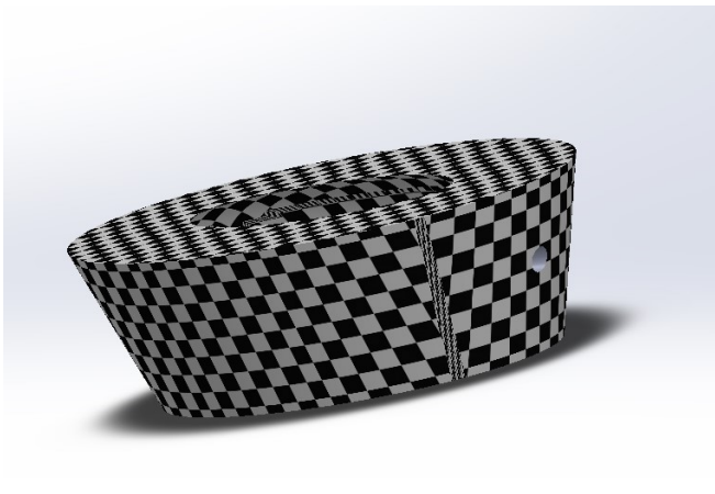
Figure 5.21: Prototype 3 Outside of the rigid ring, a small hole is visible on the right edge to blow air through to inflate the balloon.
