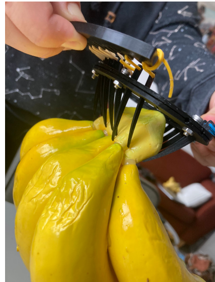
Figure 5.11: Prototype 1.1 Grasping the foam bunch of bananas side view
