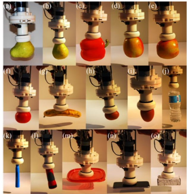
Figure 16: Granular gripper grasping several objects (Krahn, Fabbro, and Menon 2017)
