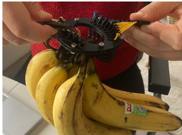
Figure 5.15: Prototype 1.2 Grasping a real bunch of bananas with the second version of the fingers prototype
