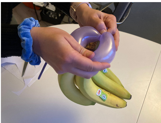
Figure 5.23: Prototype 3 Lifting a real bunch of bananas using an inflated balloon around the tip
