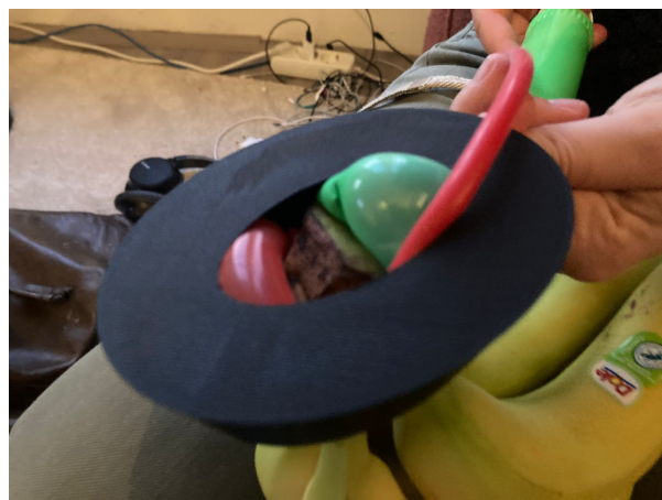
Figure 5.24: Prototype 3 Balloons inflated inside the rigid ring
