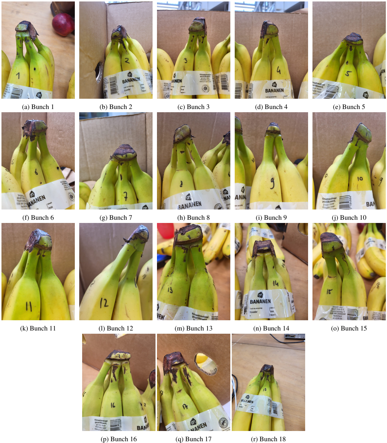
Figure A1: Photos taken of bunches of bananas after picking them up with the gripper. The photos are used for inspection of the damage done by the gripper on the peduncles
