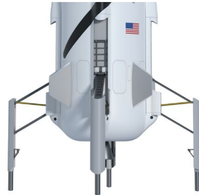
Figure 7.17: Landing legs of the New Shepard launcher 24
