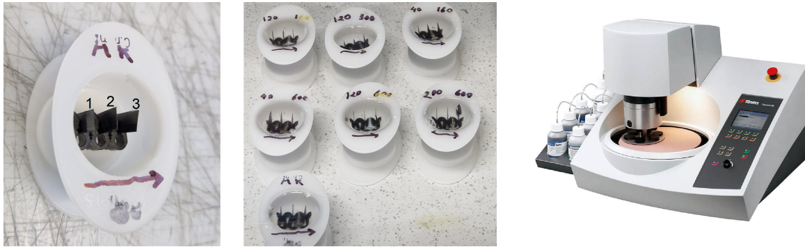
Figure 5.4: Steps for embedding samples, samples placed in moulds, moulds are embedded and the final grinding and polishing step on the Struers Tegramin.
