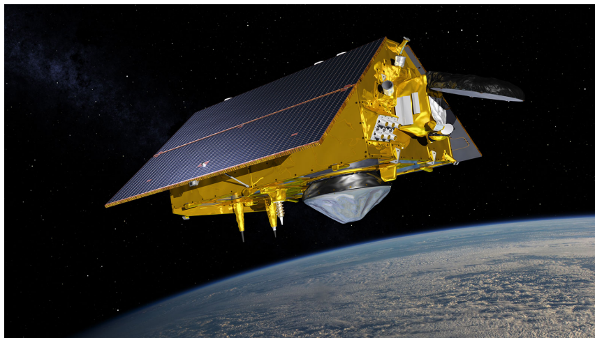
Figure 2.18: The Poseidon-4 altimeter antenna, on the bottom of the satellite. Image Credits: NASA JPL
