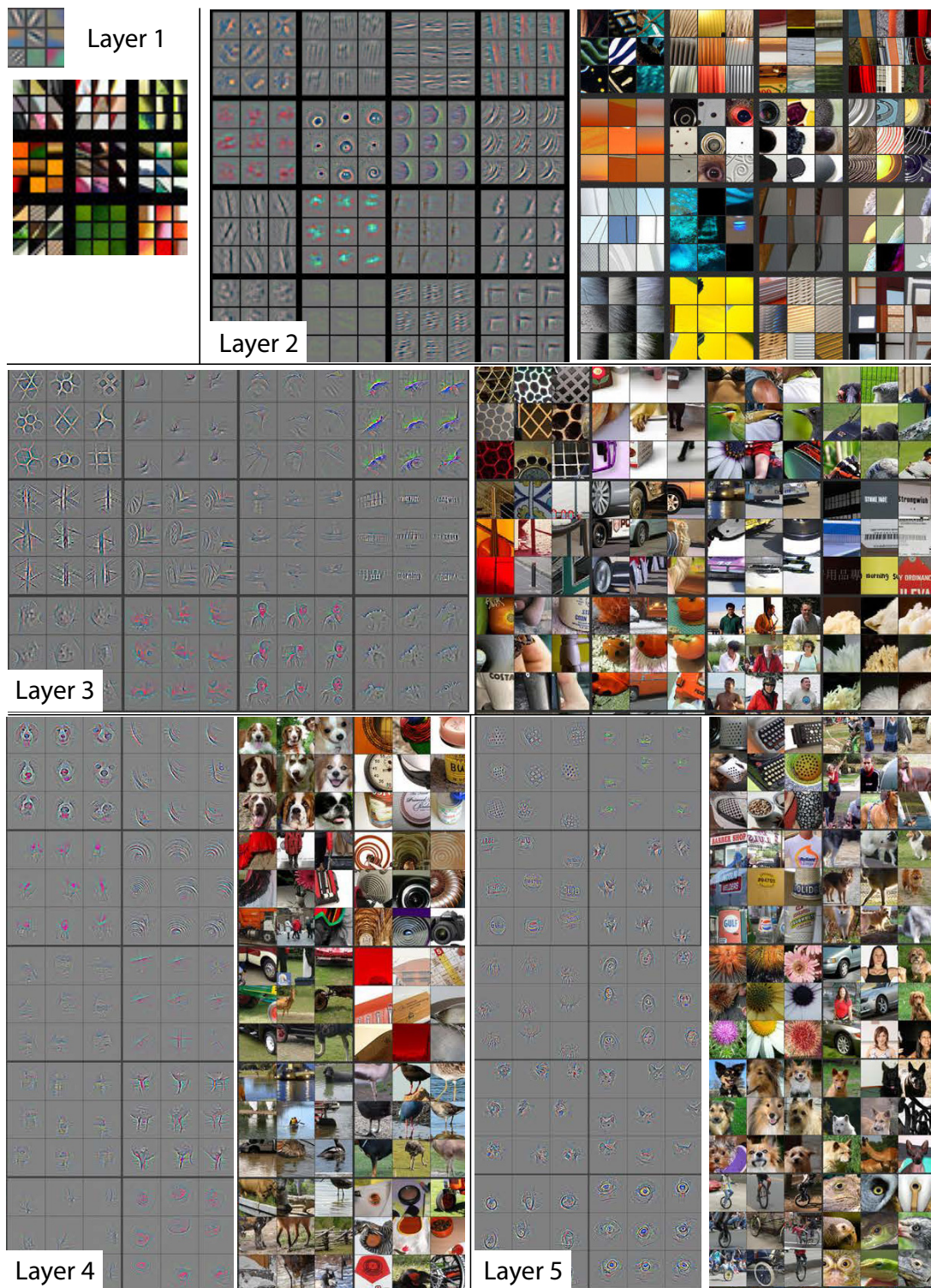
Figure 2.6: Bottom-up hierarchy of a trained network [25]; for each layer the top nine activations, projected to pixel space, for a random subset of feature maps in the validation set are visualized, along with the the corresponding image patches.
