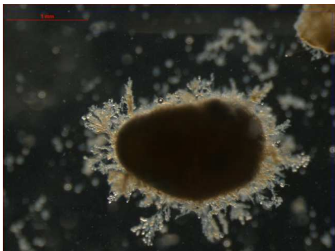
Figure 6-2: Granule from the pilot-scale reactor in Dokhaven, suffering from a protozoa bloom. Scale bar is 1 mm.
