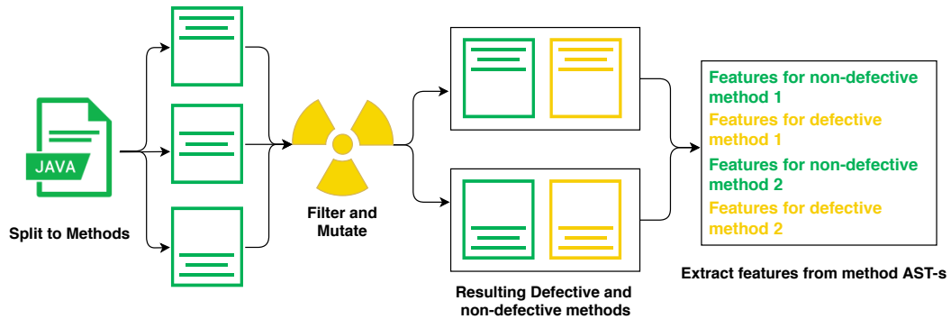
Figure 3.2: The flow of feature extraction for Code2Vec and Code2Seq models.
