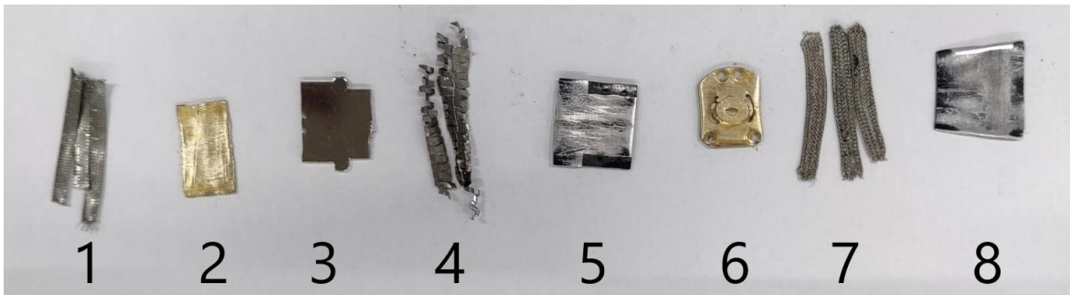
Figure 25: Metal samples of the flexible intubation scopes for identification of the material with X-Ray fluorescence
