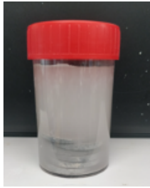
Figure 3.4: Specimen stored in lime solution for exposure.
