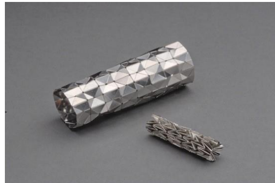
Figure 12: Zhong You's origami heart stent design, in deployed and stowed state.
