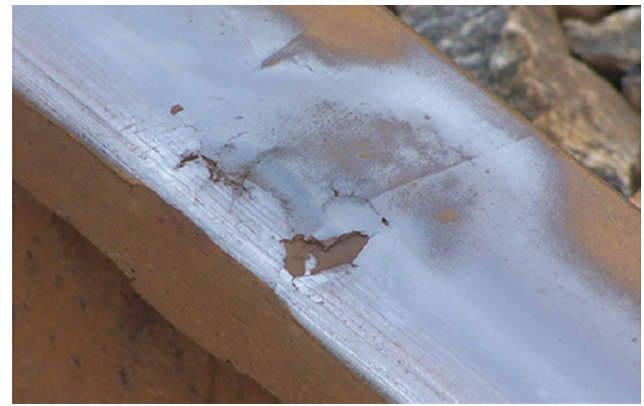
Fig. 4. One single squat at a thermite weld with shorter WM (from [15]).
