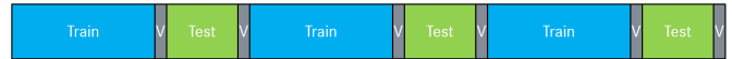
Fig. 3. The applied test, val, and train split visualized for one city. Assuming a recording length of one hour for this city, the whole session is divided into three equidistant 20 minute subsets. Each subset is then split into train, validation, and test by a 60%, 10%, 30% distribution.
