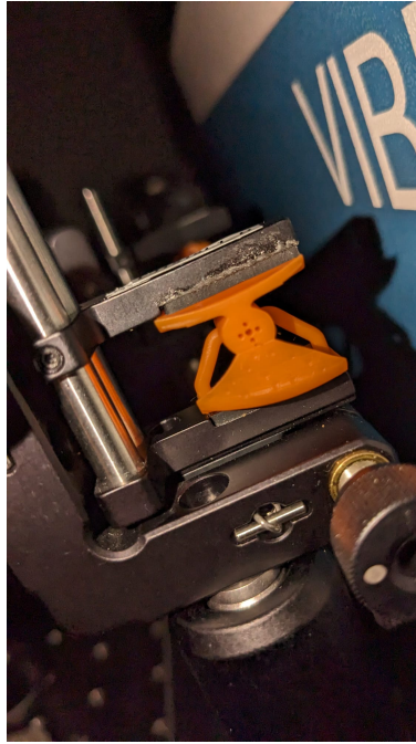
Figure 4.1: 3d printed part mimicking the catheter tip design
