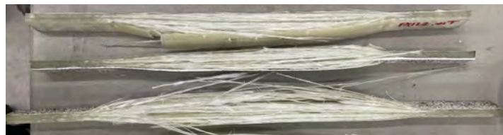
Figure 6. Delamination and fibre failure. Static material tests.
