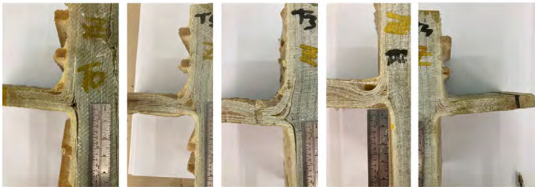
Figure 10. Failure initiation and delamination. Static component tests.
