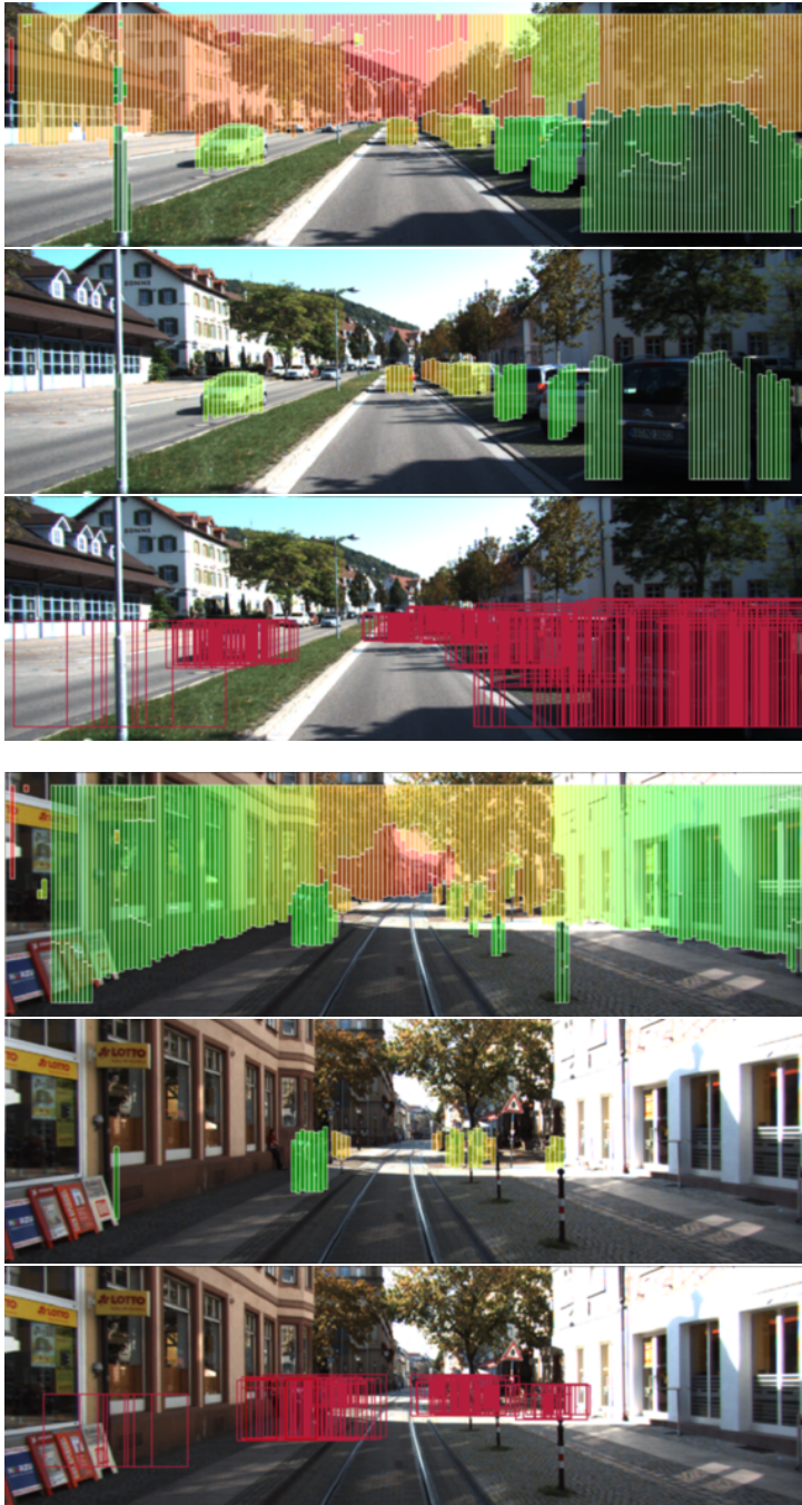
Figure 3.3: Two qualitative results of the stereo proposal generation (three rows per example). First the complete set of stixels (top) is filtered by several constraints. The resulting proposals (bottom) have the height of the remaining stixels (middle). Their width is adapted to match given aspect ratios.
