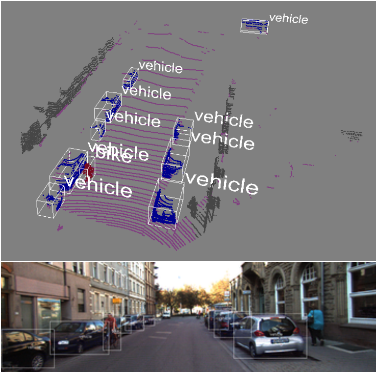
Figure 3.2: Example of lidar bounding box proposal through clustering. Top: Lidar data and 3D boxes resulting from the point clusters. Bottom: 2D proposal boxes resulting from the projection of the 3D boxes.
