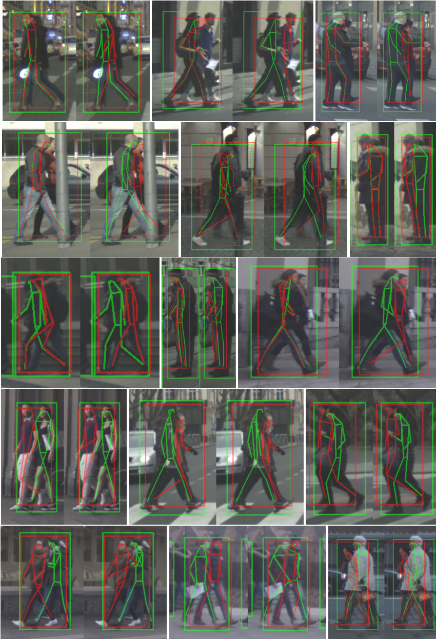
Figure 5.13: Qualitative results of AlphaPose+ (left within each pair of image crops) and the new pairwise pose estimation (right within each pair of image crops) for back pedestrians (red) and front pedestrians (green) of valid paired detections (green and red bounding boxes). The first three rows show samples where the presented method surpasses AlphaPose+, while the last two rows show error cases.
