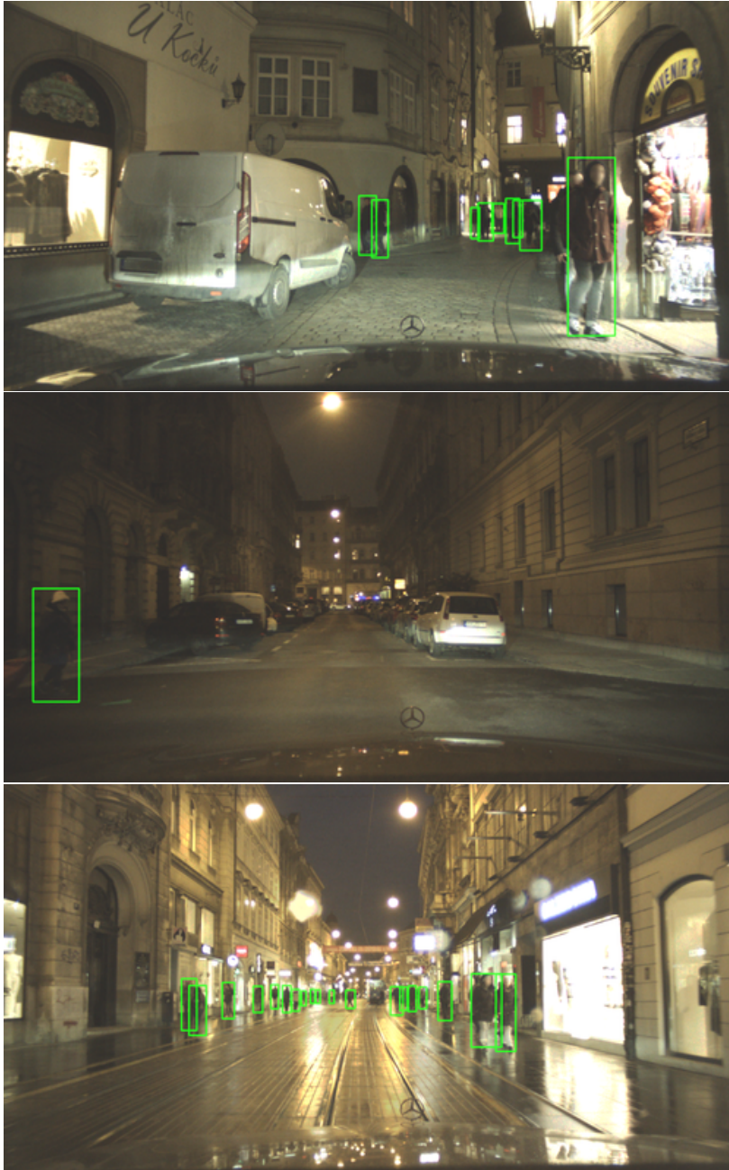
Figure 4.11: Qualitative detection results for true positives of Faster R-CNN all at fppi of 0.3 (green: pedestrians, blue: riders). Samples recorded during dusk and night.
