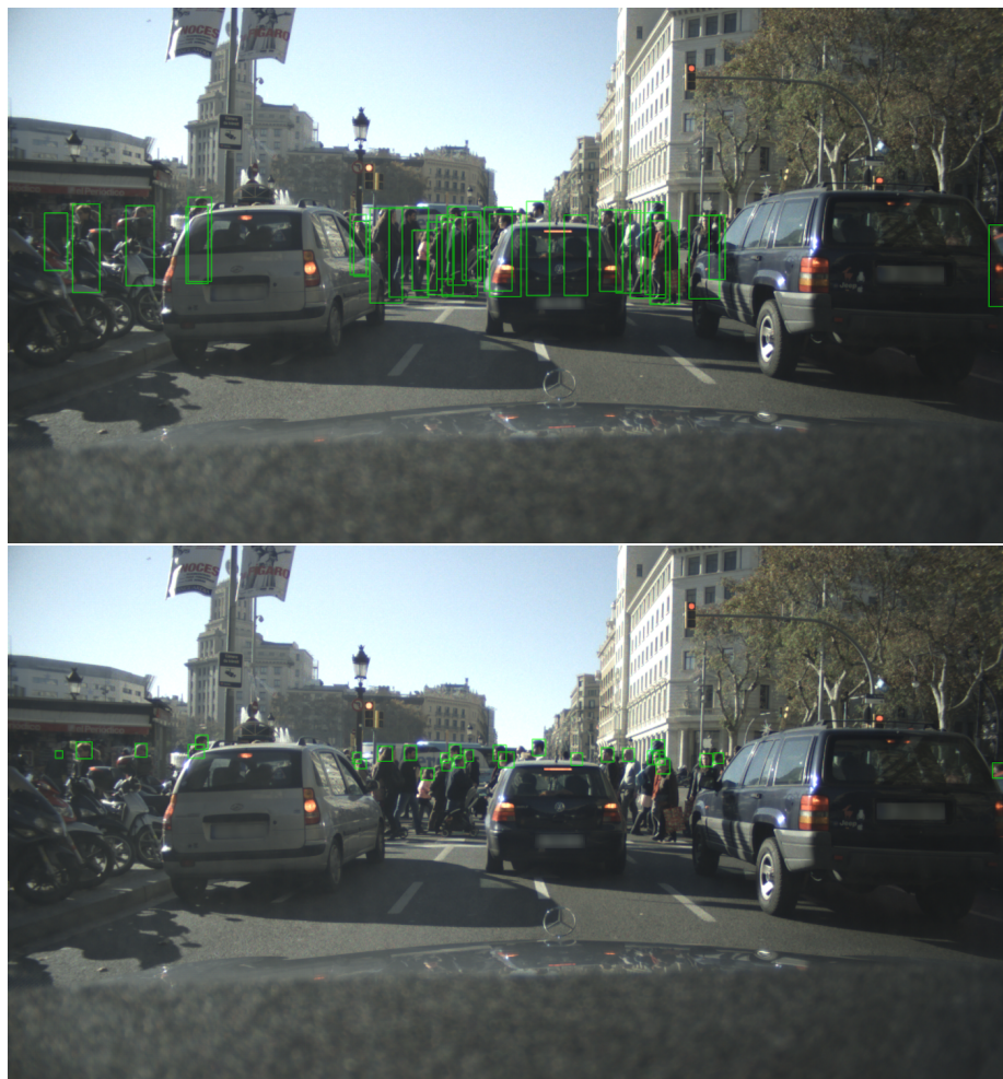
Figure 5.6: Exemplary visualization of the ground truth body (top) and head box annotations (bottom). In most cases, the level of occlusion of head boxes is lower than for the full body boxes. Reproduced from [30] with author's permission.
