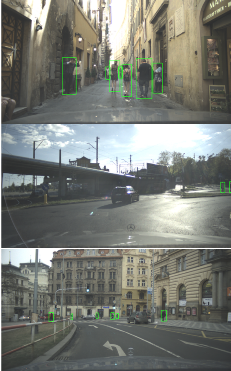
Figure 4.8: Qualitative detection results for true positives of Faster R-CNN all at fppi of 0.3 (green: pedestrians, blue: riders). Samples recorded during dry weather.
