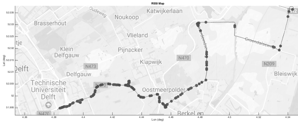
Figure 5.18: Received packets during line of sight measurement.
