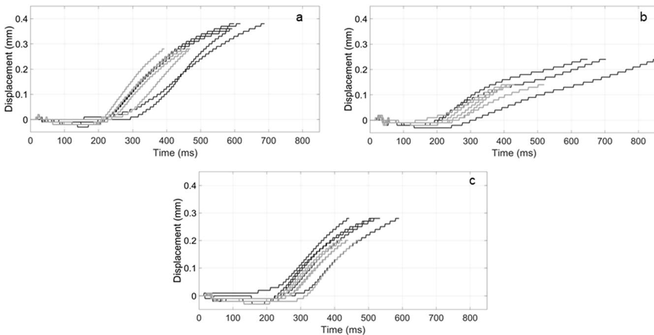
Fig. 14. Displacement of the sonotrode during the welding process in the a) epoxy-PEEK 250, b) reference PEEK-PEEK and c) epoxy-PEEK 175 configurations. Note: grey curves correspond to specimens welded up to  $d_{low}$ ; black curves correspond to specimens welded up to  $d_{high}$  (see Table 4).
