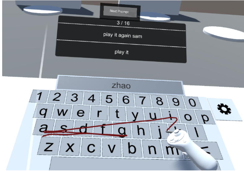
Figure 1: Picture of the word-gesture keyboard in VR being used. The user is drawing the word “again“ by drawing the gesture through the keys a-g-a-i-n.
