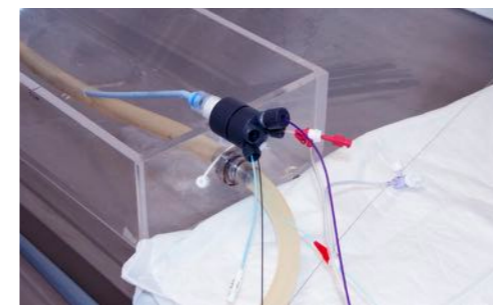
Figure 13.28 Sheath with add-on and introduced tools, placed in a flexible rubber tube
