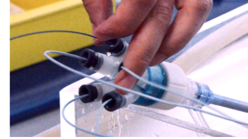
Figure 21.5 Manoeuvring of stiff wire, with visible leakage drop from valve
