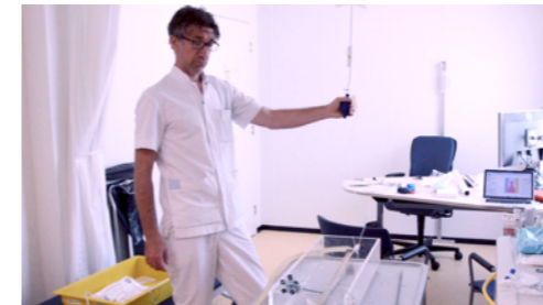
Figure 21.6 Manual pumping of pressure bag to build up 175 mmHg pressure
