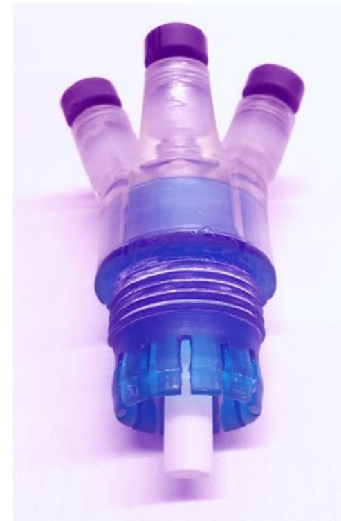
Figure 21.7 Recommended plug addition to prototype
