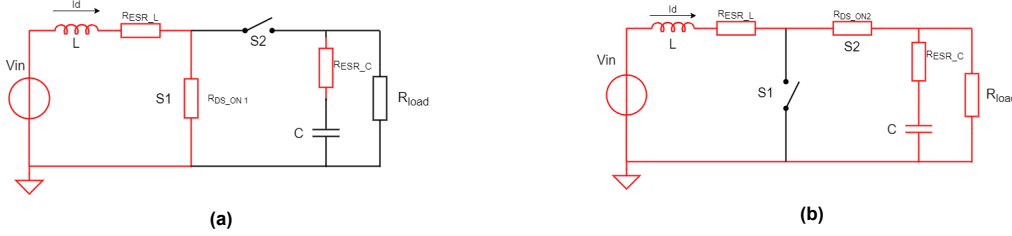
Figure 3.3: (a) Phase 1 and (b) Phase 2 of the boost converter with resistive elements causing conduction loss
